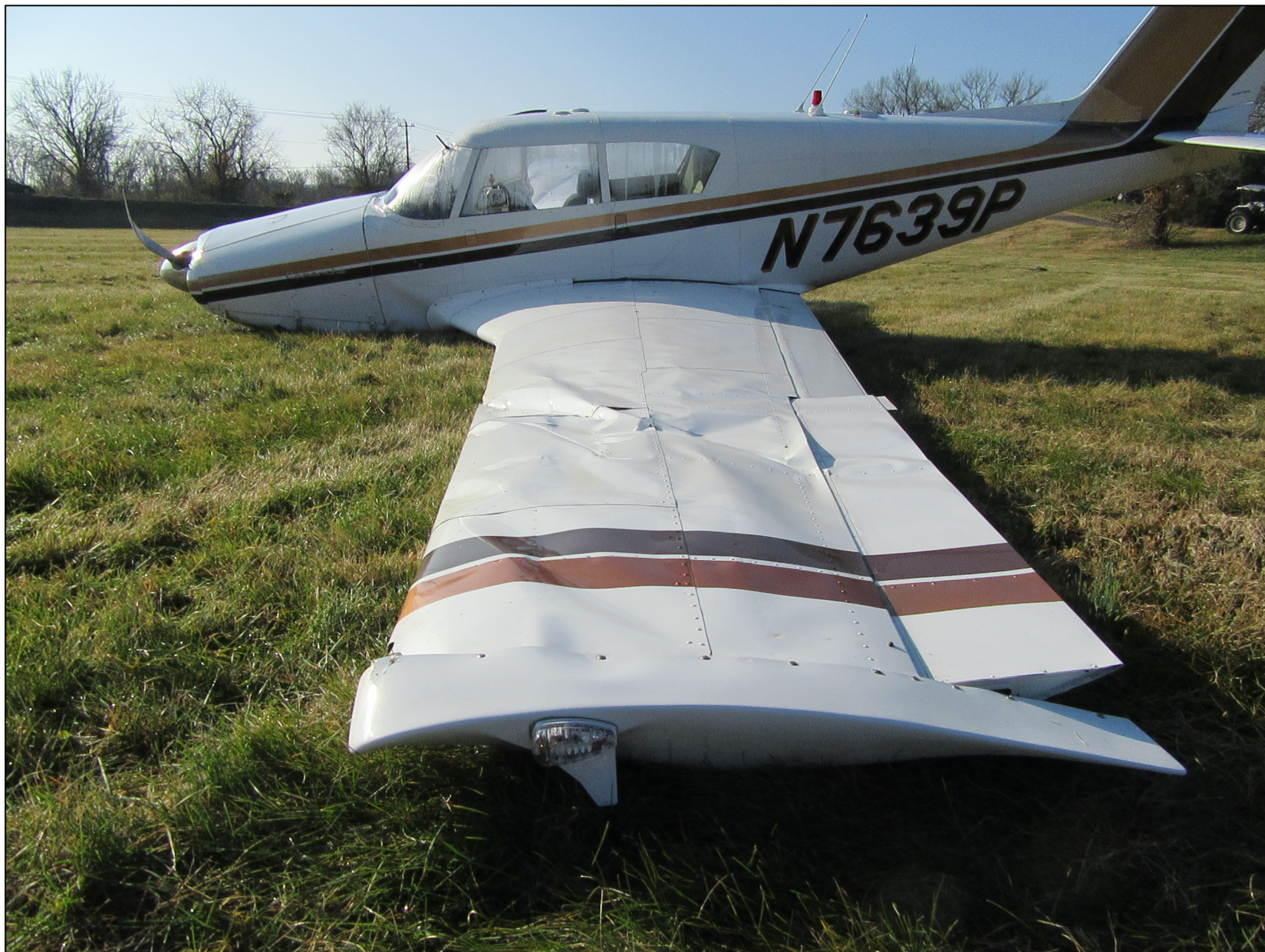
Photo 3 – Additional view of the airplane showing substantial damage to the left wing (Photo Courtesy of FAA)
