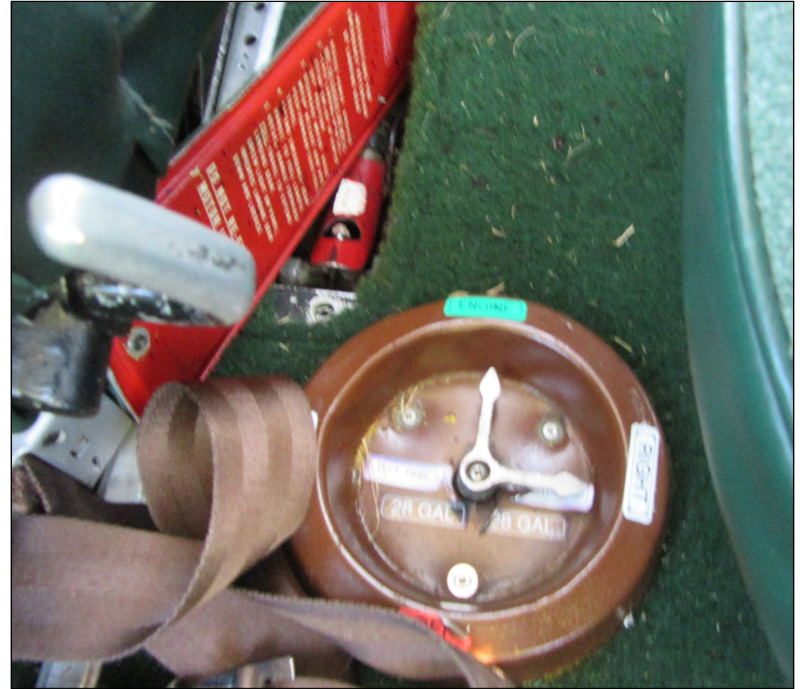
Photo 5 – View of the fuel selector selected to the right fuel tank. (Photo Courtesy of FAA)
