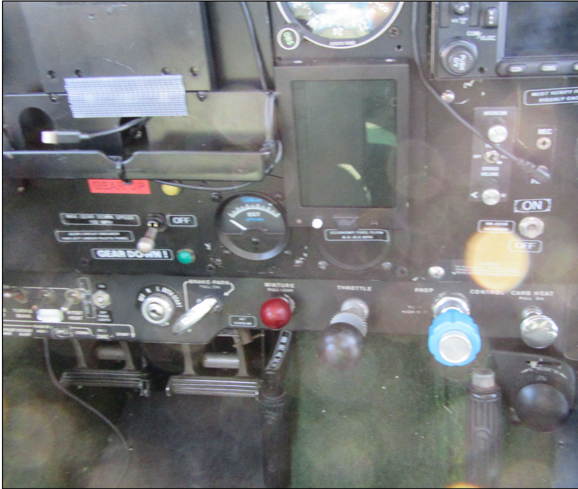
Photo 4 – View of the engine controls. The position of the carburetor heat lever was off (Photo Courtesy of FAA)
