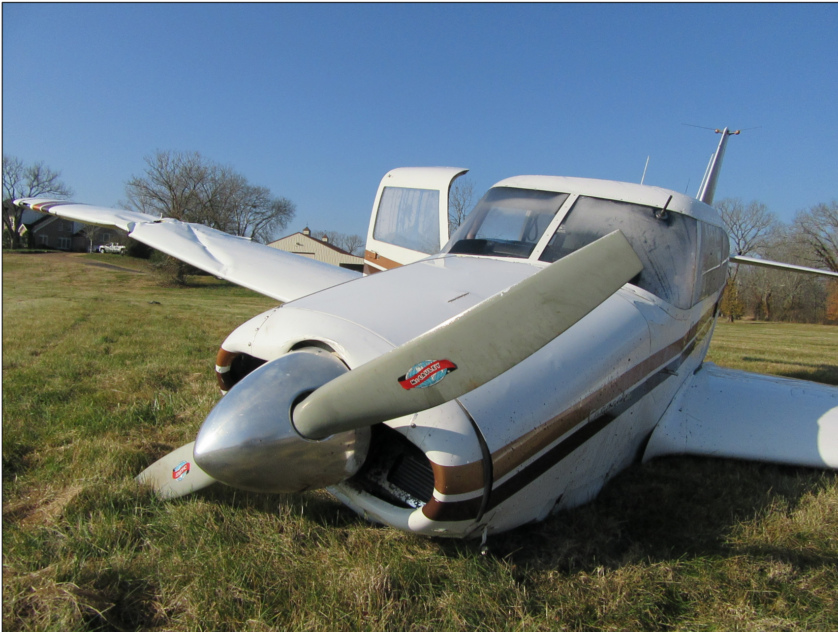
Photo 2 – Additional view of the airplane showing substantial damage to the right wing (Photo Courtesy of FAA)
