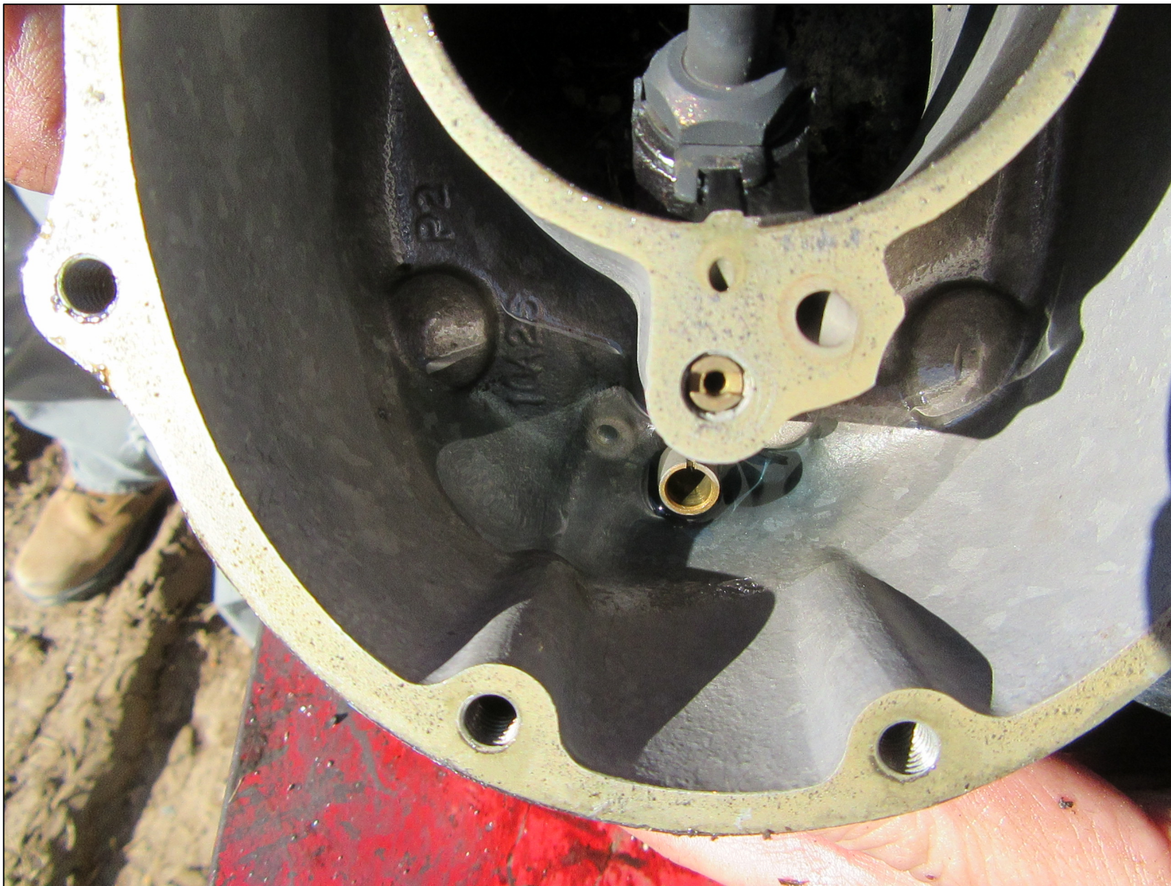
Photo 8 – View of the carburetor bowl disassembled during engine examination (Photo Courtesy of FAA)
