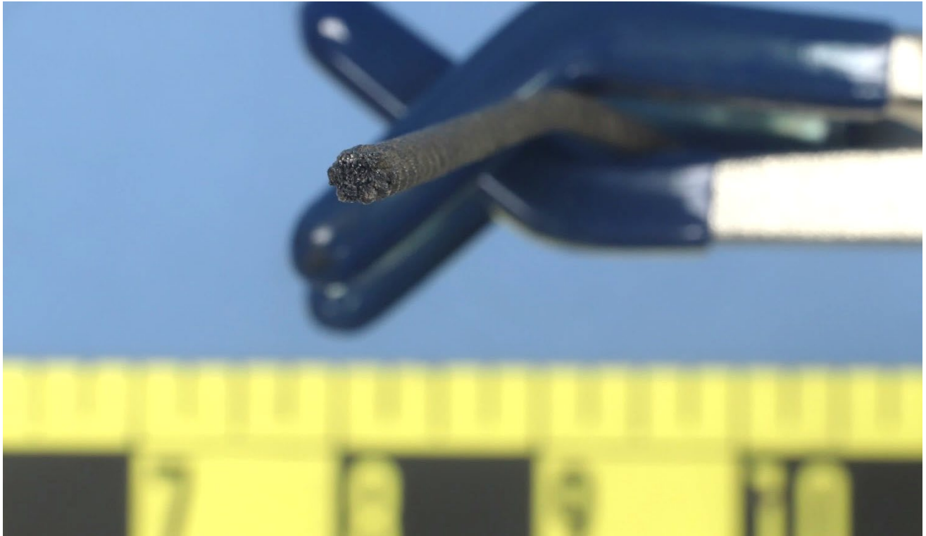
Figure 20 – View of the fracture surface of the strands from cable remnant in Figure 18.
