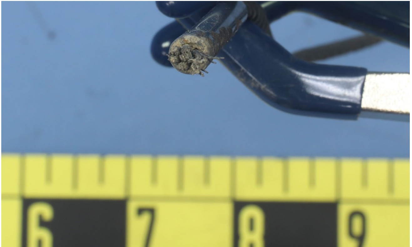
Figure 3 – View of the fracture surface of the wire strands and fork remnant in Figure 2.
