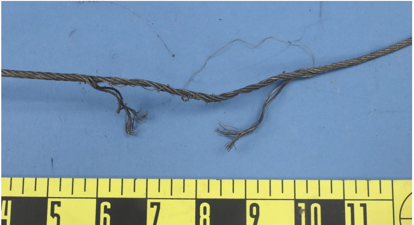
Figure 7 – View of the frayed and fractured wire strands in the bottom of Figure 1.
