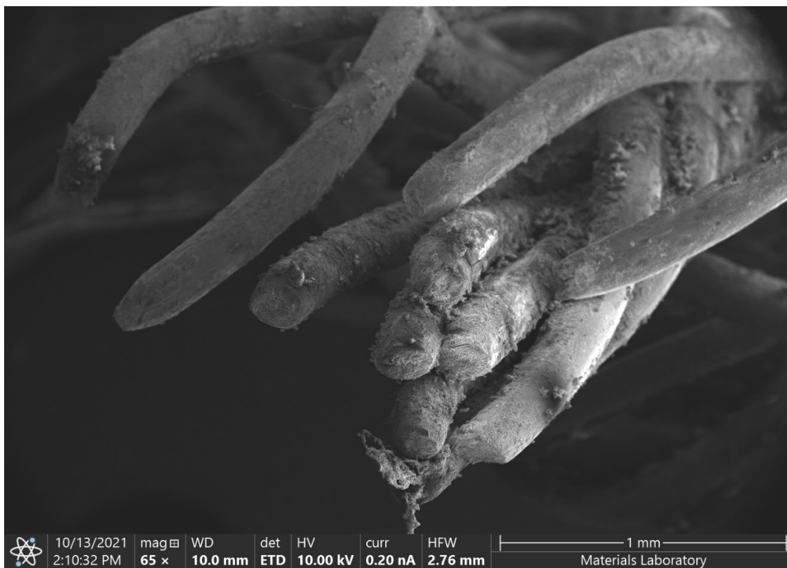
Figure 12 – SE micrograph of a set of fractured wires in the frayed area of the cable.
