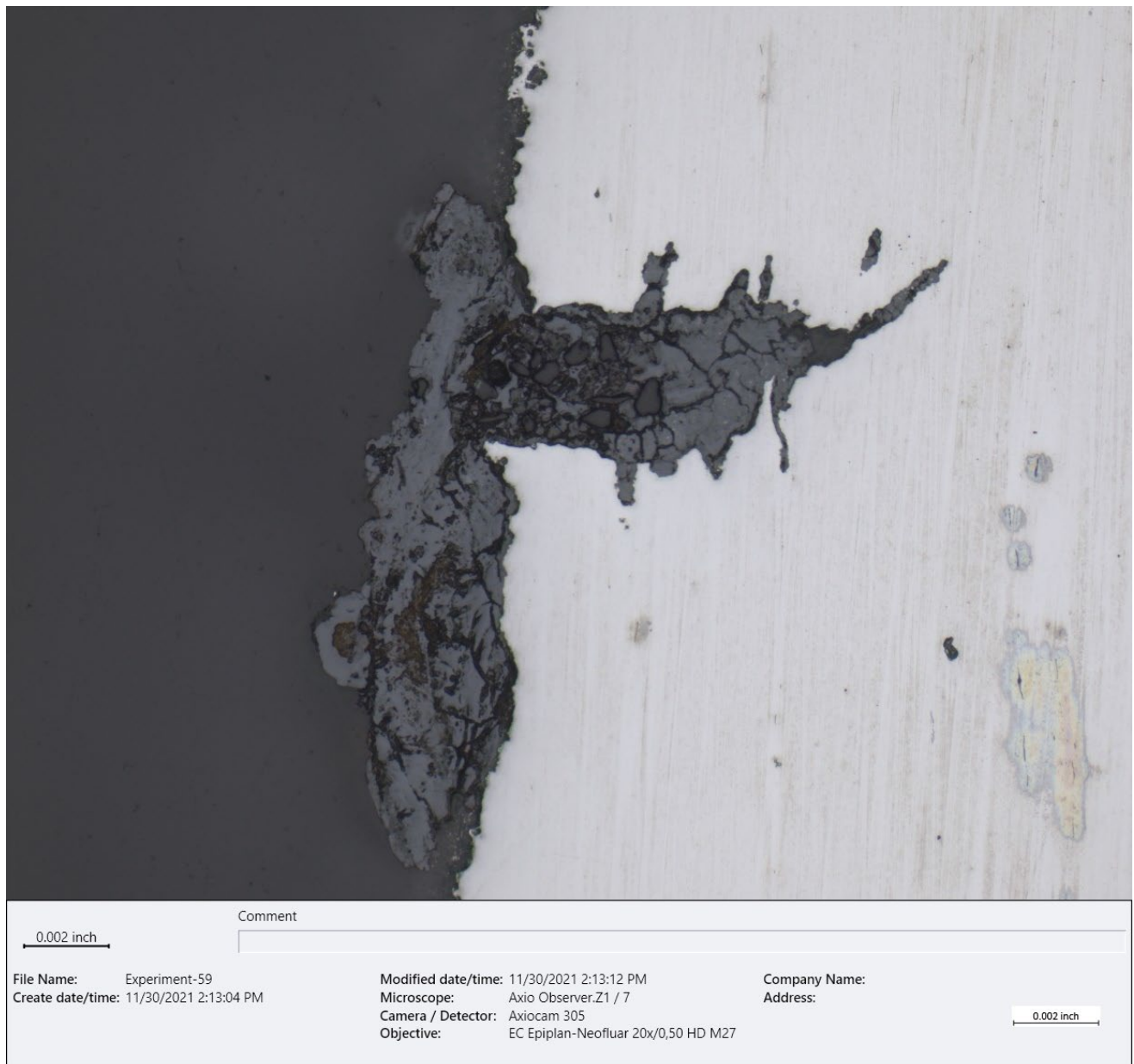
Figure 36 – BF optical micrograph of a crack from the sectioned terminal end, showing nonmetallic compounds along crack front and secondary cracks (~200X, etched from tap water).
