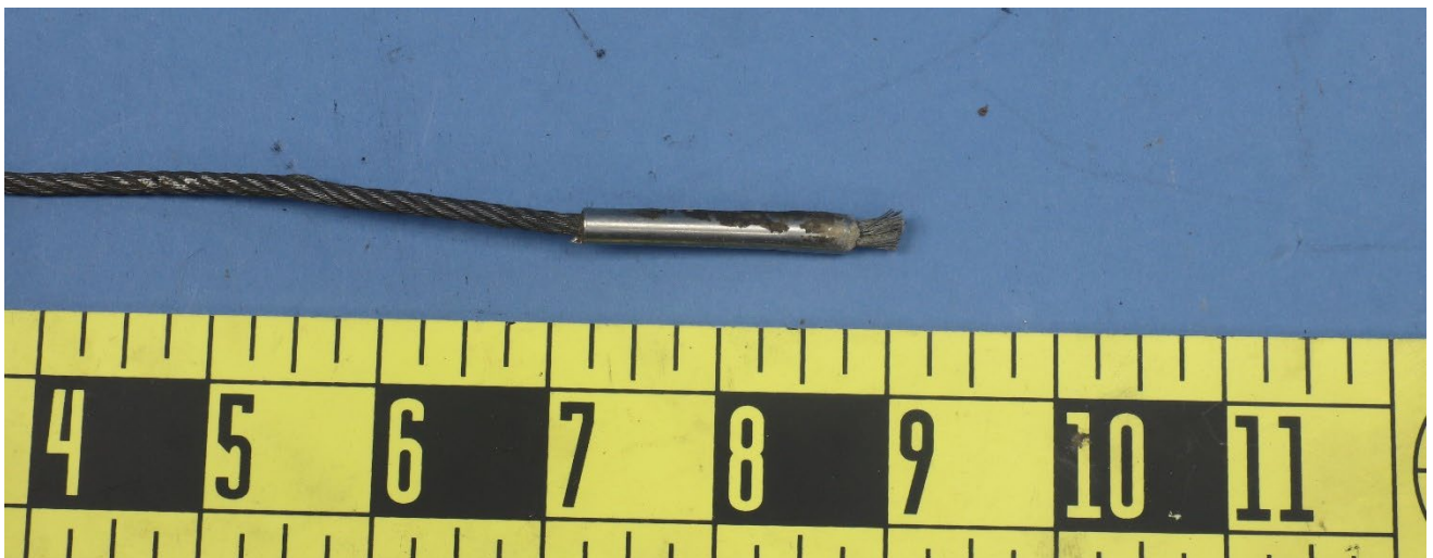
Figure 2 – View of the fractured fork with the cut wire strands, circled in Figure 1, showing the fractured end.
