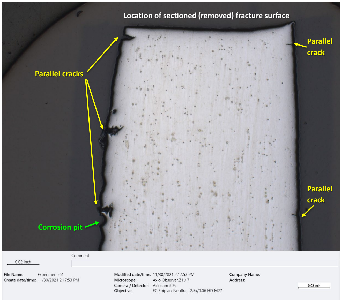
Figure 33 – Bright-field (BF) optical micrograph of a cross section of the terminal end, after sectioning of the fracture surface end (~25X, etched from tap water).
