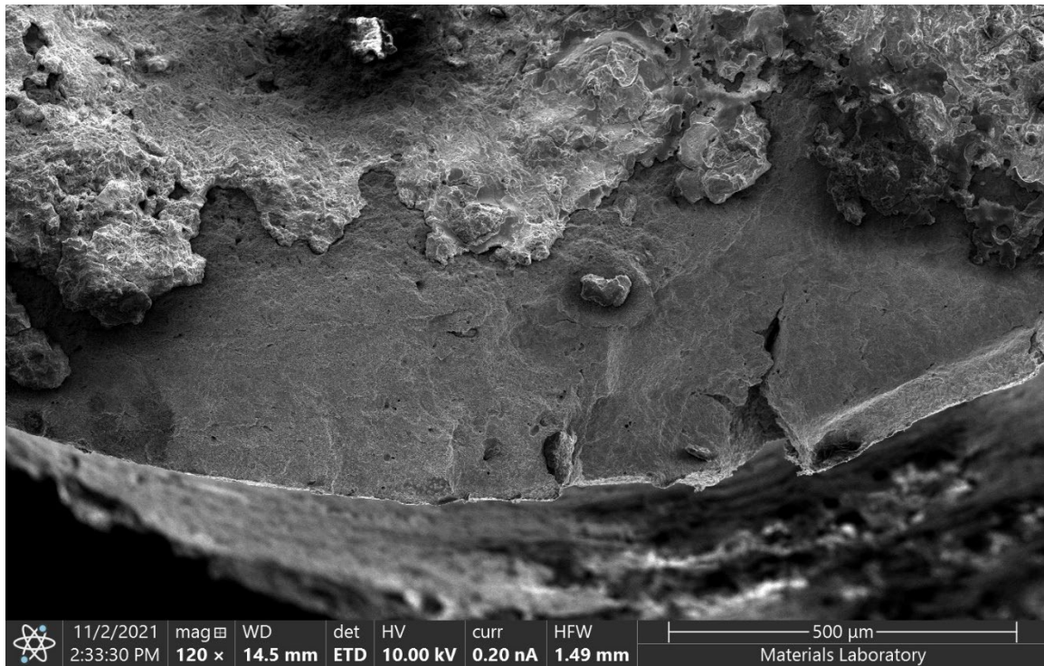
Figure 25 – SE micrograph of the edge of the end fracture surface, showing an area of ratchet marks and crack arrest marks.
