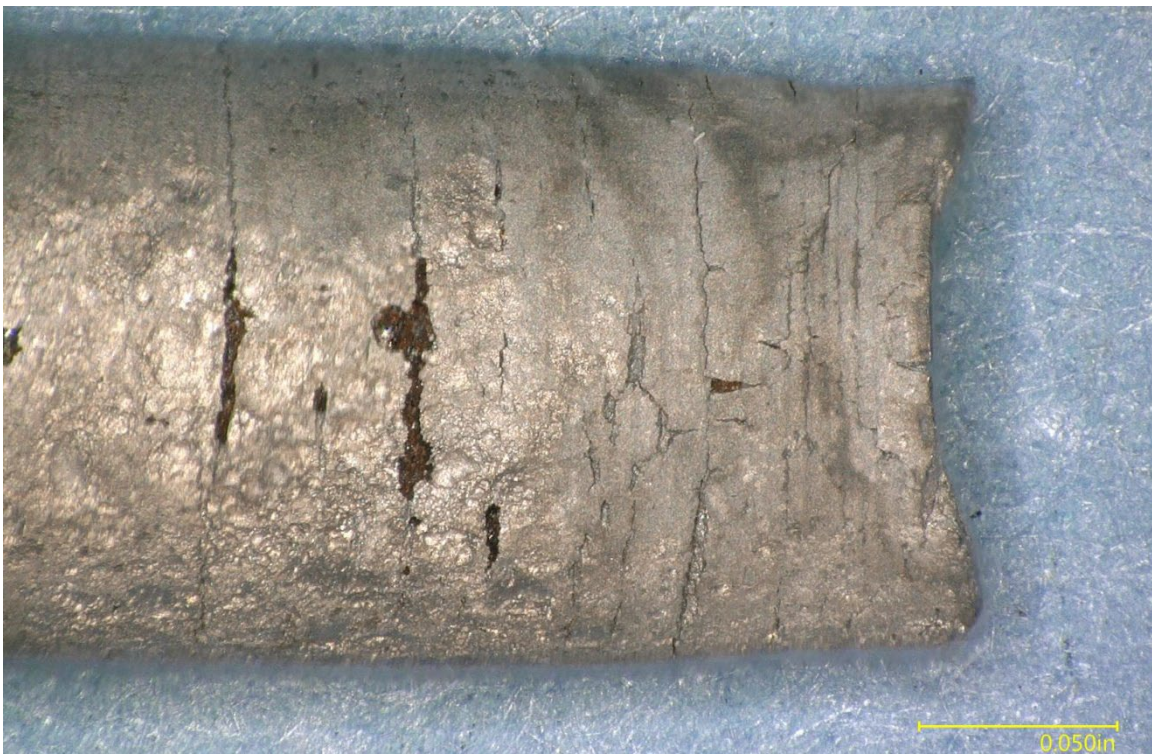
Figure 23 – The side of the end fracture, rotated 90° from Figure 22, showing a flattened area with some perpendicular secondary cracks.
