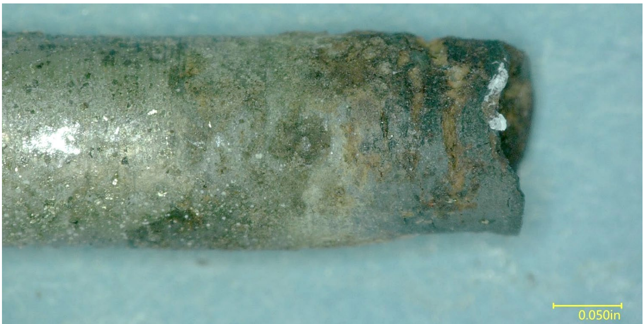
Figure 21 – View of the fractured terminal end, after disassembly, but prior to cleaning.
