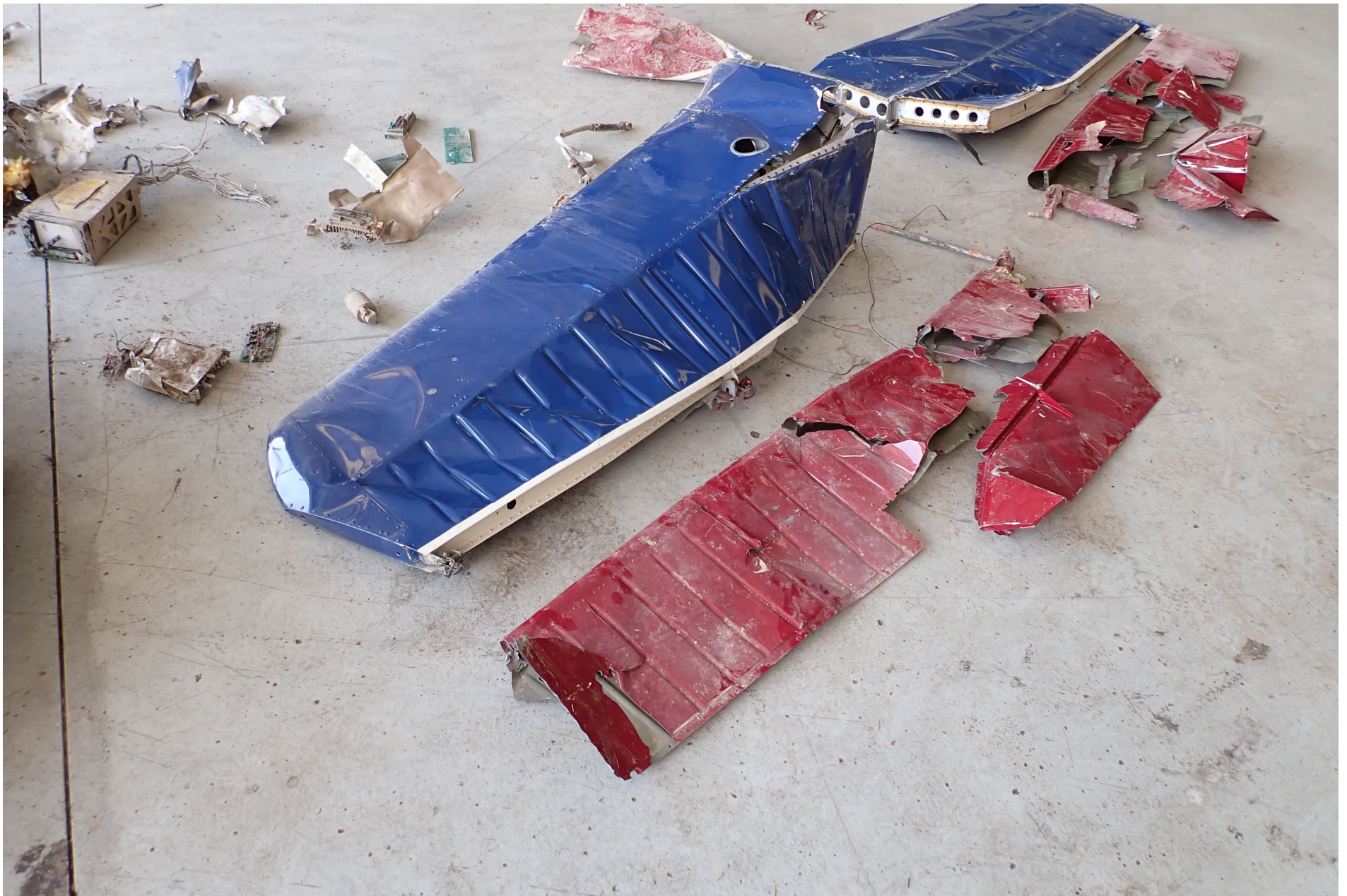
Photo 7 - Digital Photograph From Textron Aviation. View of the Reconstruction of the Both Stabilizers and Elevators.
