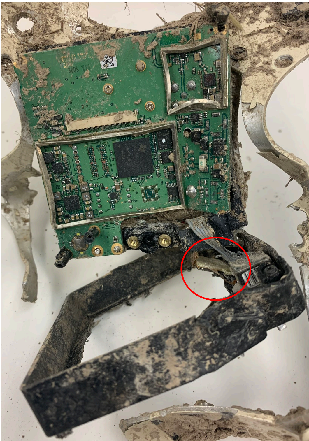
Figure 1. Photo of damaged Garmin G5 with micro Secure Digital (SD) card slot highlighted.
