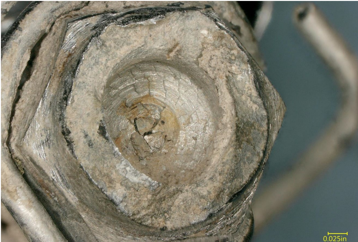
Figure 10 – View of the stud side (cockpit side) terminal stud fracture surface, post acetone cleaning.
