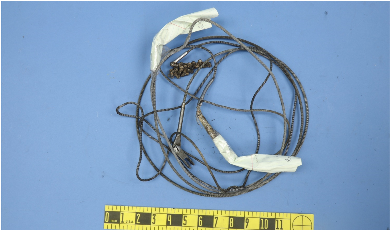
Figure 1 – View of the control wire rope remnants, as received.
