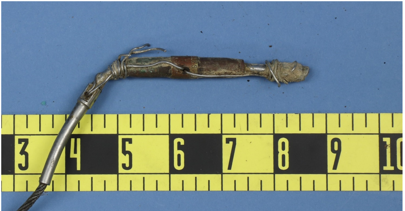
Figure 6 – View of the as-received turnbuckle fitting with a fractured portion of a terminal stud from the 'Cockpit End' wire rope remnant, viewed from the side.
