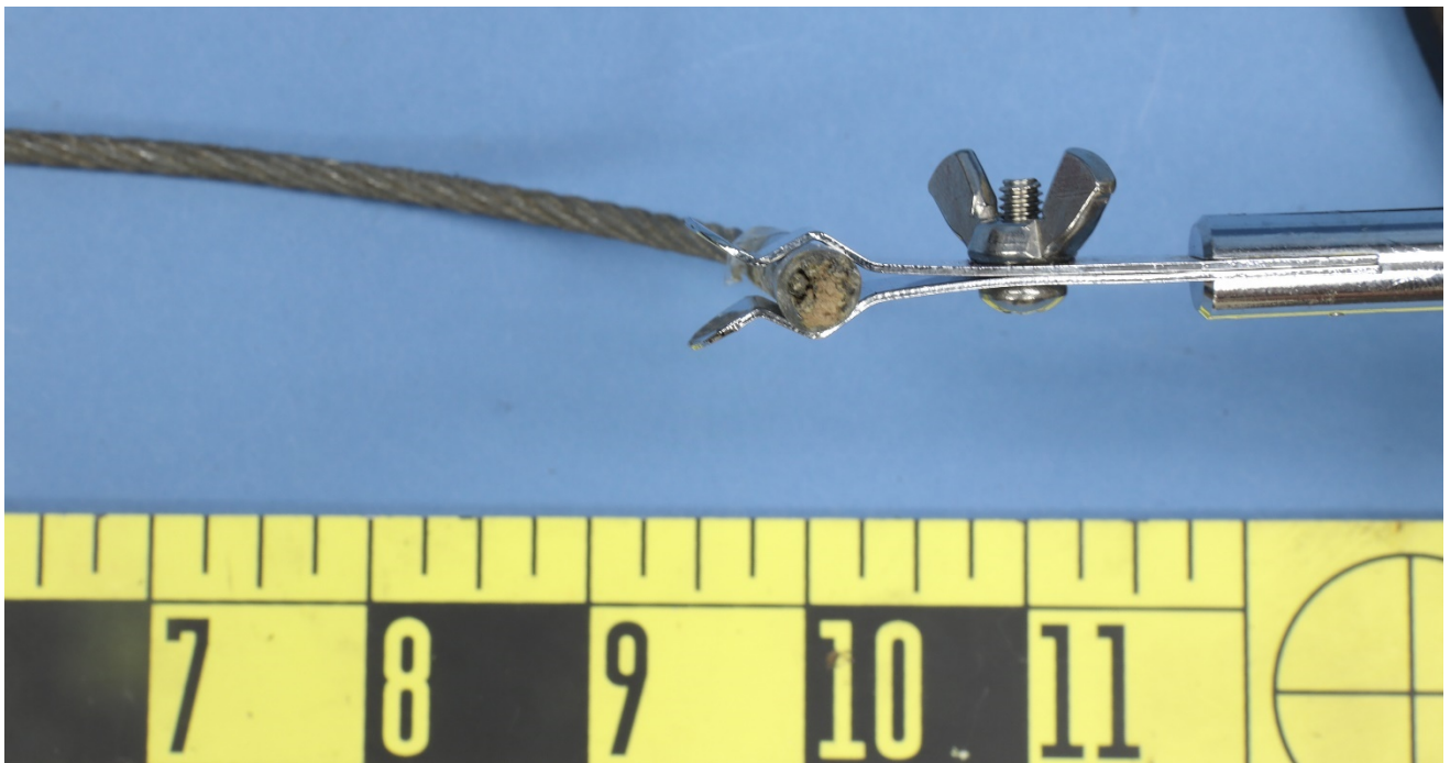
Figure 4 – View of the swaged end of the terminal stud fracture surface from Figure 3, showing caked dirt and debris in the wire strands.
