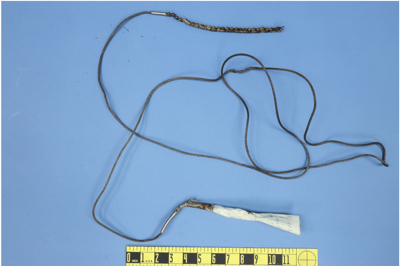
Figure 5 – View of the control wire rope remnant labeled 'Cockpit End', as received.
