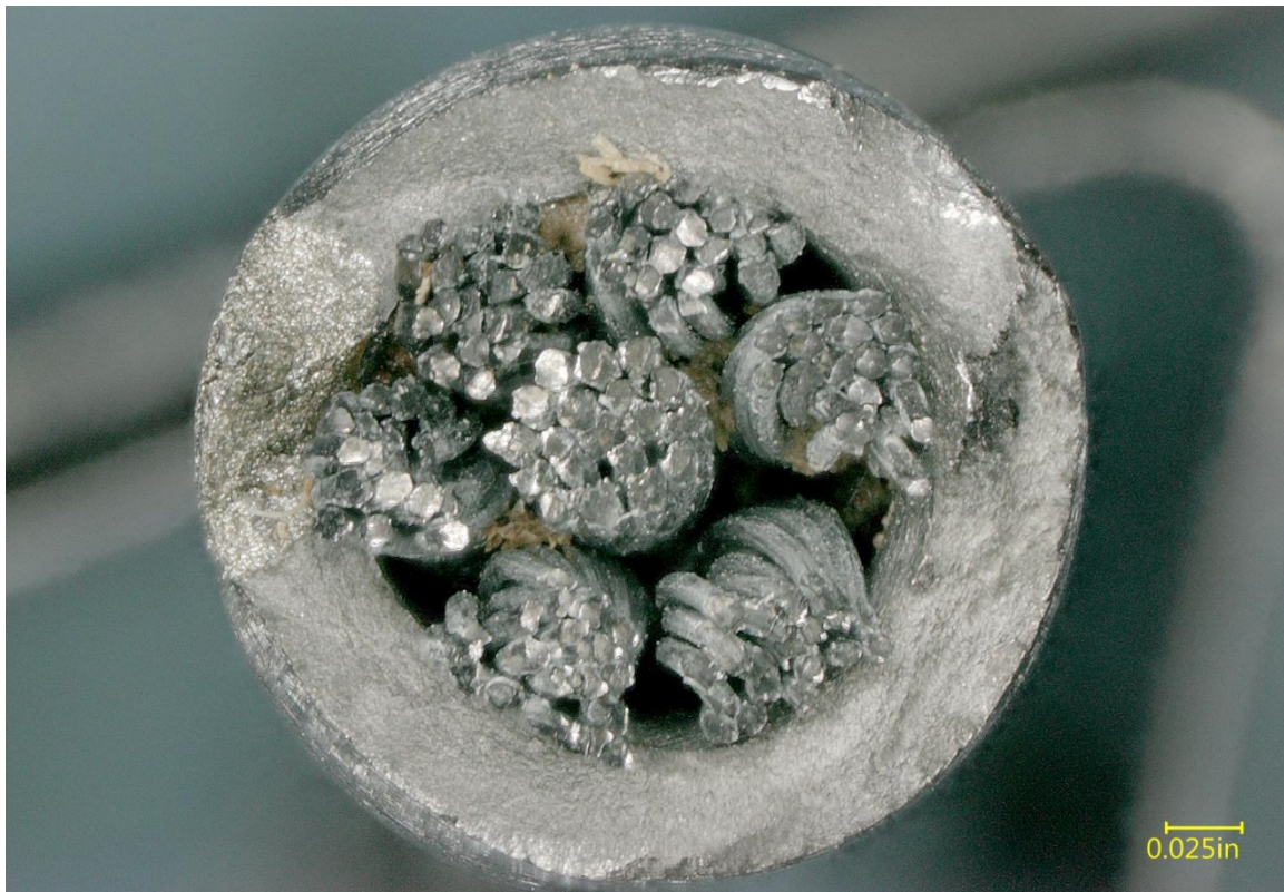
Figure 12 – View of the swaged end of the fractured terminal stud (WMS end) of the fitting, showing the wire-rope ends.
