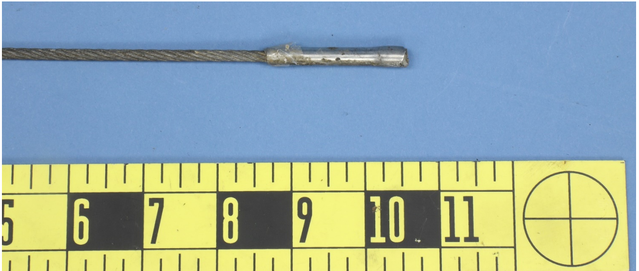
Figure 3 – View of the swaged end of the fractured terminal stud fitting end of the WMS end, viewed from the side.
