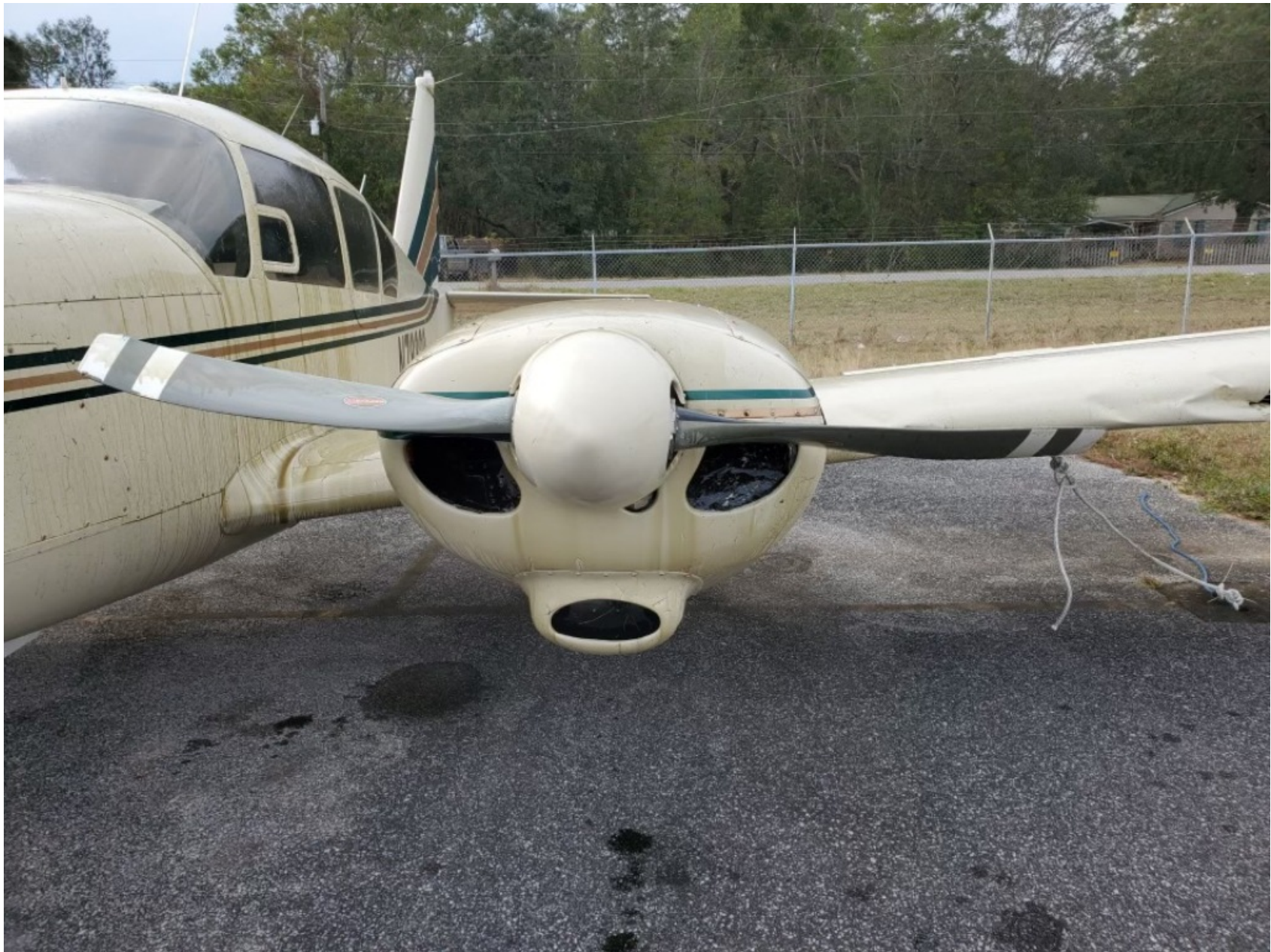
Photo 2 – Front View of LH Engine (Photo taken by FAA)
