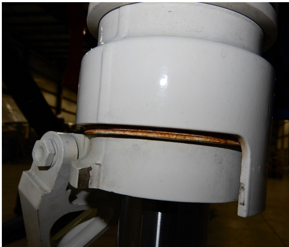
Figure 2. Left side view of impact mark on nose landing gear.
