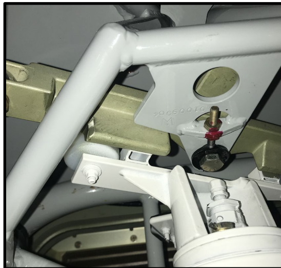
Figure 6-M600 Left turn mechanical stop between engine mount and steering arm just prior to engagement.
