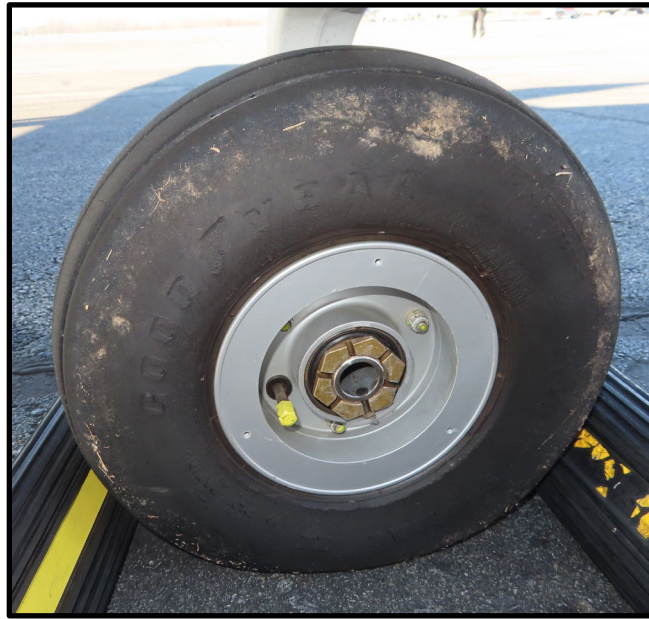
Figure 8-NLG tire with abrasion and crosswise scuffing.
