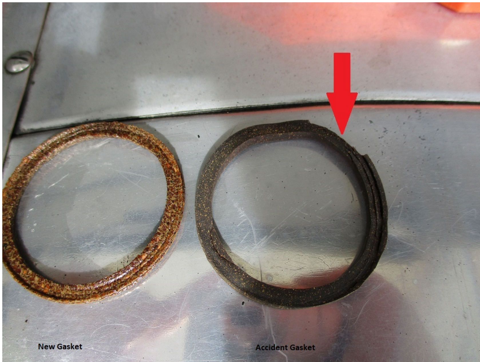
Photo 4 – Fuel Filter Screen Cover Gasket From Fuel Transfer Pump (Photo Courtesy of FAA)
