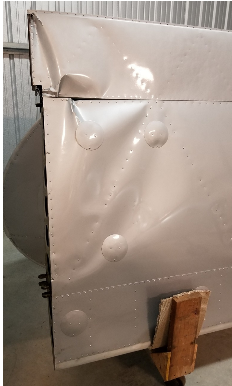
Photo 3 – Right Wing Aileron Damage (Photo Courtesy of FAA)
