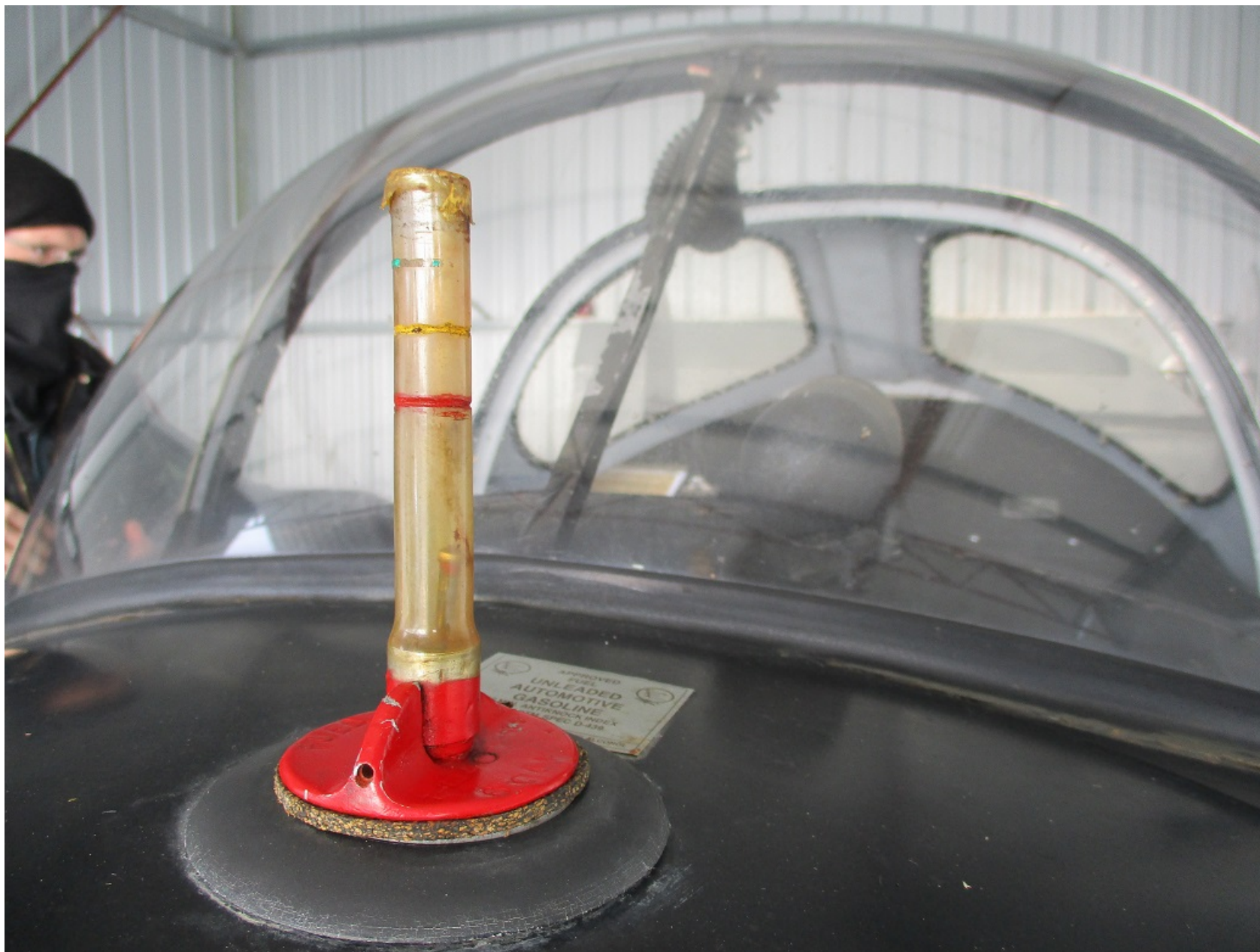
Photo 5 – Unapproved Sight Gauge For Fuel Header Tank (Photo Courtesy of FAA)
