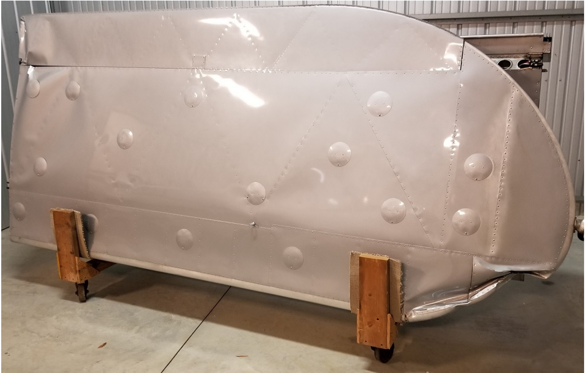
Photo 2 – Right Wing Damage (Photo Courtesy of FAA)
