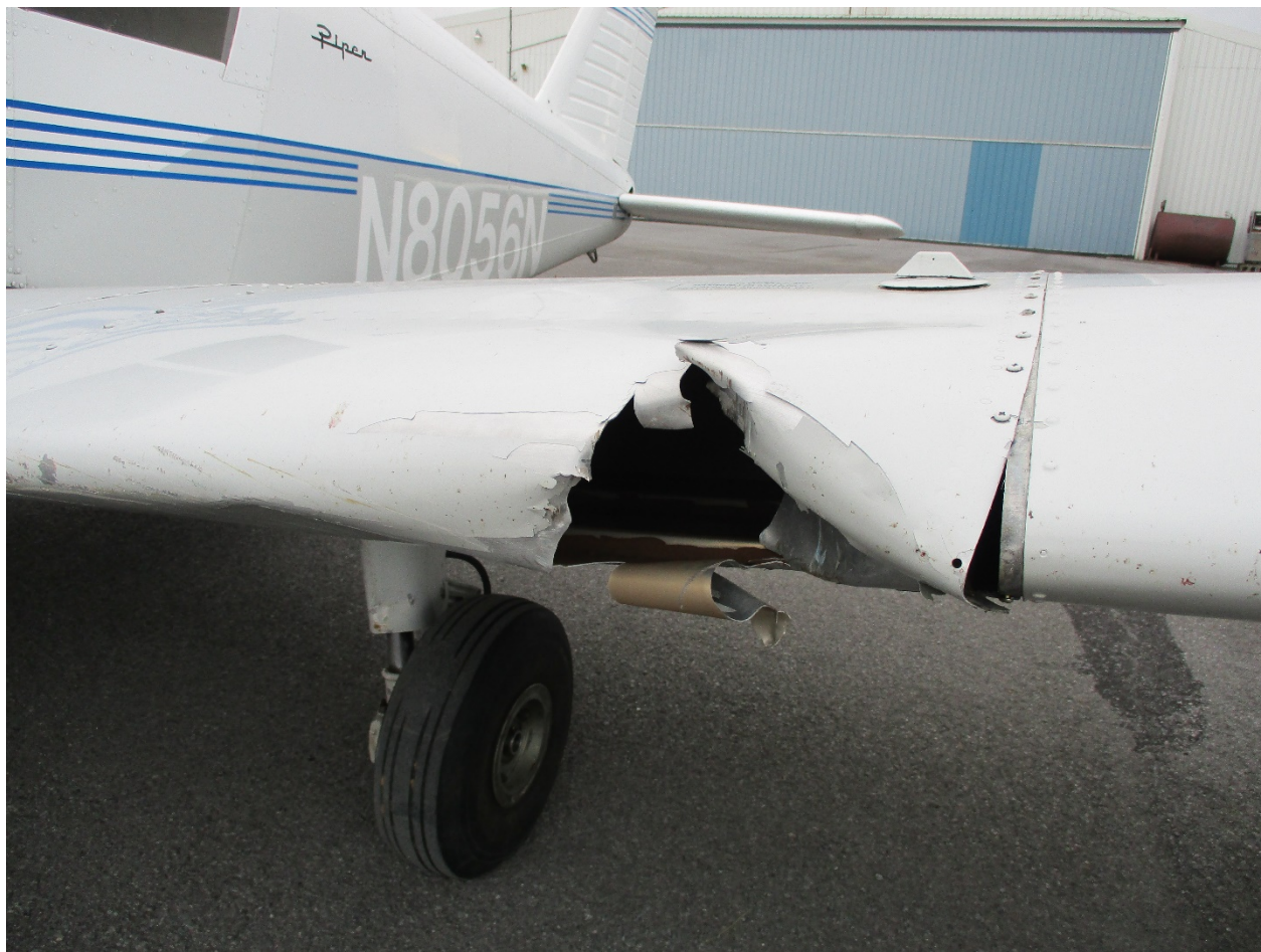
Photograph 3 3 – left wing damage.
