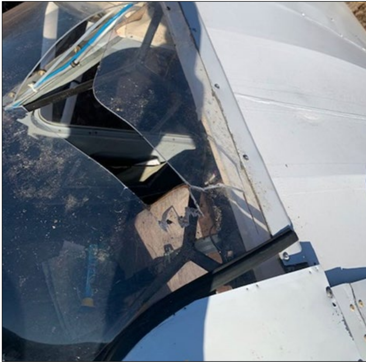
Photo 3 – View of the cracked windscreen (Photo Courtesy of FAA)
