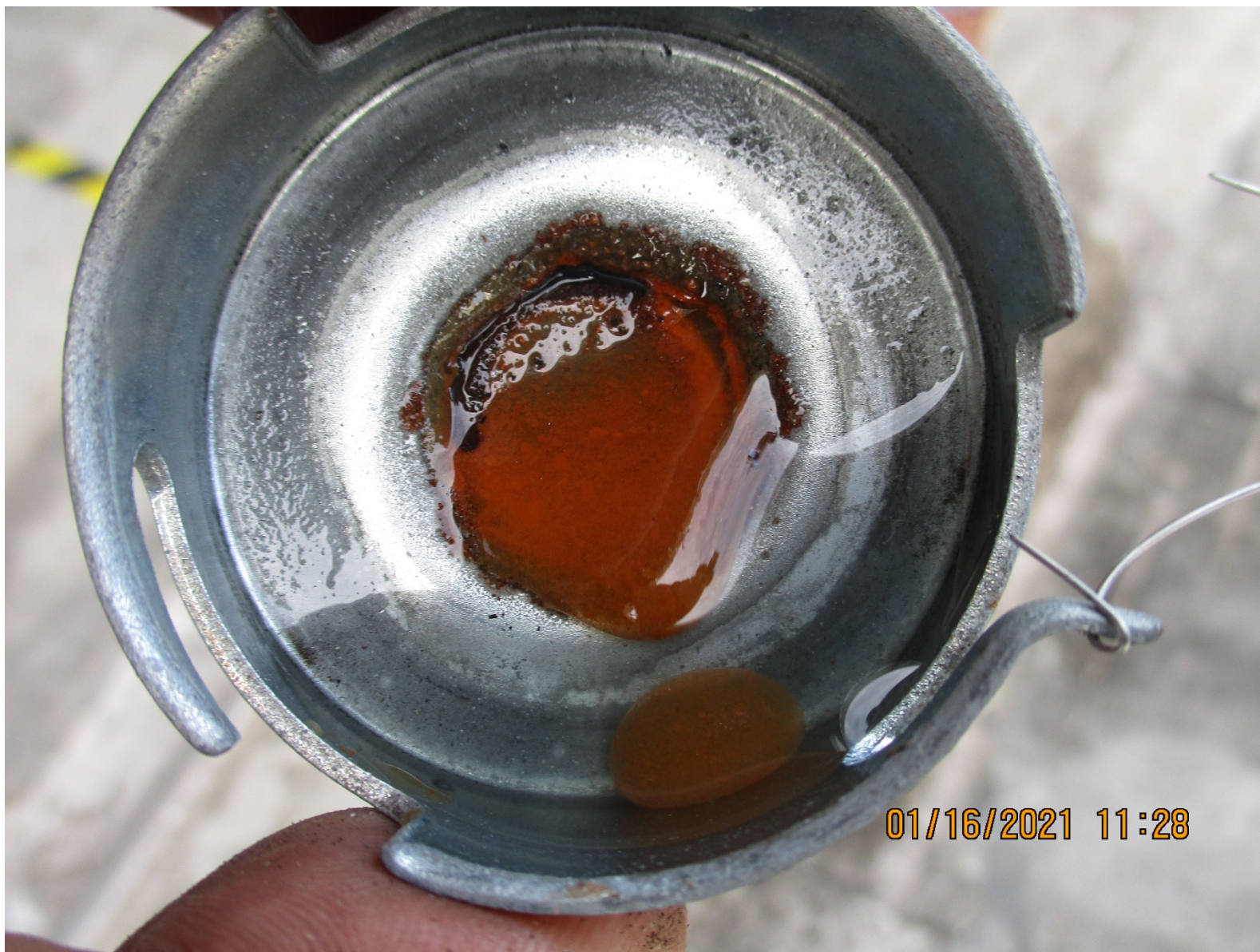
Photo 3 – View of brown liquid in fuel system. (Courtesy of FAA)
