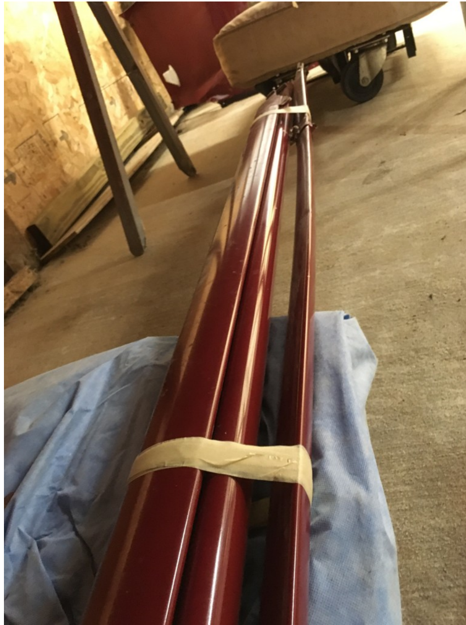
Photo 2 - Digital Photograph Provided by Ted Davis. View Depicting the Wing Lift Struts. Note the Bowing of the Strut to the Right in the Photograph.
