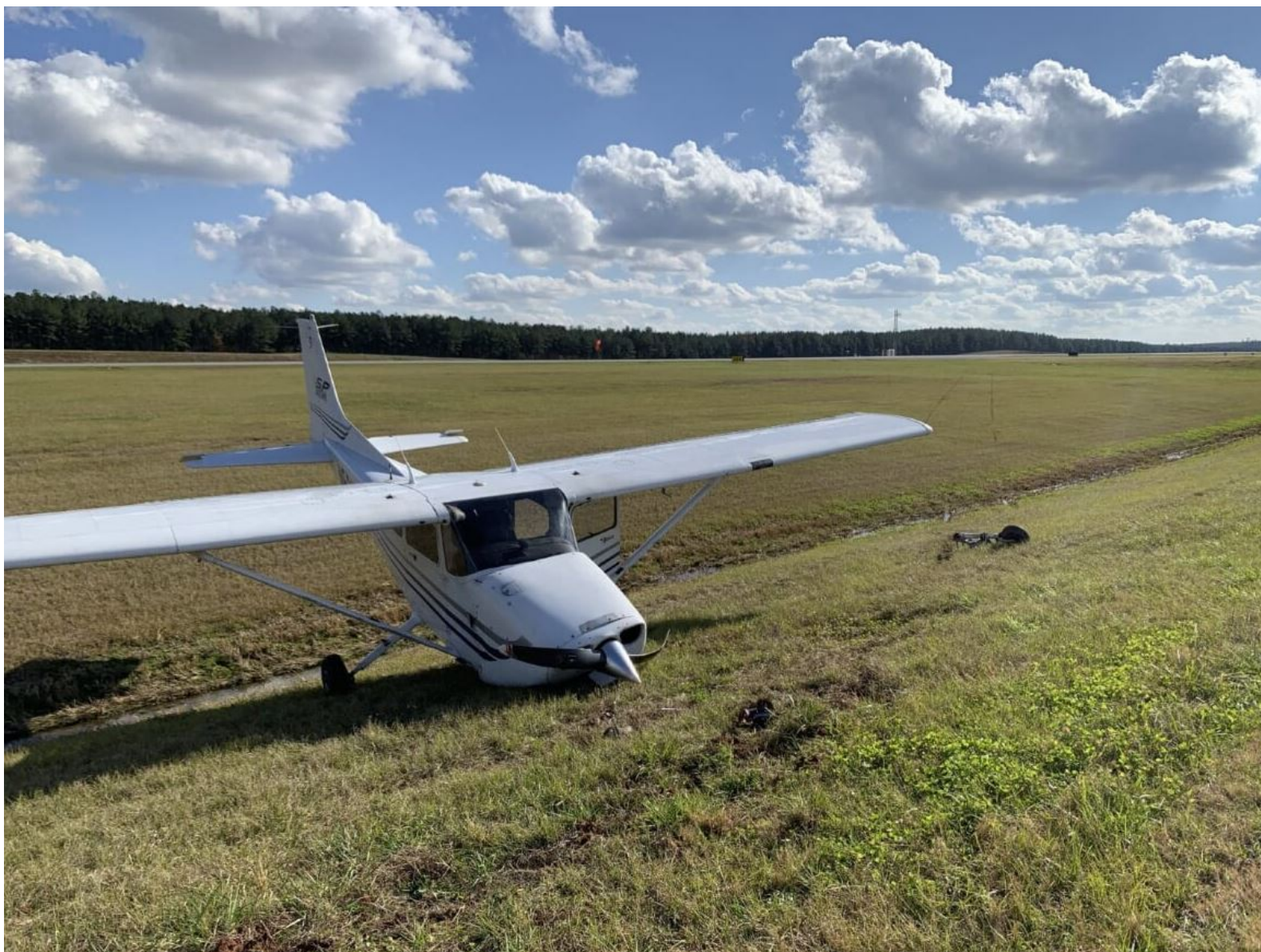
Photo 1 – Photograph of airplane damage; airplane resting on hill. Note the sheared off nose landing gear in background. (Courtesy of FAA)
