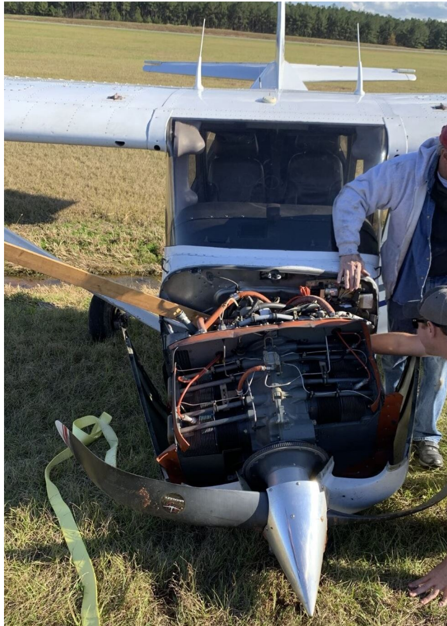
Photo 2 – Photograph of separated engine and propeller damage. (Courtesy of FAA)
