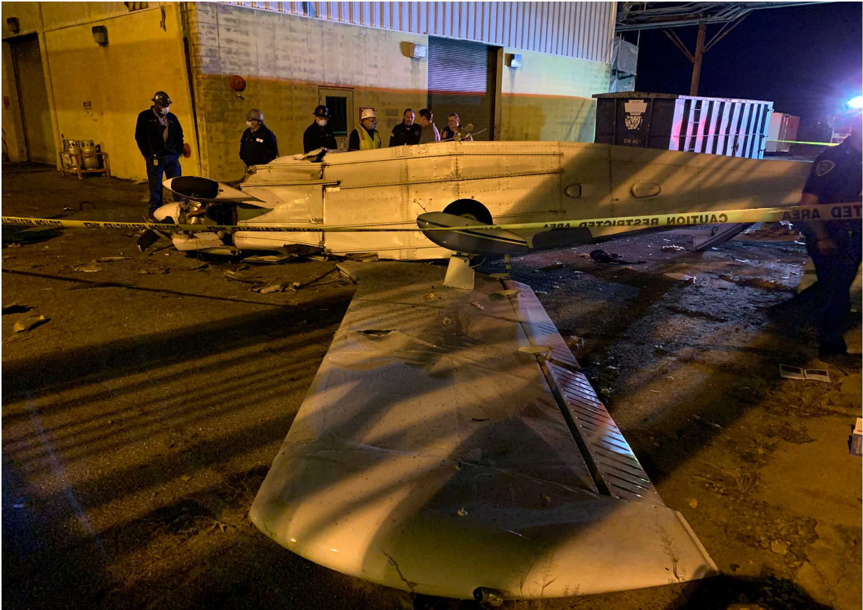
Photo 1 – FAA Photo of airplane on side of building inverted in parking area. Picture shows damage to the entire airframe.
