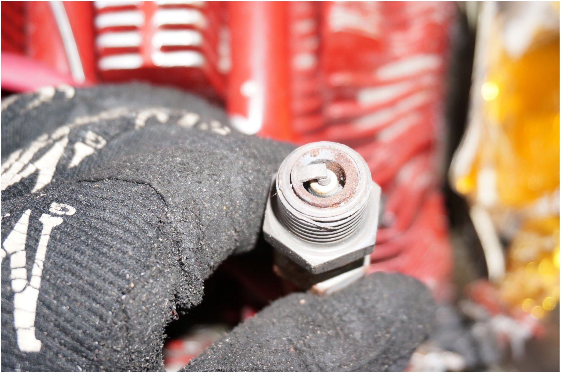
Photo 10 – Damaged Threads on Adaptor
