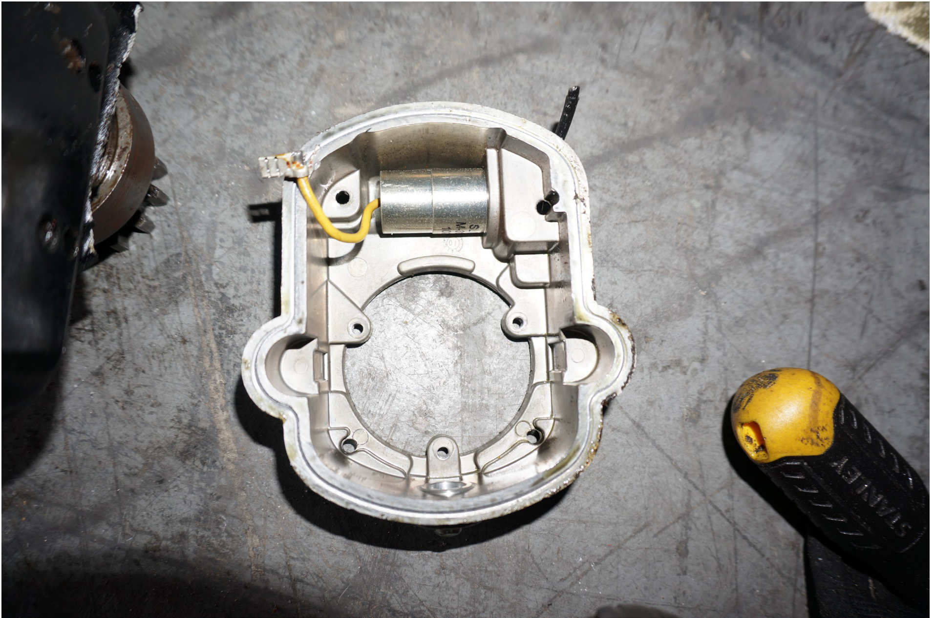
Photo 12 – Interior of Magneto Cover
