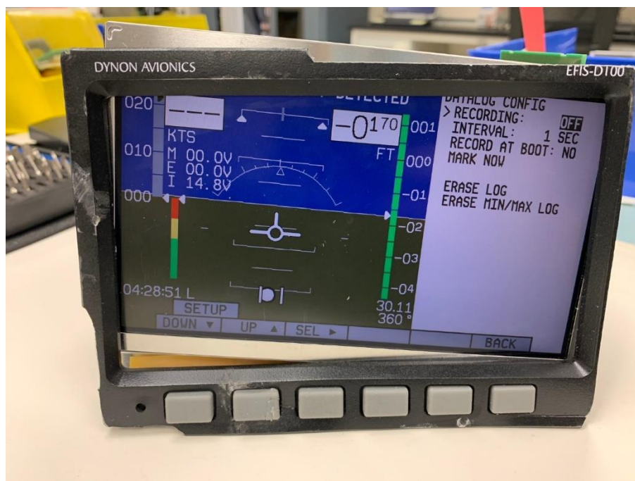
Figure 3. The Datalog Configuration page of the Dynon EFIS D-100.
