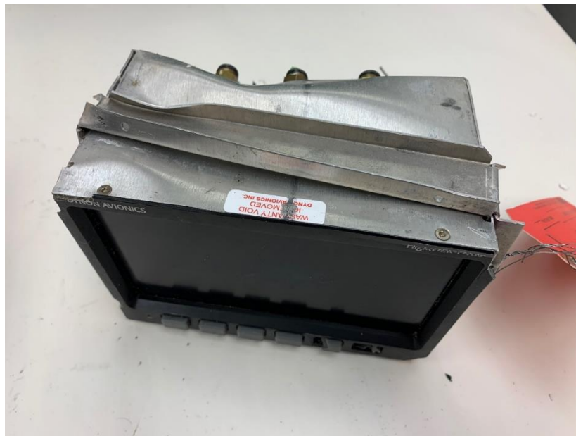
Figure 4. Damaged exterior of Dynon FlightDEK-D180.
