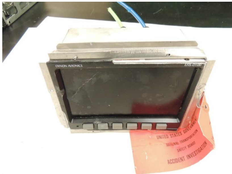
Figure 2. Damaged exterior of Dynon EFIS D-100.
