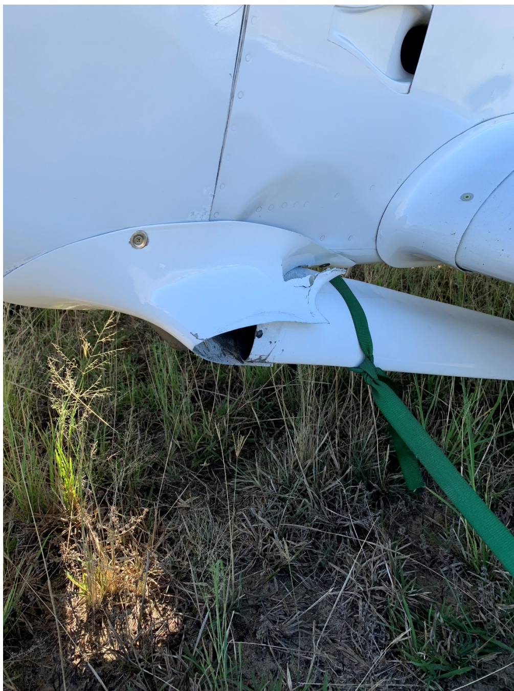
Photograph 2 2 – Left main gear strut.
