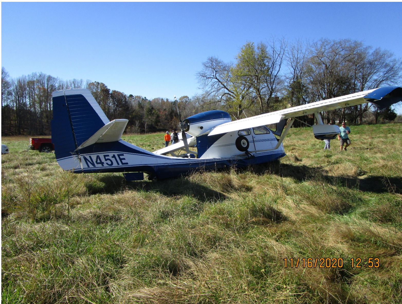
Photo 2 – View of Right Wing Strut Damage (Courtesy of FAA)
