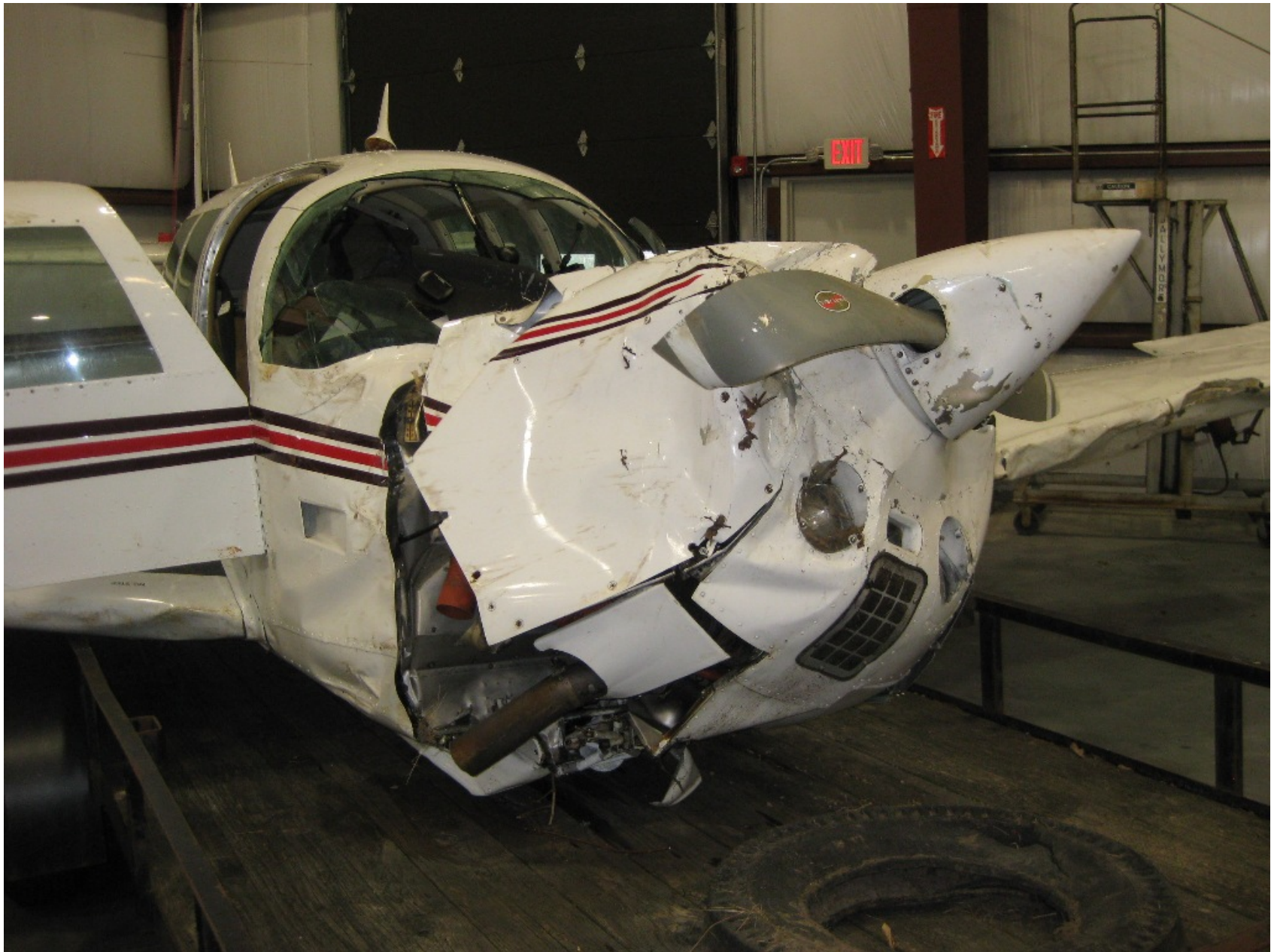
Photo 2 – View of the engine damage after the airplane was recovered (courtesy of FAA).
