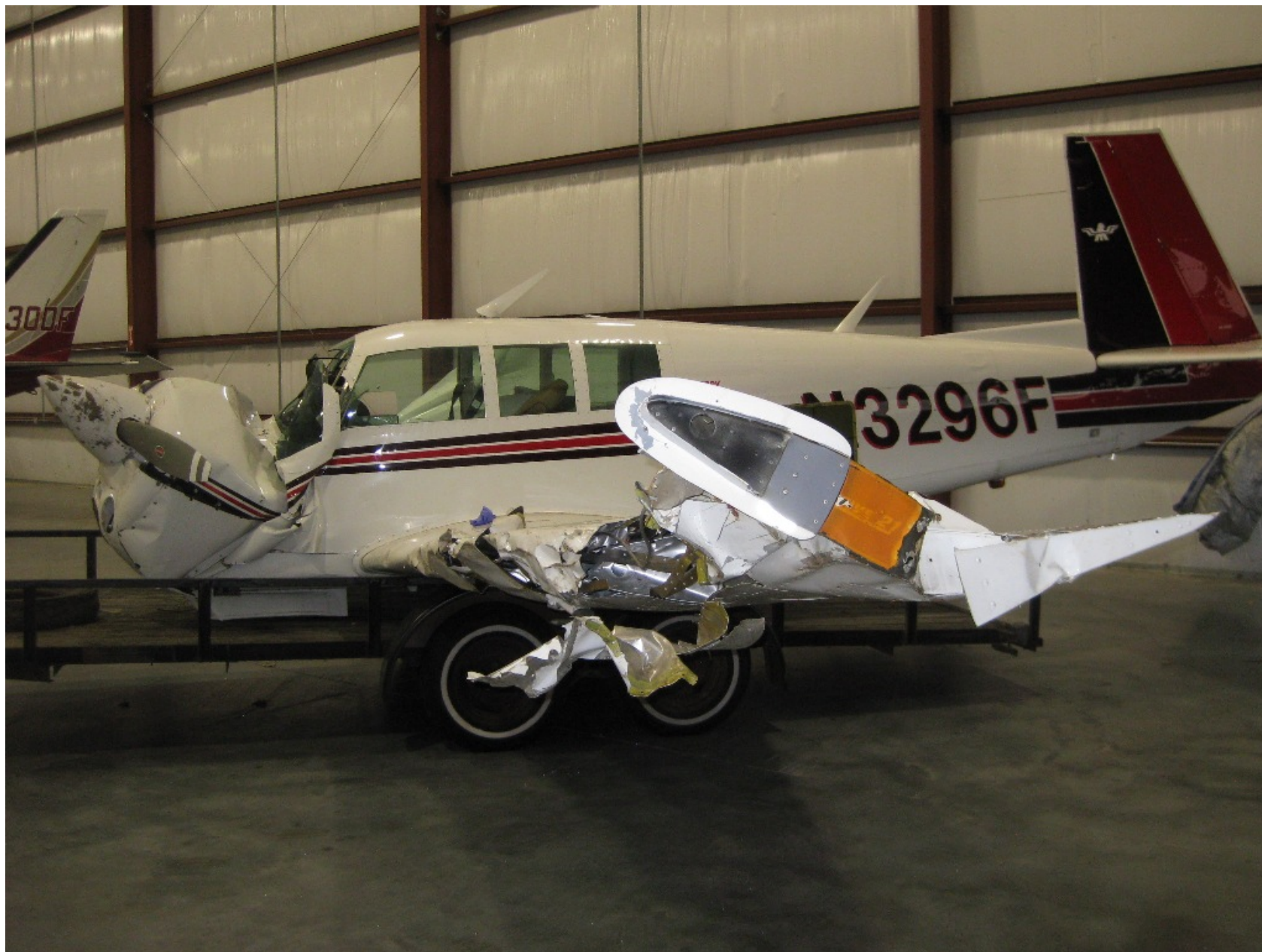
Photo 4 - View of damage to the left wing after the airplane was recovered (courtesy of the FAA).
