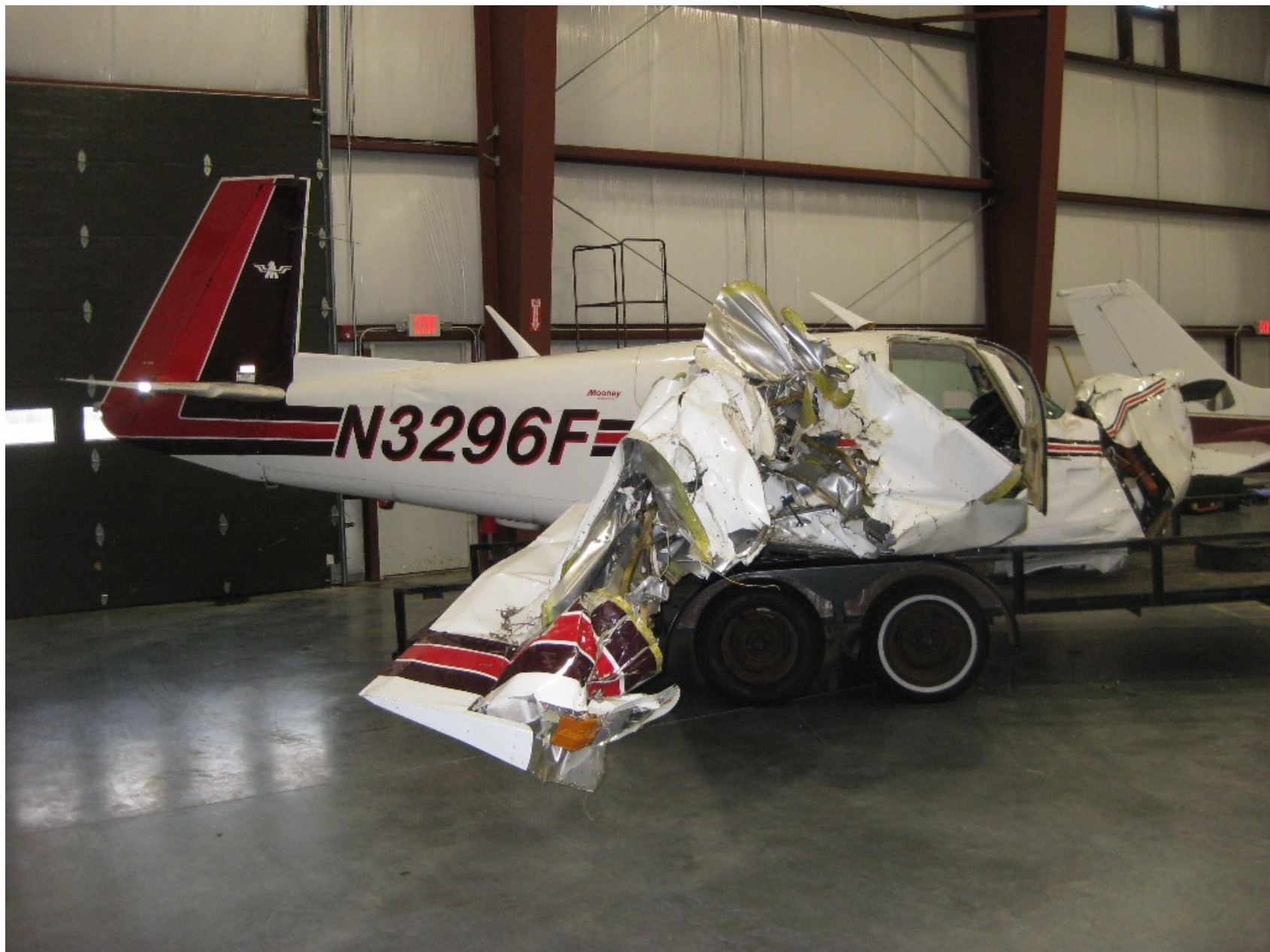
Photo 3 – View of damage to the right wing after the airplane was recovered (courtesy of the FAA).
