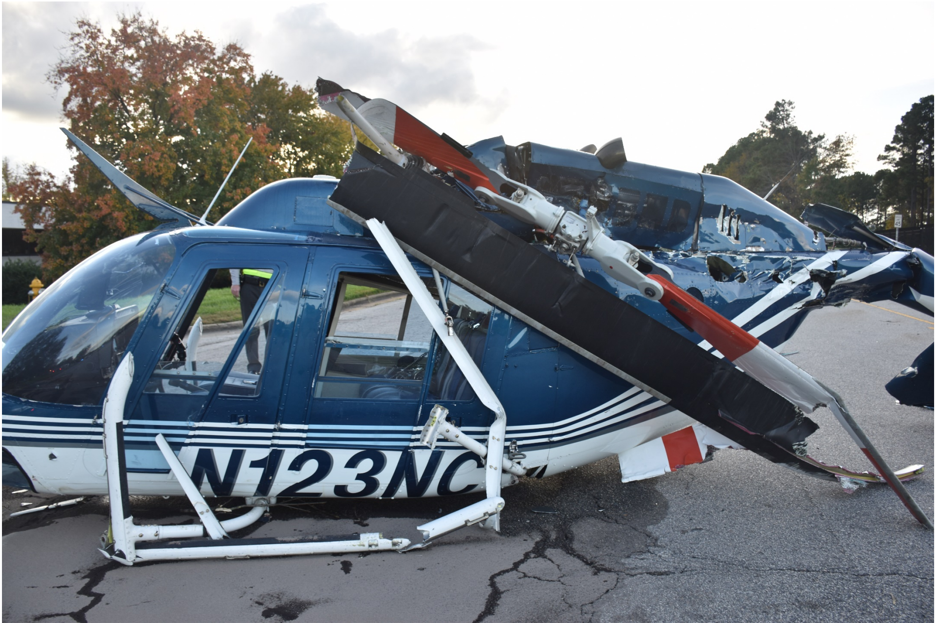
Photo 4 - Digital Photograph From NC Highway Patrol. Close-Up Left Side View of the Fuselage. Note the Damaged Main Rotor Blades and Mast, Tailboom, and Skids.
