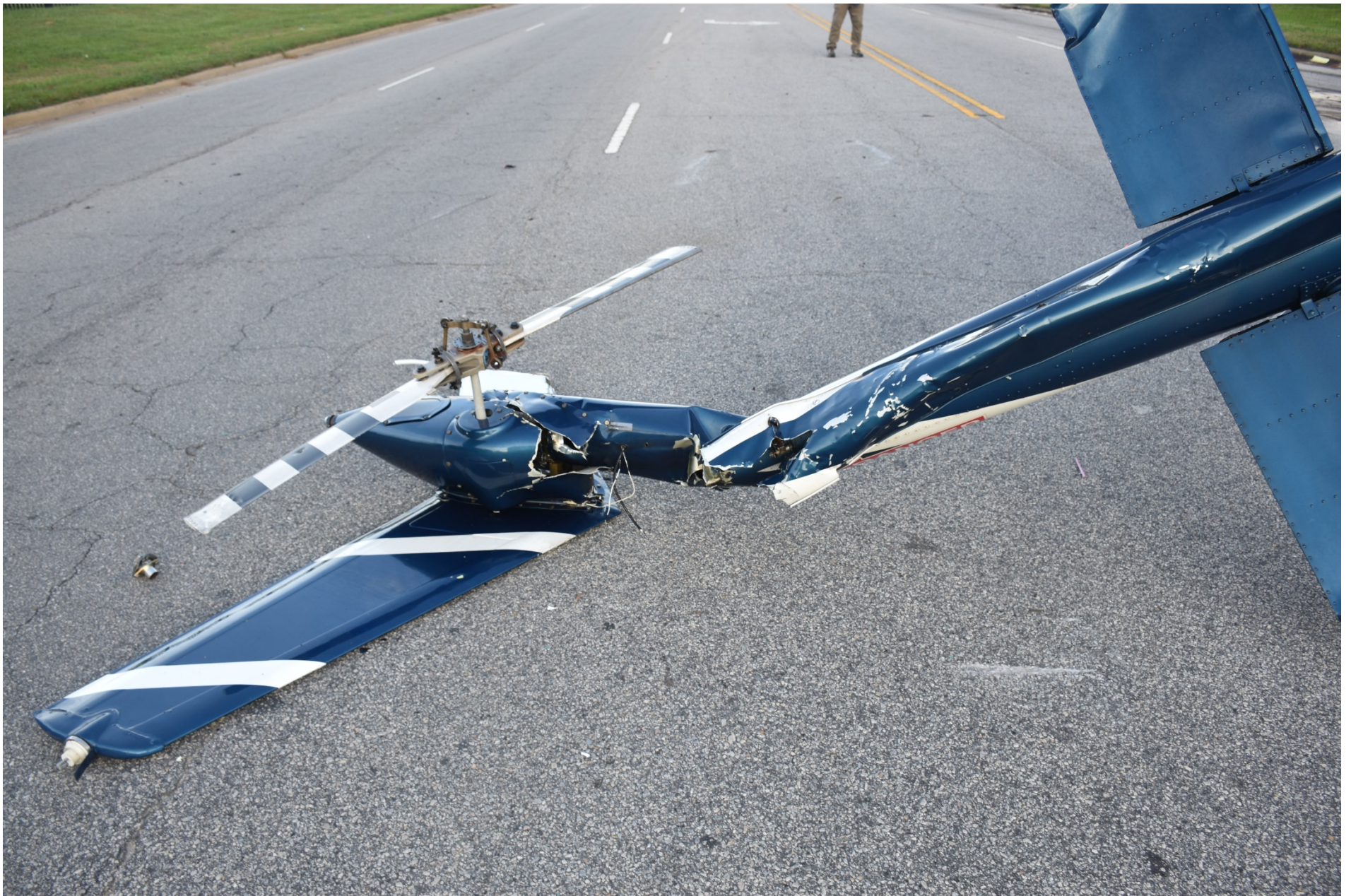
Photo 3 - Digital Photograph From NC Highway Patrol. View of the Aft Portion of the Tailboom and Tail Rotor Assembly.
