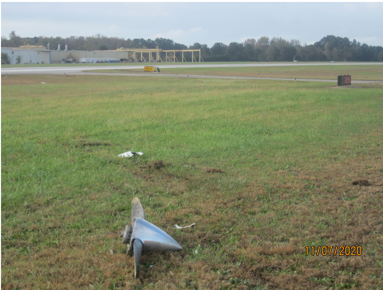
Photo 3 – Photograph of the runway and damage path. Note the separated propeller. (Courtesy of FAA)
