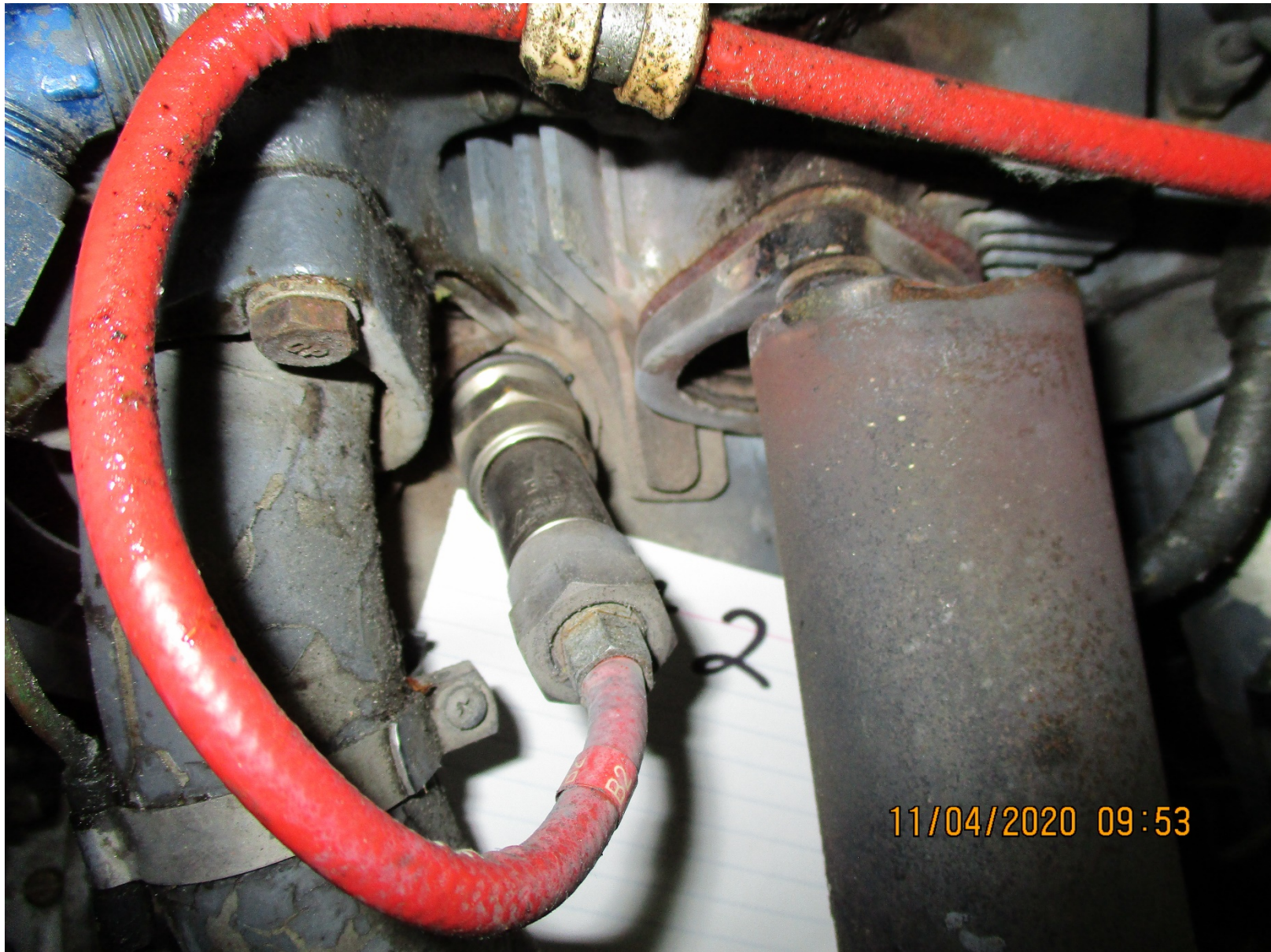
No. 2 Cylinder Soot on Spark Plug Lead (IMG0171 - Photo Courtesy FAA)
