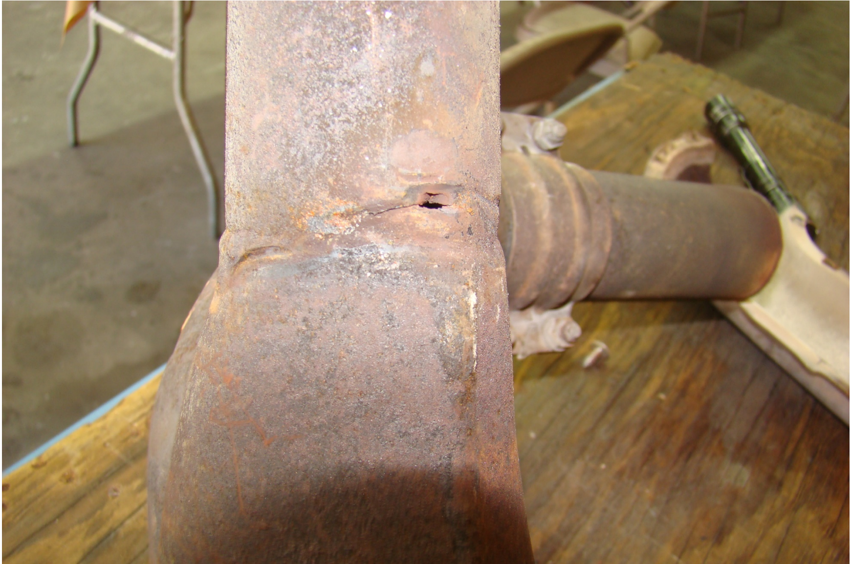
Left Side Exhaust Riser – Hole/Crack (Photo Courtesy FAA)
