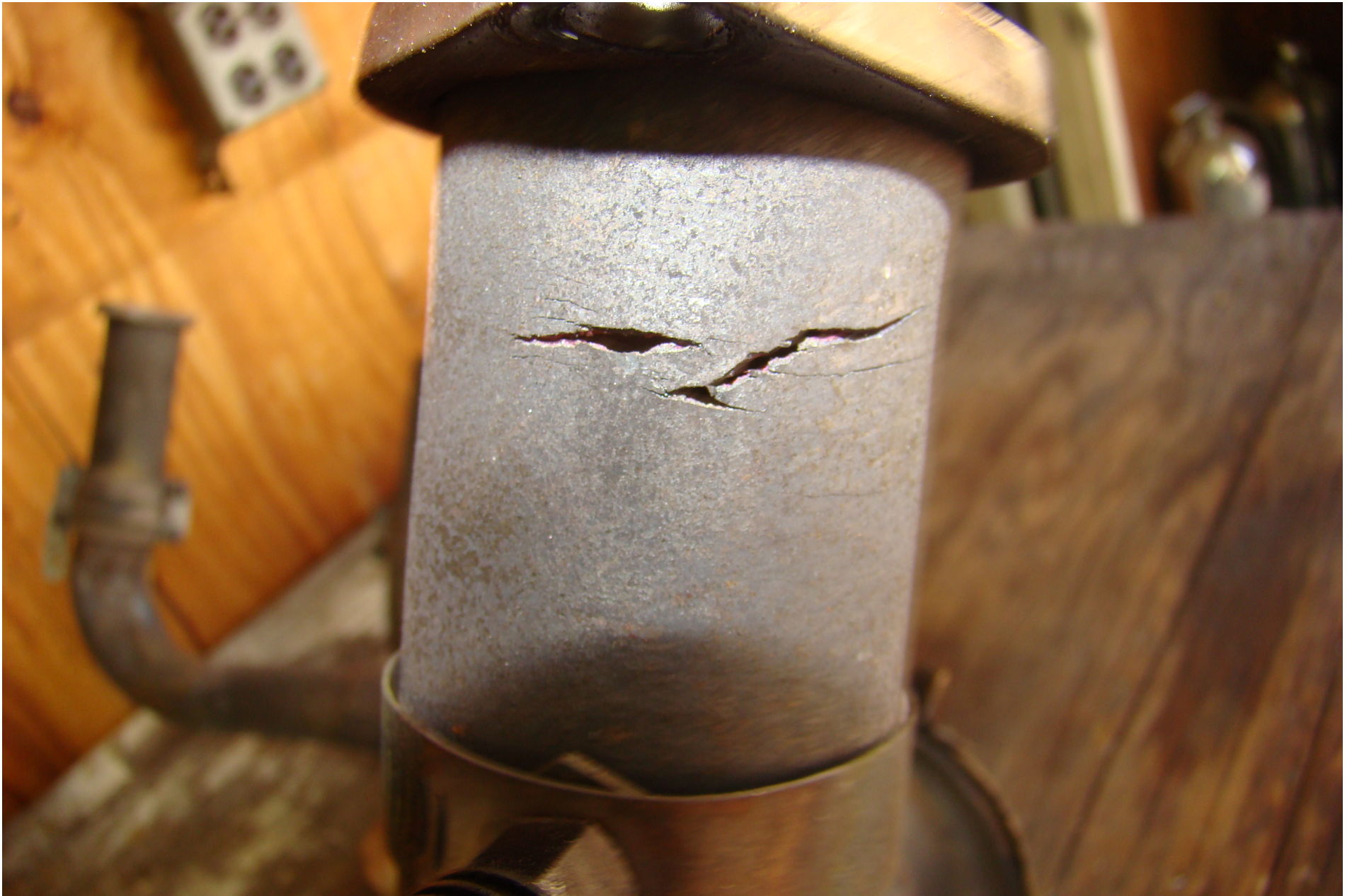
No. 3 Cylinder Exhaust Tube Cracks (Photo Courtesy FAA)
