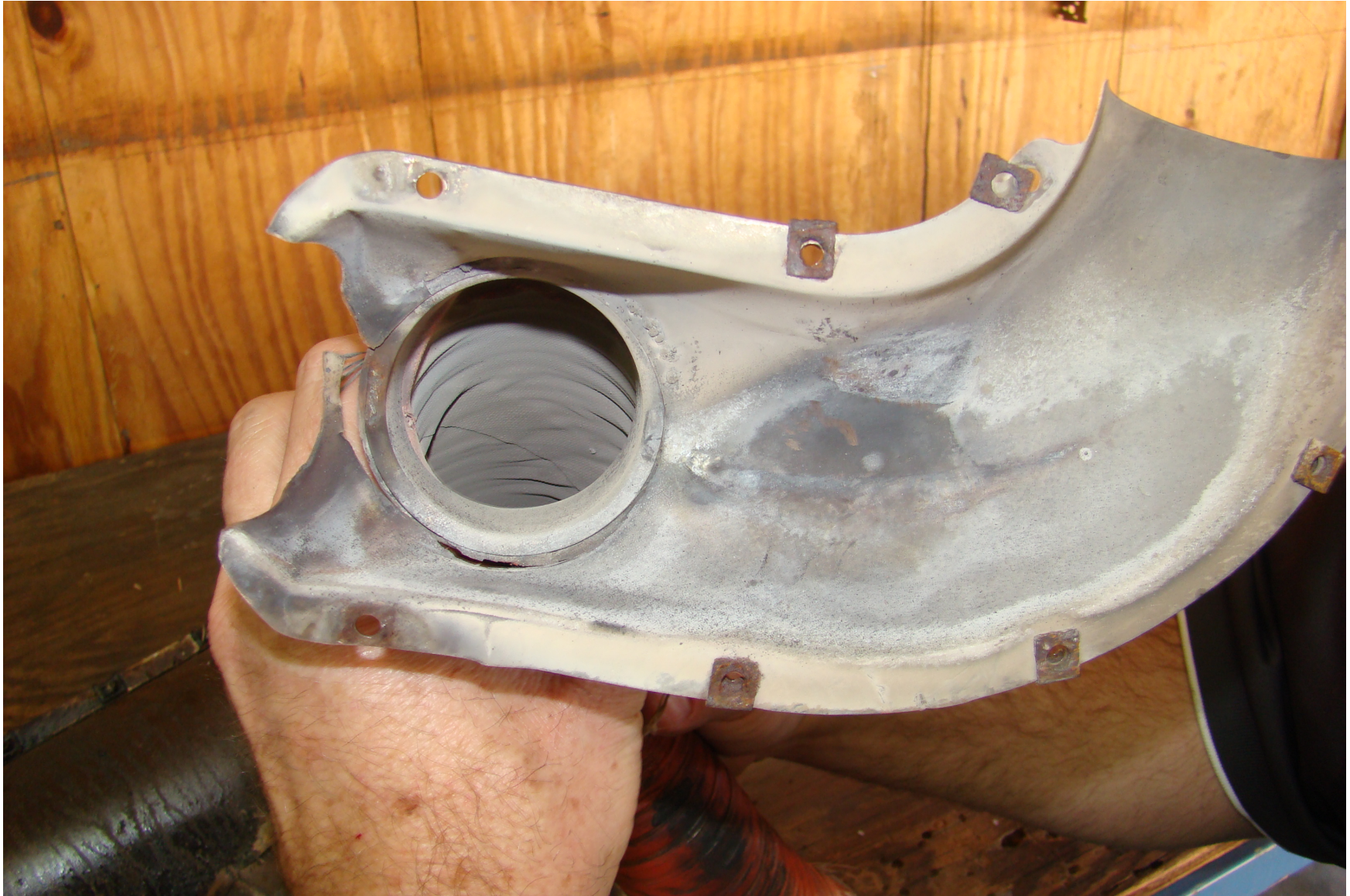
Soot in Carburetor Heat Muff and Tube (Photo Courtesy FAA)
