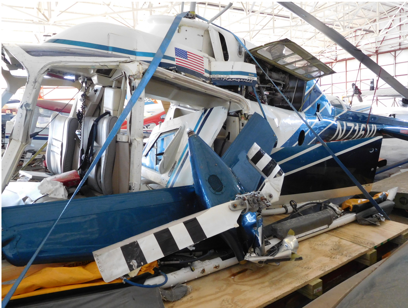
Photo 2 – Digital Photograph From Insurance Adjuster. Left side View of the Helicopter Following Recovery, also Depicting Recovered Tail Rotor Assembly.
