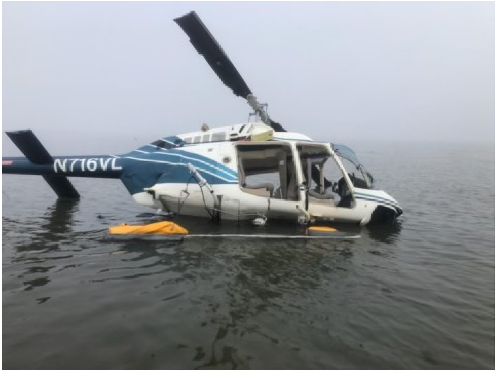
Photo 1 – Digital Photograph From Nassau County Police Department Aviation Unit. Right Side View of the Helicopter. Note the Separated Doors and Displaced Crosstubes.
