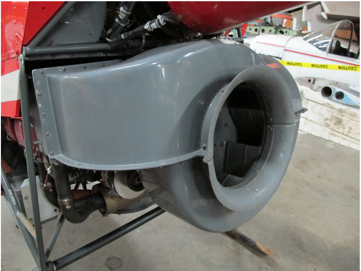
Above and below: Cooling scroll and fan.
