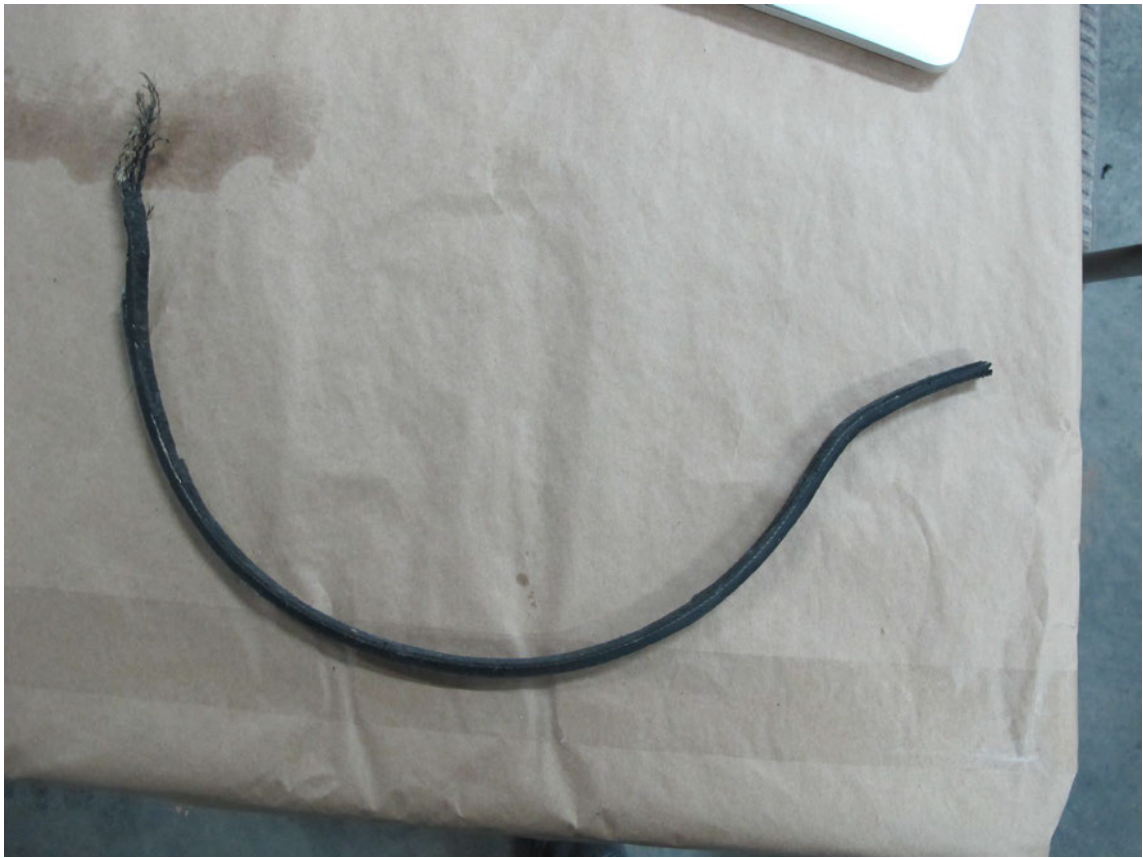
Above and below: The remaining portion of V-belt.
