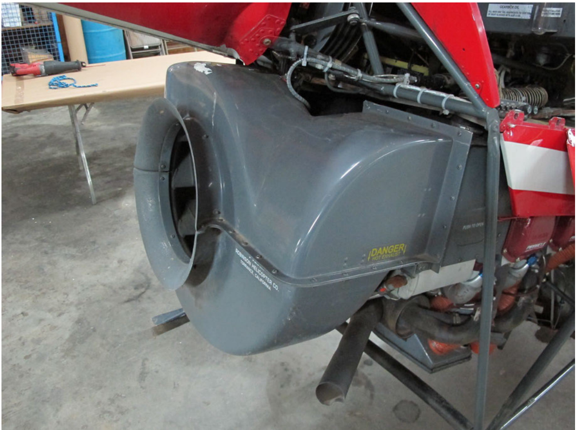
Above and below: Cooling scroll and fan.
