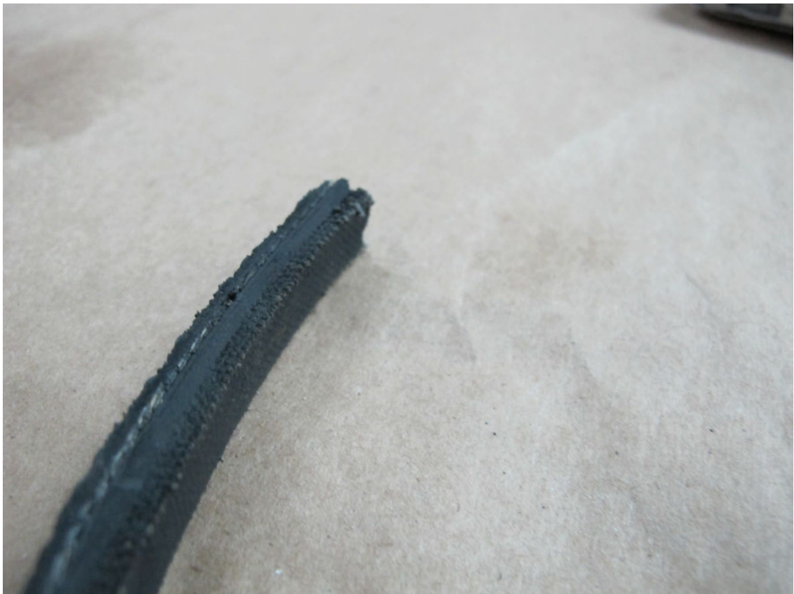
Above and below: The remaining portion of V-belt.
