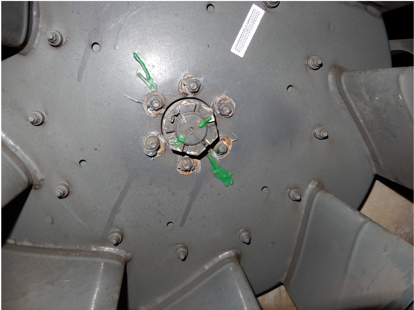
Photo 8 – Fanwheel Assembly (NTSB Photo)
