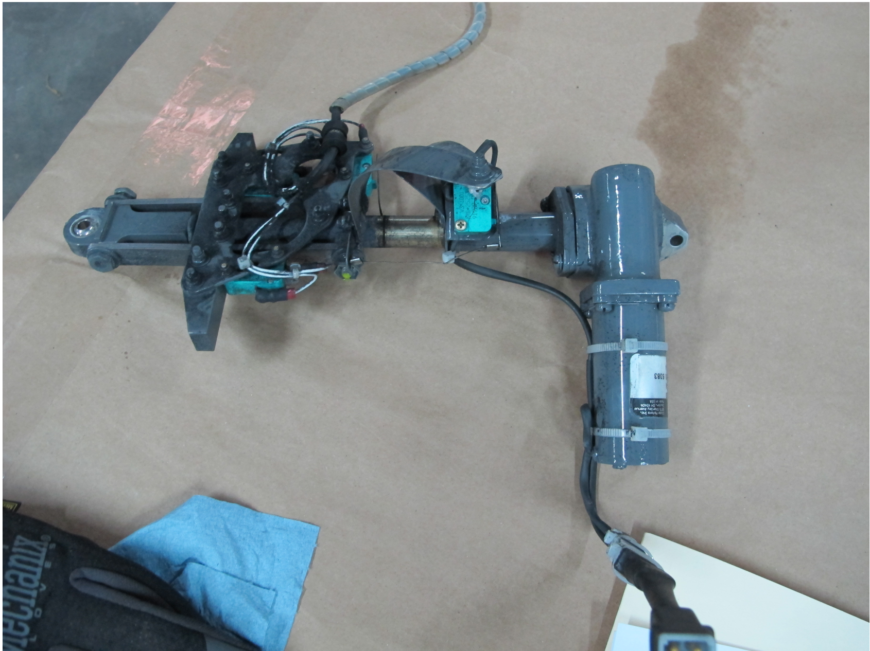
Photo 9 – Belt Tension Actuator (Robinson Helicopter Photo)
