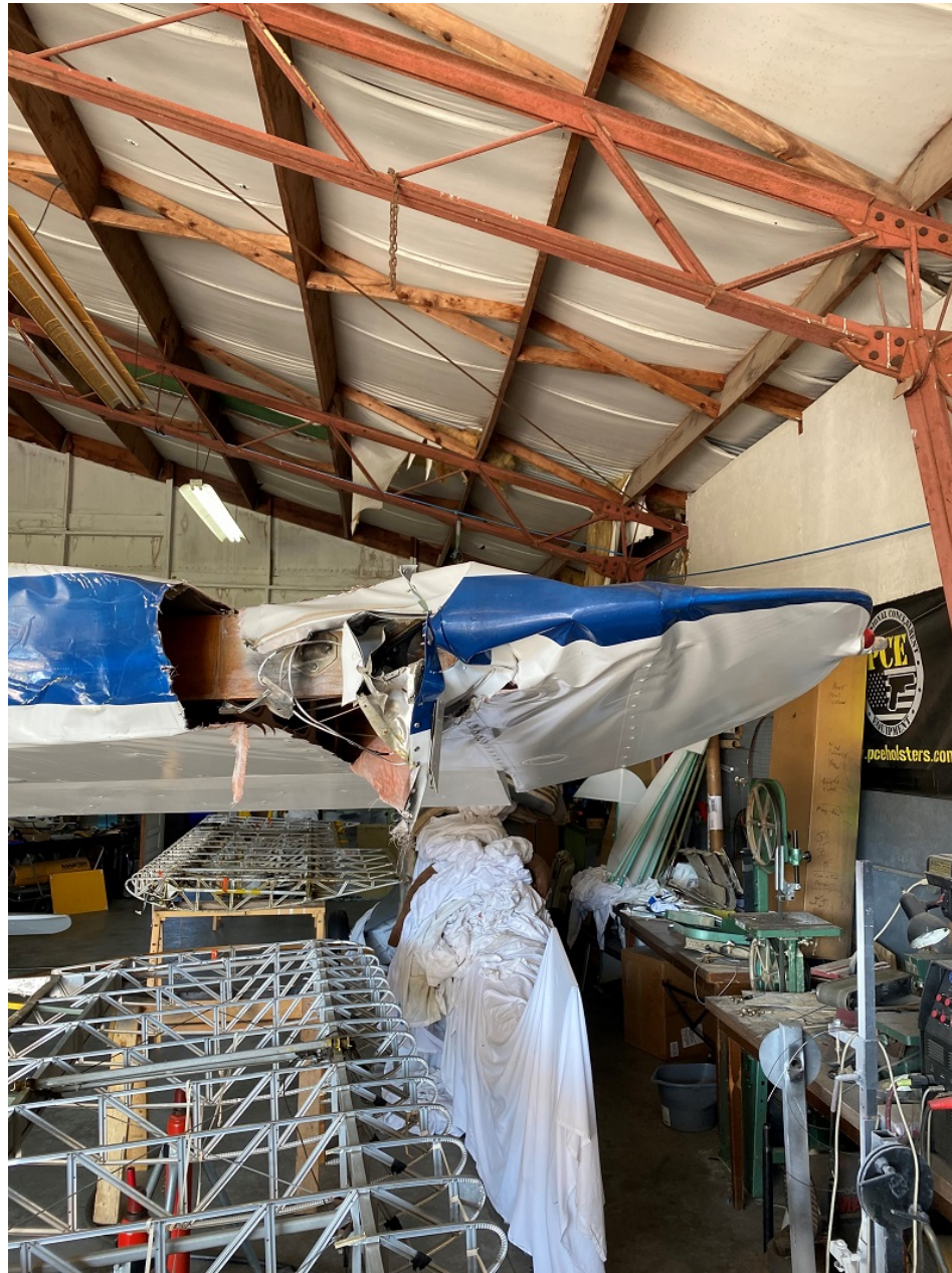
Photo 2 – Left Wing Damage (Photo Courtesy of FAA)
