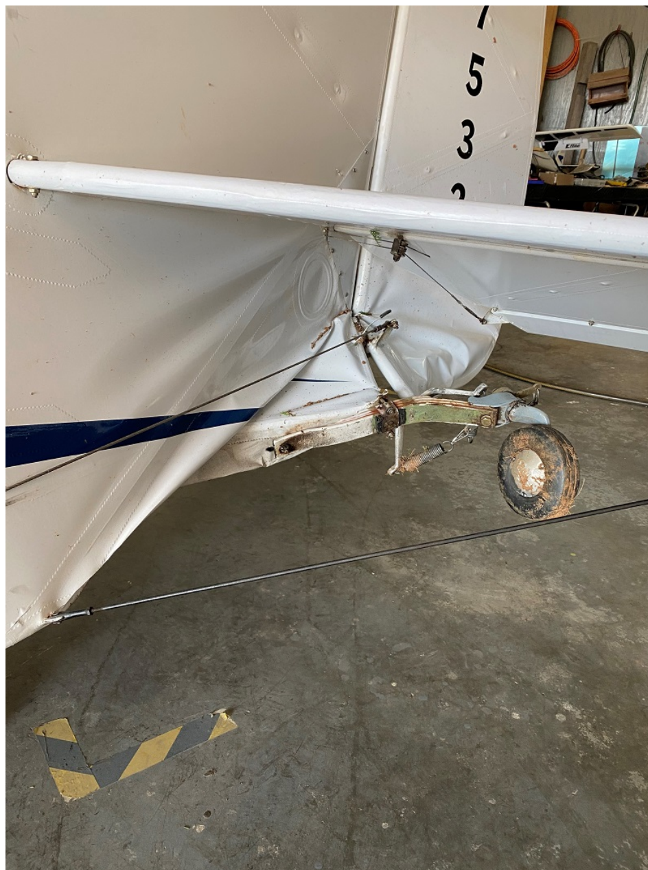
Photo 3 – Empennage Damage (Photo Courtesy of FAA)
