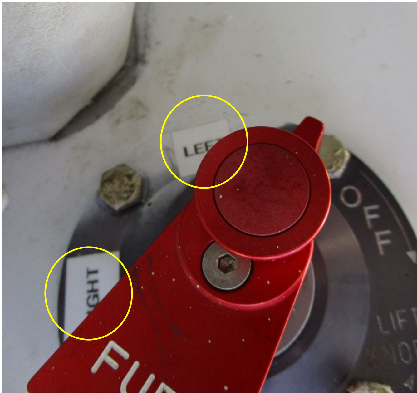
Figure 1 – View of the fuel selector placards, mislabeled. Left was right, right was left (Photo Courtesy of FAA)
