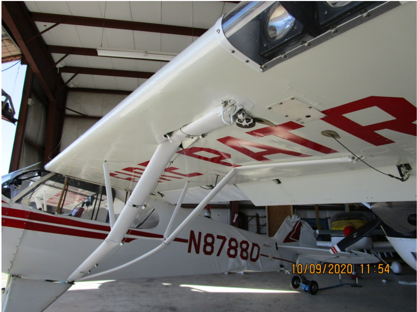
Photo 2 - Digital Photograph Provided by FAA. Left Side View of the Airplane Following Recovery. Note the Damage to Both Left Wing Lift Struts.
