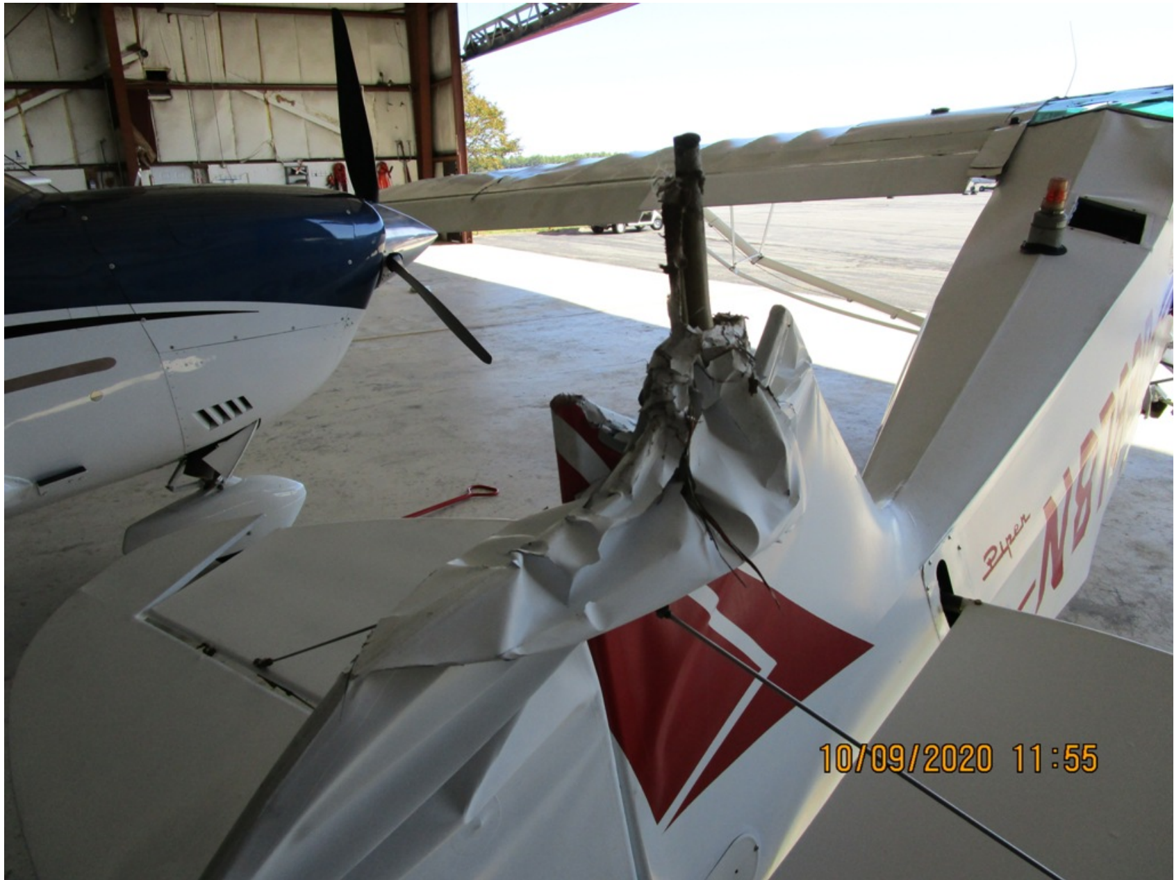
Photo 3 - Digital Photograph Provided by FAA. Right Rear View of the Airplane Following Recovery. Note the Damage to the Rudder and Vertical Stabilizer.
