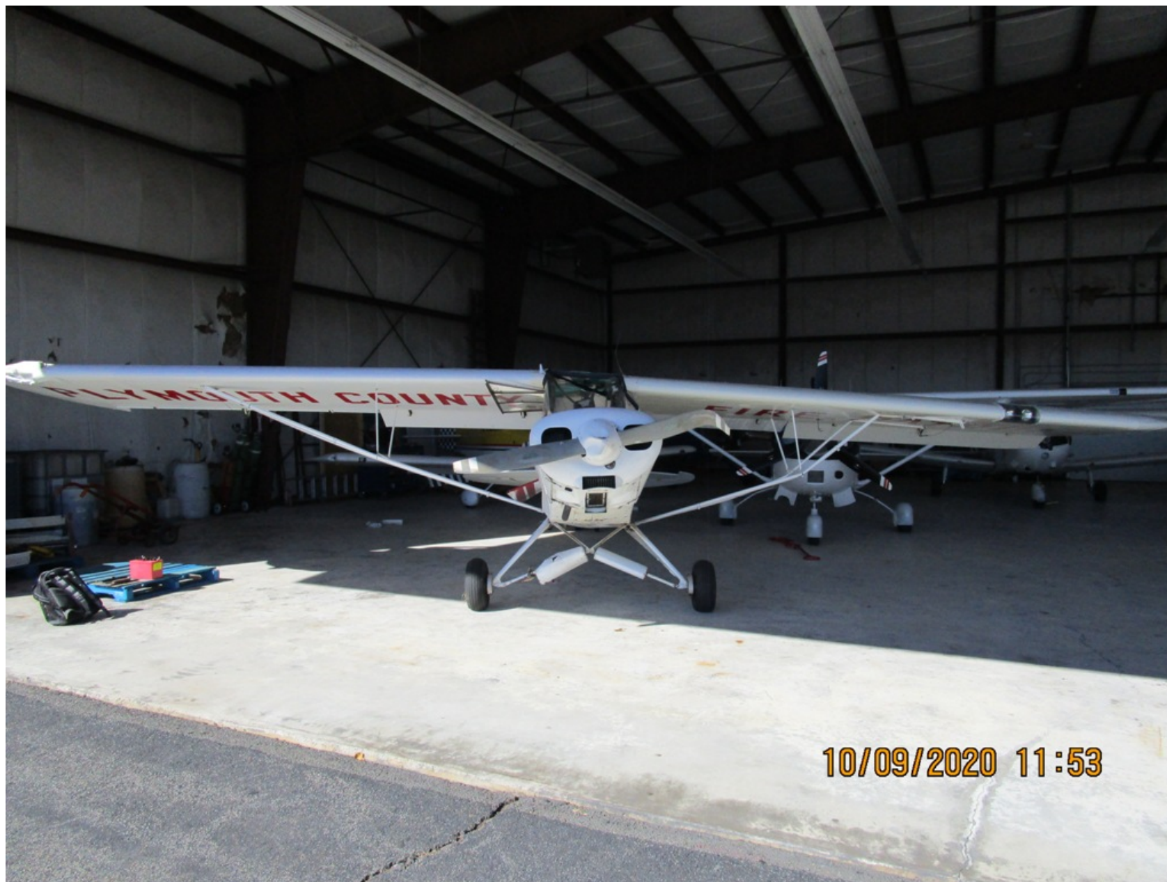
Photo 1 – Digital Photograph Provided by FAA. Frontal View of the Airplane Following Recovery. Note the Abnormal Position of the Left Wing, Damaged Propeller Blade, and Damage at the Right Wing Tip.
