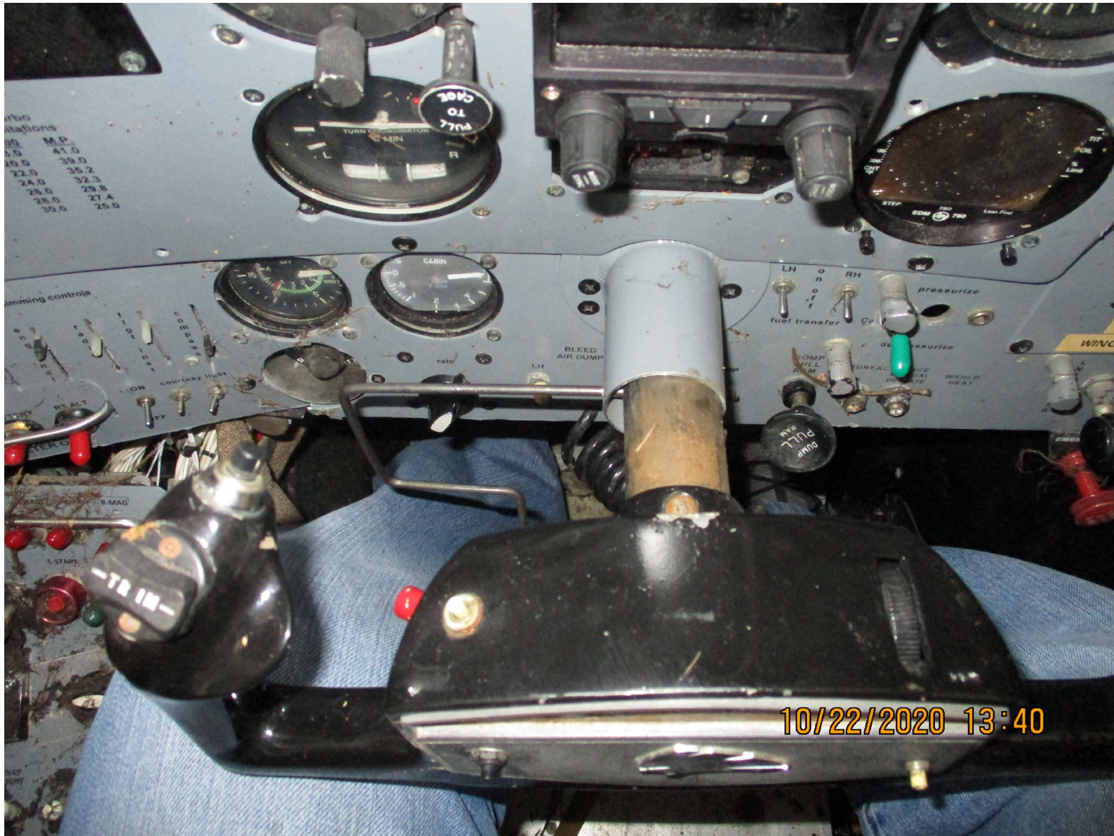
Photo 3 – Pilot seat control lock installed on left side of column looking down. (Courtesy of FAA)
