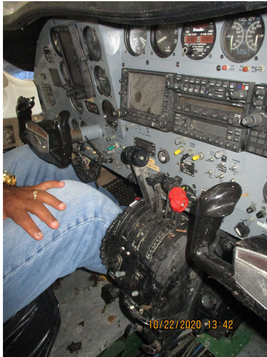
Photo 5 – Copilot’s view of pilot control lock installed on the right side of the column. (Courtesy of FAA)
