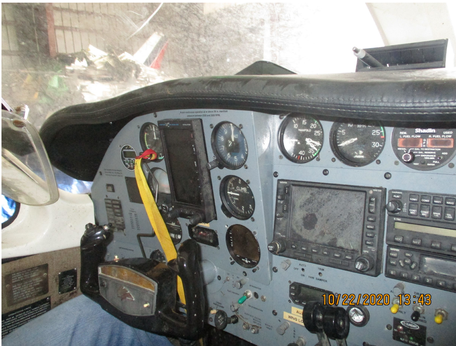
Photo 6 – Control lock installed in a vertical position with flag on top. (Courtesy of FAA)
