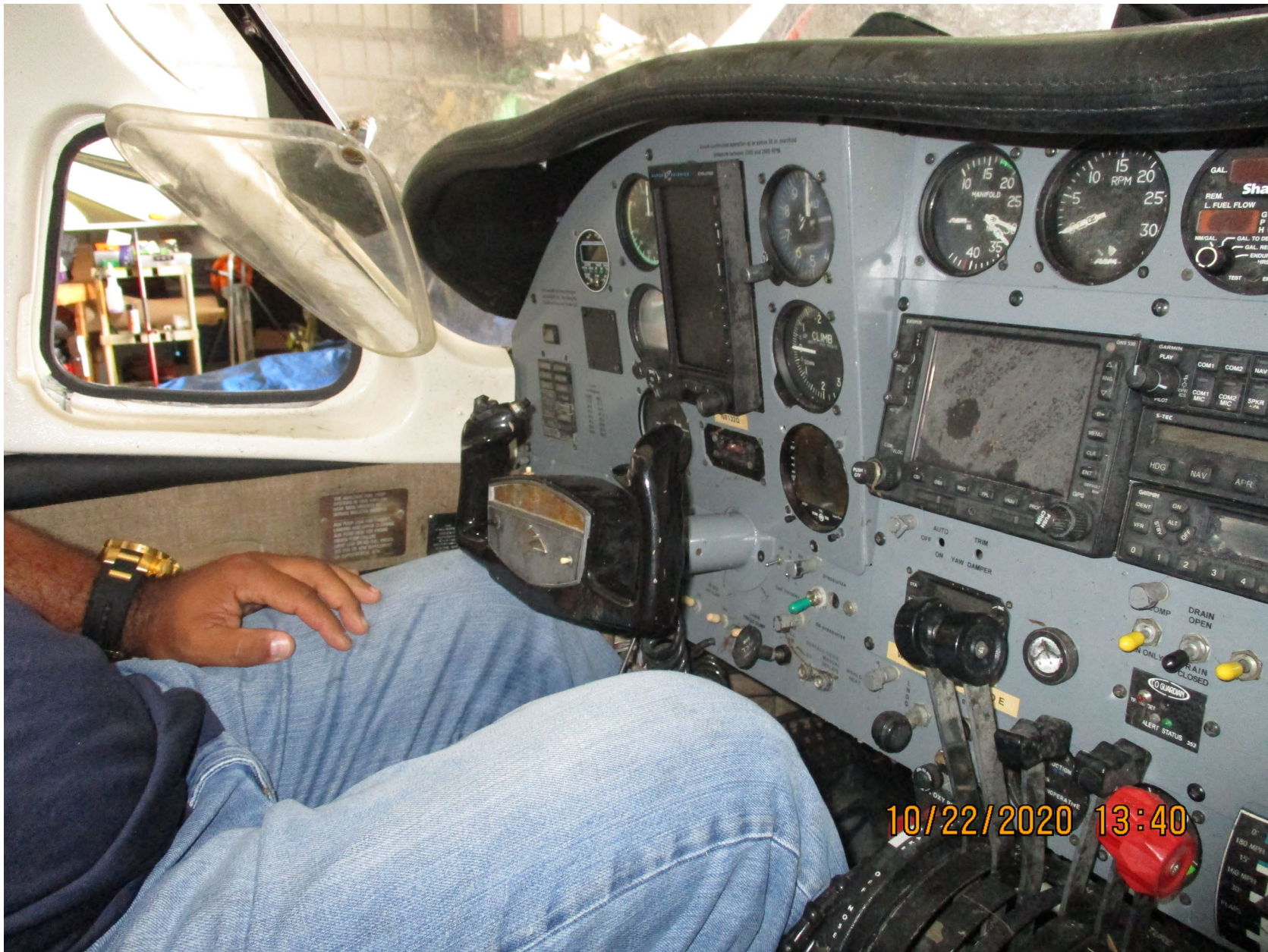
Photo 2 – Right seat (Co-pilot's view) of control lock installed. Note FAA Inspector sitting in pilot seat. (Courtesy of FAA)
