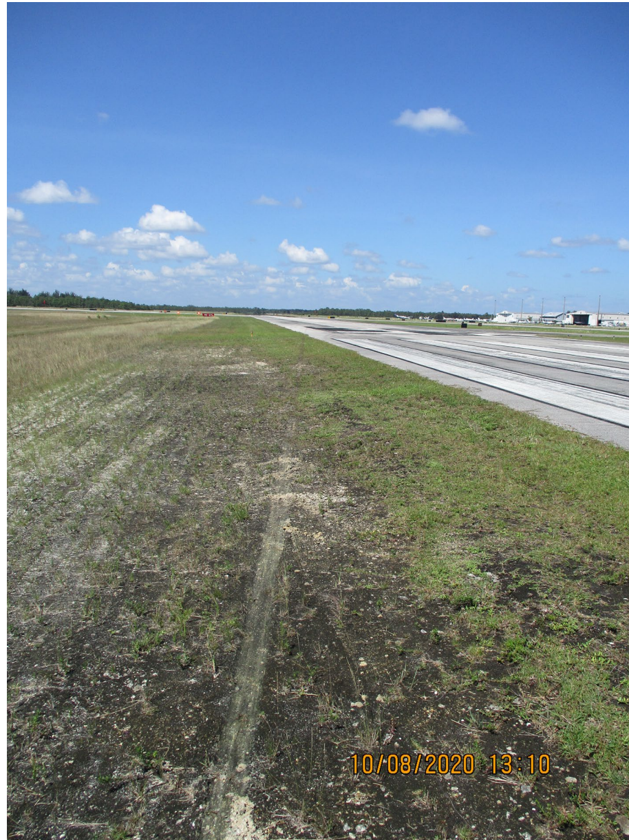
Photo 11 – View of tire skid marks looking back towards runway 14. (Courtesy of FAA)
