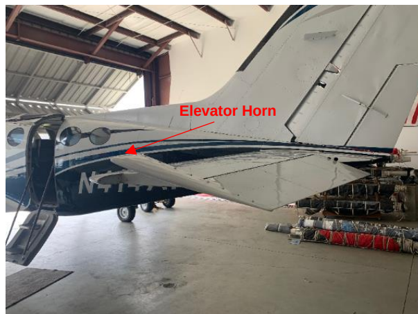
Figure 4. A exemplar photo of a Cessna 414 with an elevator control lock installed. The elevator is fixed in a trailing edge down position. Elevator horns are seen on the edge of the horizontal stab and above the horizontal stab.
