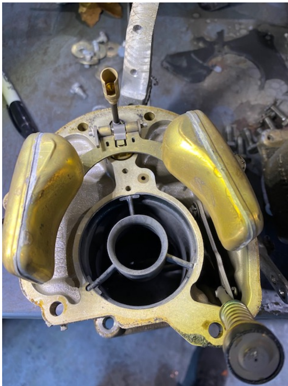
Photo 6 – Carburetor Floats (Photo Courtesy of Florida Air Recovery)
