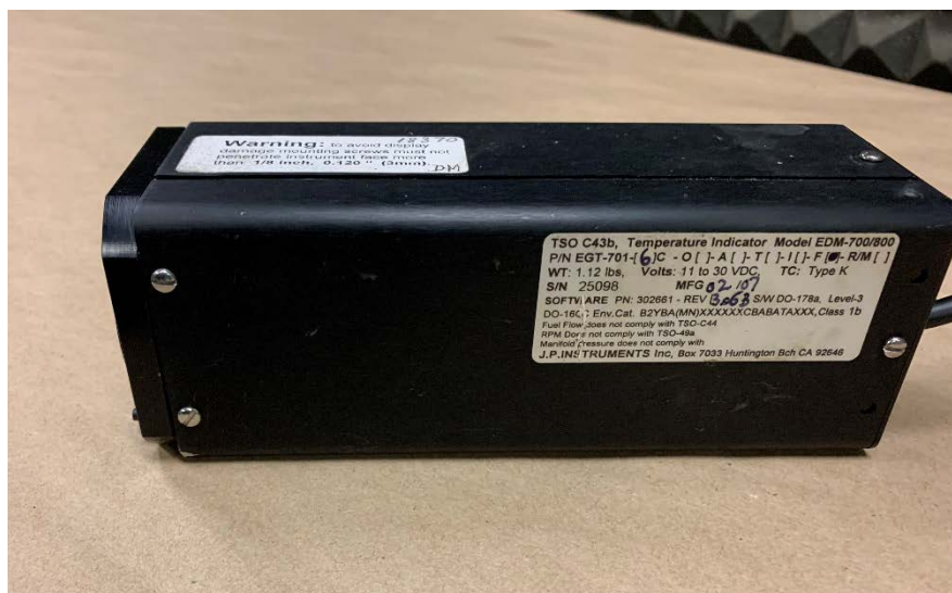
Figure 2. View of side of engine data monitor
