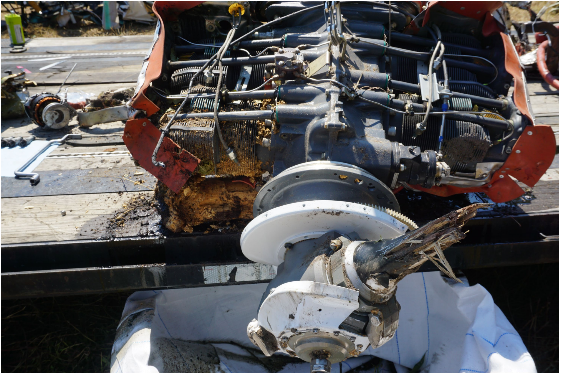
Photo 4 – View of engine and propeller showing impact damage.
