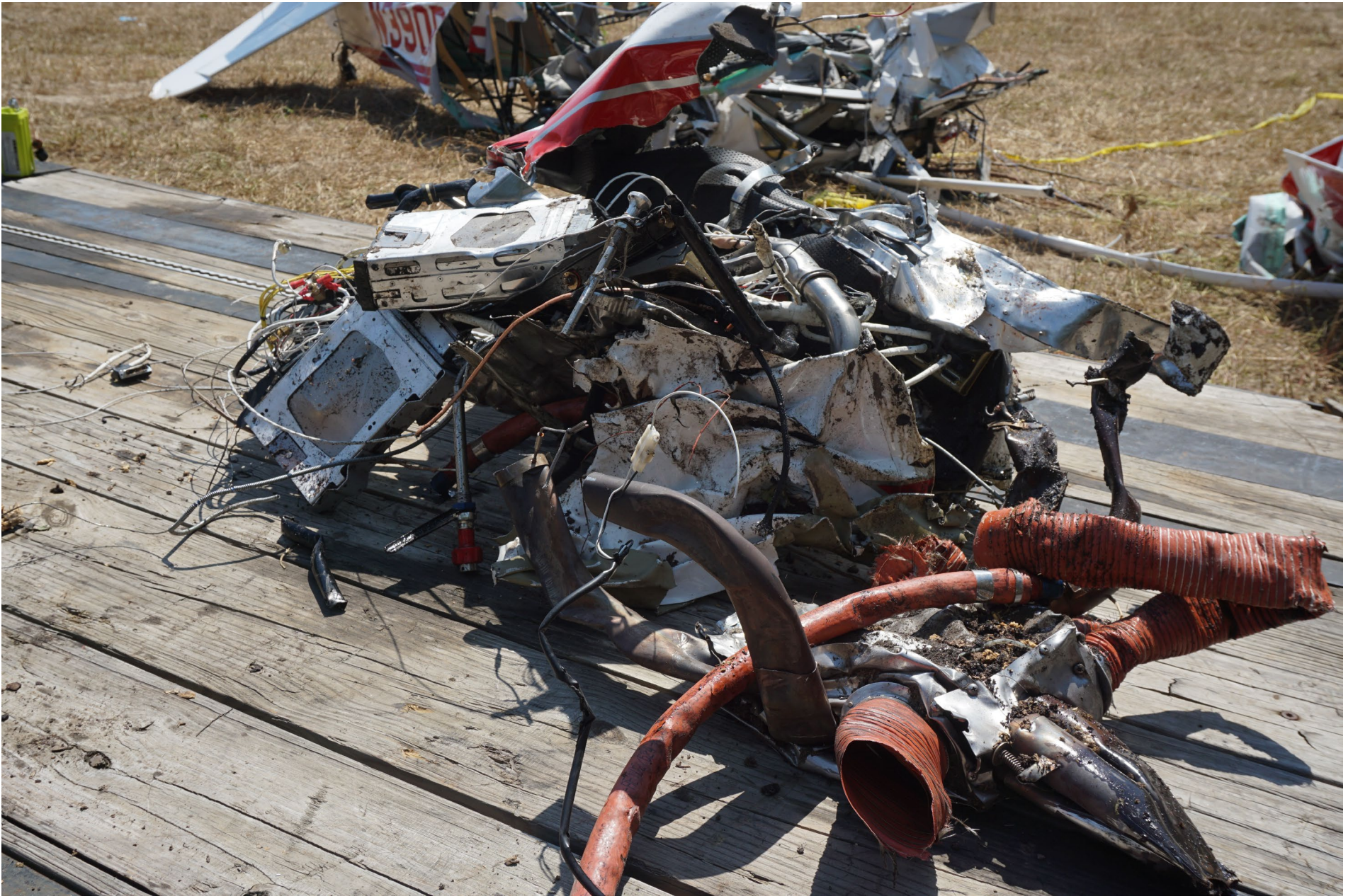
Photo 3 – View of instrument panel showing impact damaged.
