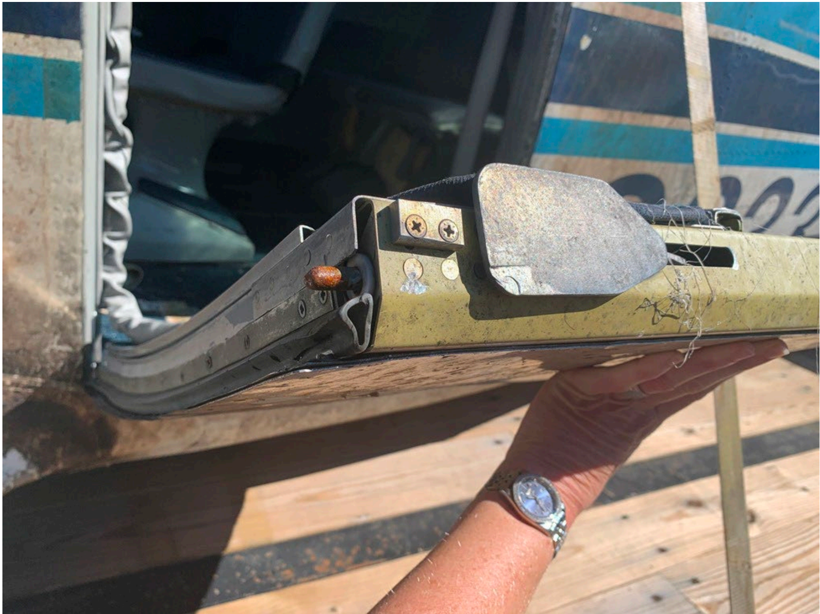
Photo 6 – Main Cabin Lower Door Handle and Locking Pin in Locked Position
