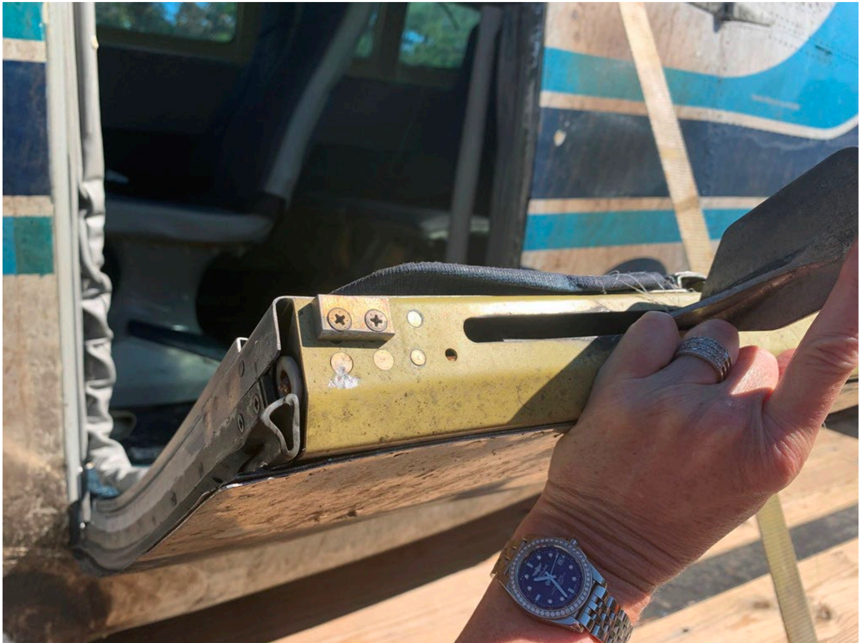
Photo 7 - Main Cabin Lower Door Handle and Locking Pin in Unlocked/Open Position
