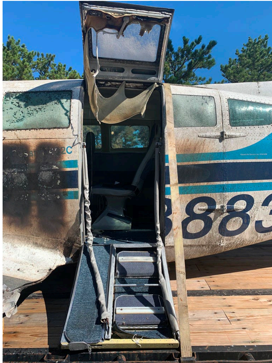
Photo 5 – Main Cabin Door Extended on Flat Bed Truck Post-Recovery
