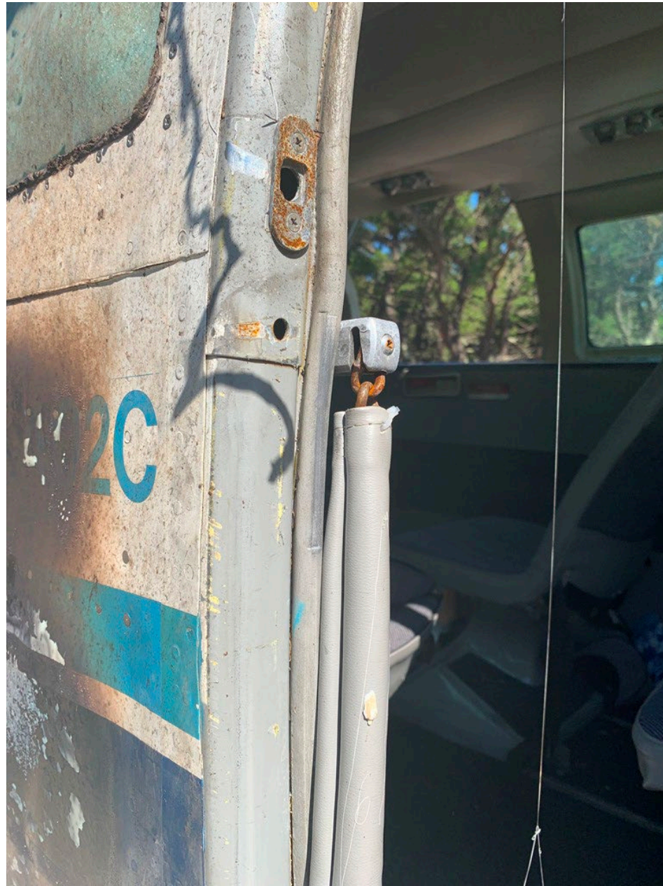
Photo 8 – Main Cabin Door Upper Strike Plate and Lower Latching Bore
