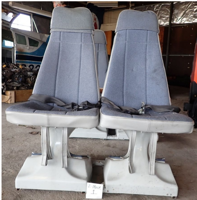
Figure 9. Two rigid seat buckets attached to pedestals which are connected to each other with frame.
