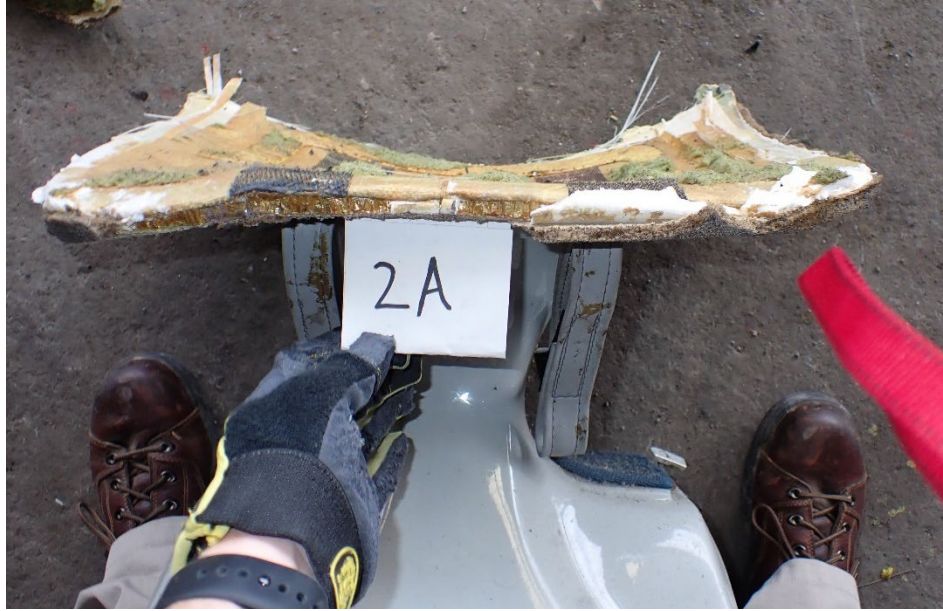
Figure 12. View of seat pan from the front showing damage to the forward right portion of the pan.
