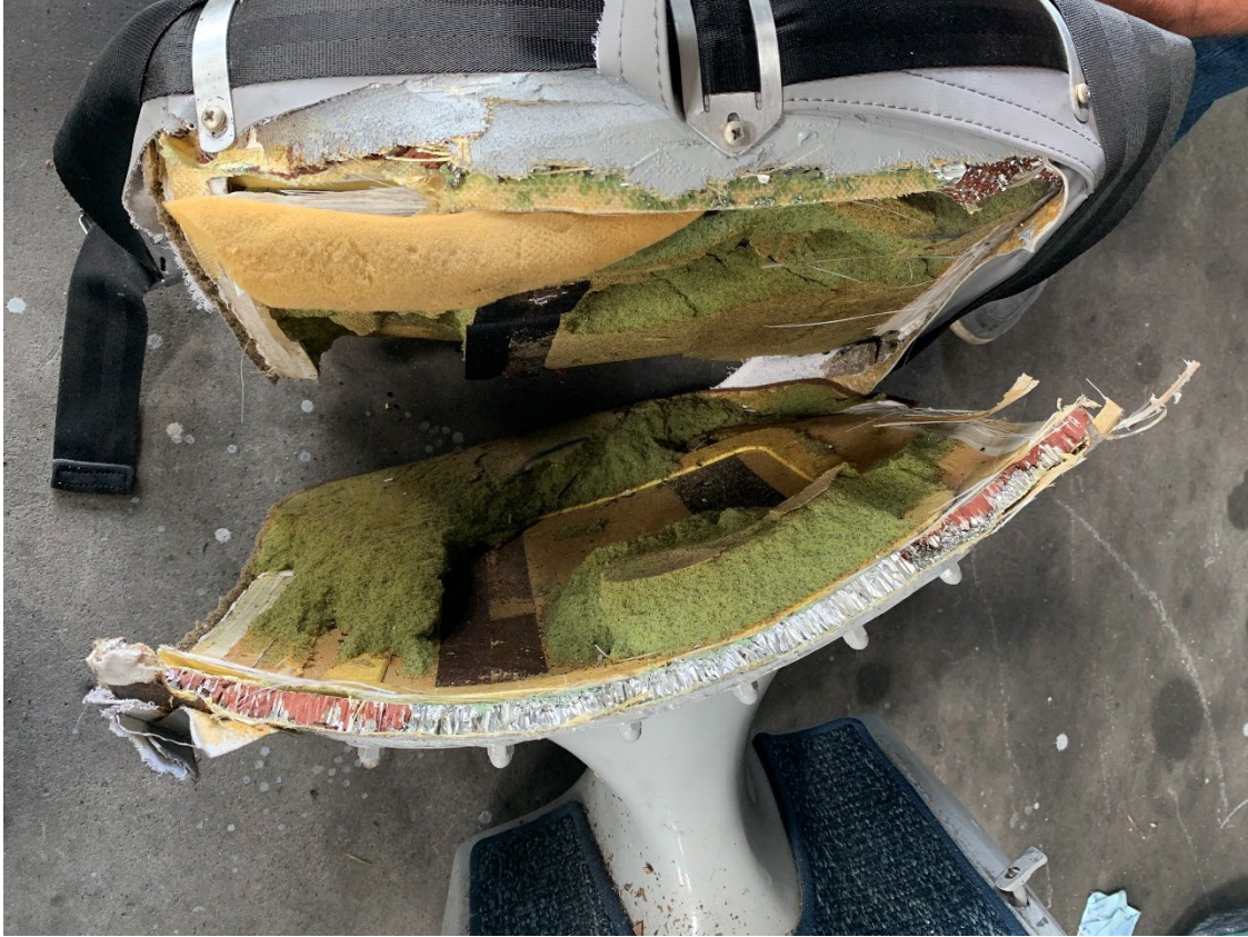
Figure 11. Seat 2A viewed from the rear with broken section lifted away revealing damage to the seat bottom cushion.
