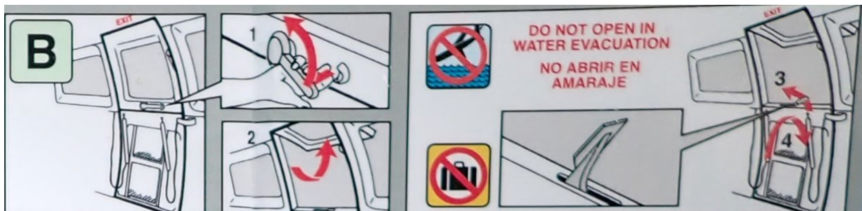
Figure 20. Directions for opening the main cabin door from the Cape Air briefing card.
