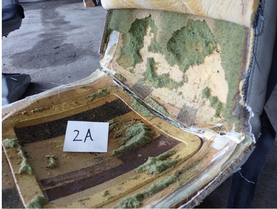
Figure 14. Seat 2A with covering and foam removed from seatpan and the lower portion of the seatback.
