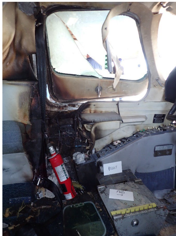
Figure 5. Photograph of charring aft of the pilot seat after the pilot seat was removed.
