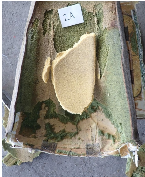
Figure 13. Seat 2A seatback with covering and foam removed to show crumpling on the bottom left section of the structure.
