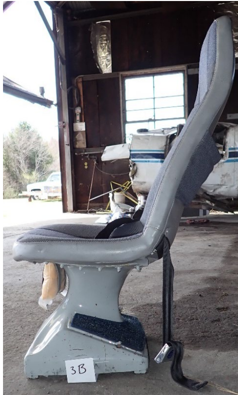
Figure 8. Solid seat bucket passenger seat with no motion built in for the seatback.
