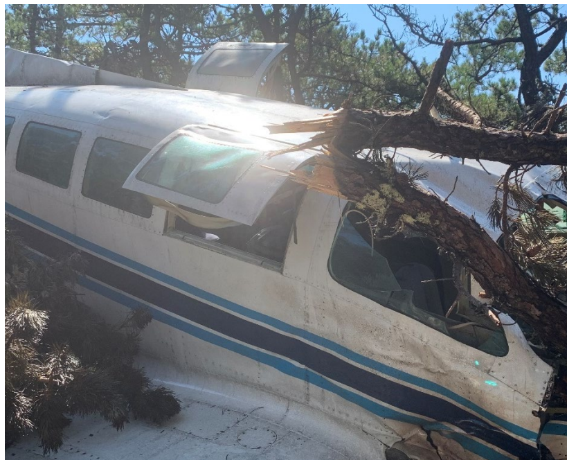
Figure 18. Right escape hatch located adjacent to seat 2B, as found after the fire was extinguished.
