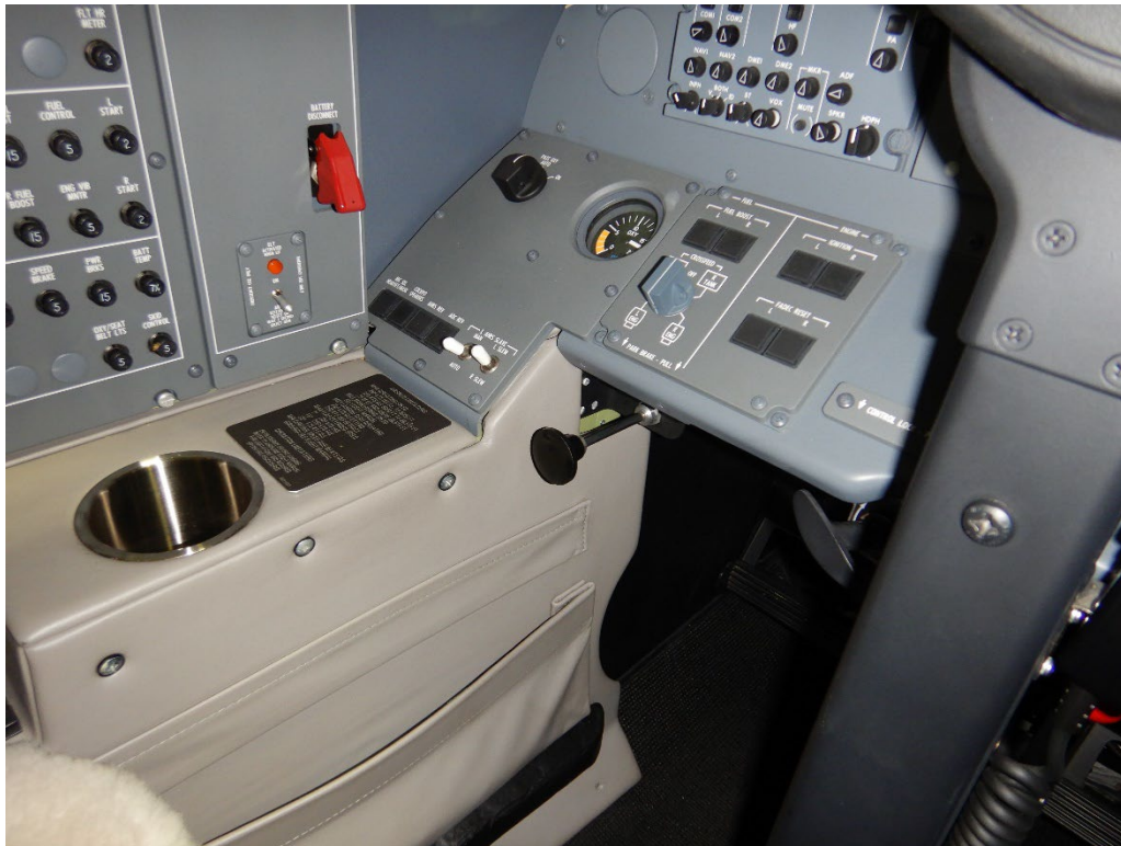
Figure 1: Digital Photograph From Textron Aviation. View of the Park Brake Handle in Pulled Position of an Exemplar Airplane.
