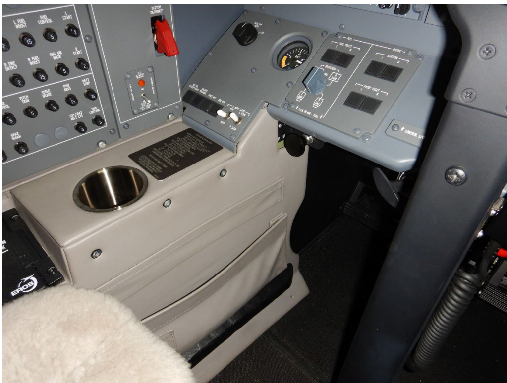
Figure 2: Digital Photograph From Textron Aviation. View of the Park Brake Handle in the Released Position of an Exemplar Airplane.
