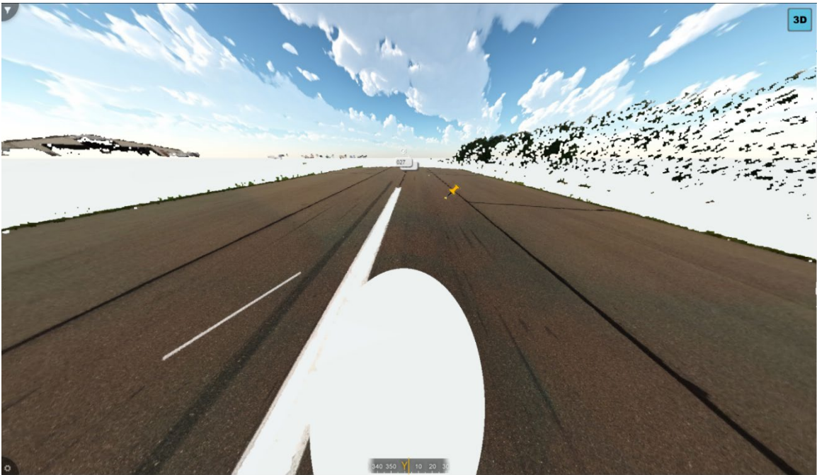
Figure 4: Faro Image From Scan Station 26 Located About 2,326 Ft From Approach End of Runway 2. Pin indicates 1 st identified Location of the Tire Mark Made by the Right Main Landing Gear Tire 2,360.9 Ft and about 9 Ft Right of Runway Centerline.
