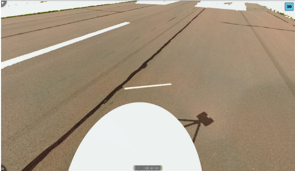
Figure 10: Faro Image From Scan Station 43 Located About 3,337 Ft From Approach End of Runway 2. Marks from Left and Right Main Landing Gear Tires with Grooves of both Noted.
