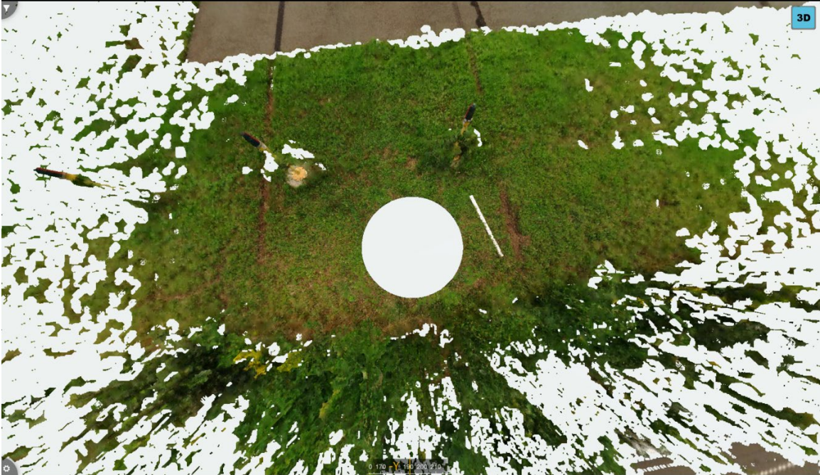
Figure 15: Faro Image From Scan Station 49 Located At Edge Of Airport Terrain Before Terrain Drop. Note marks from Both Main Landing Gear Tires in Grass.
