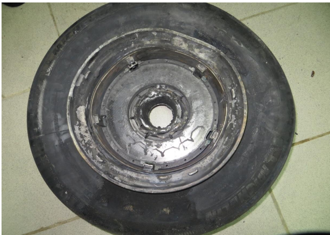
Figure 7: Damaged main landing gear wheel assembly
