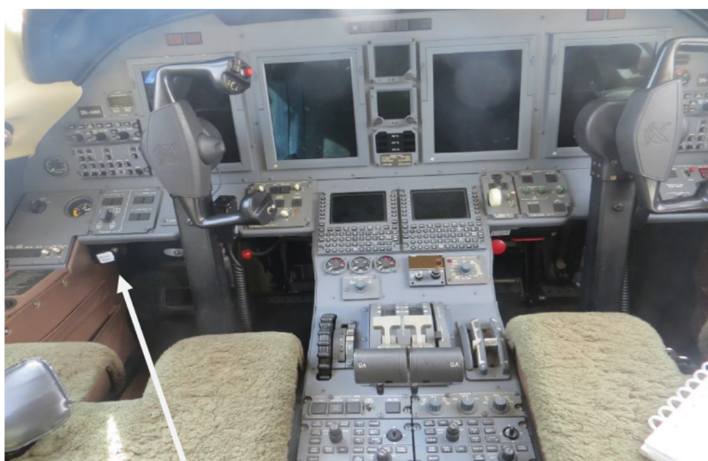
Figure 2: Parking brake position in the cockpit
