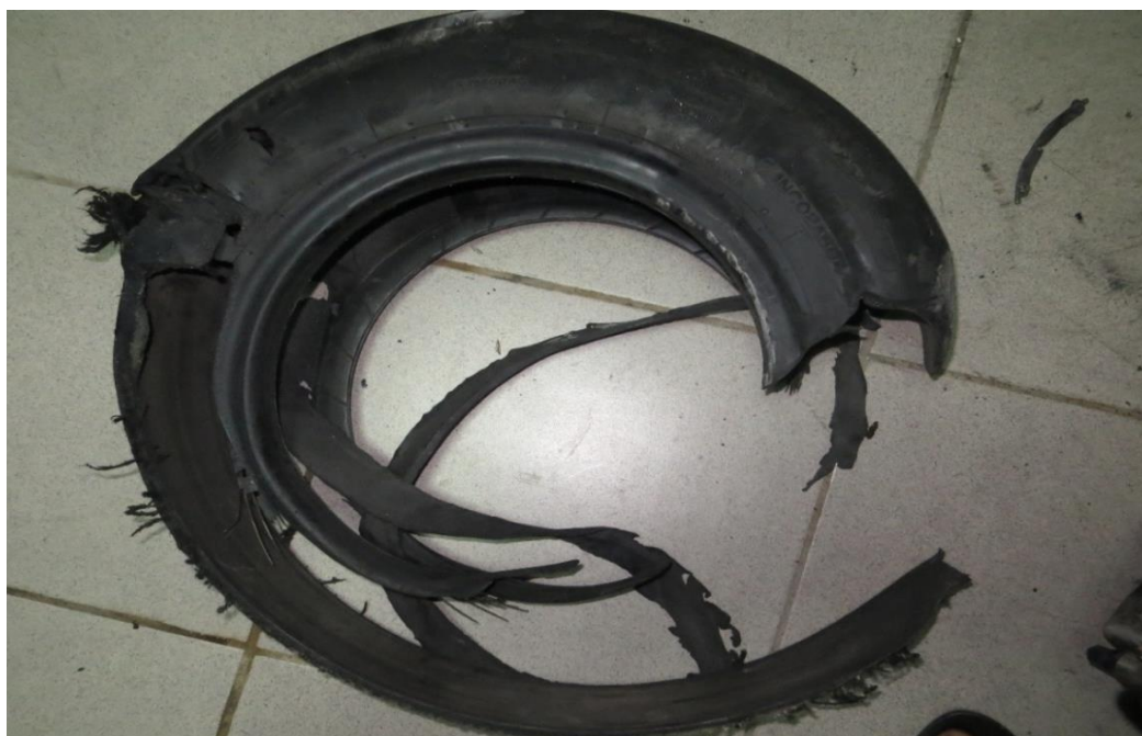
Figure 4: Burnt main landing gear tyre
