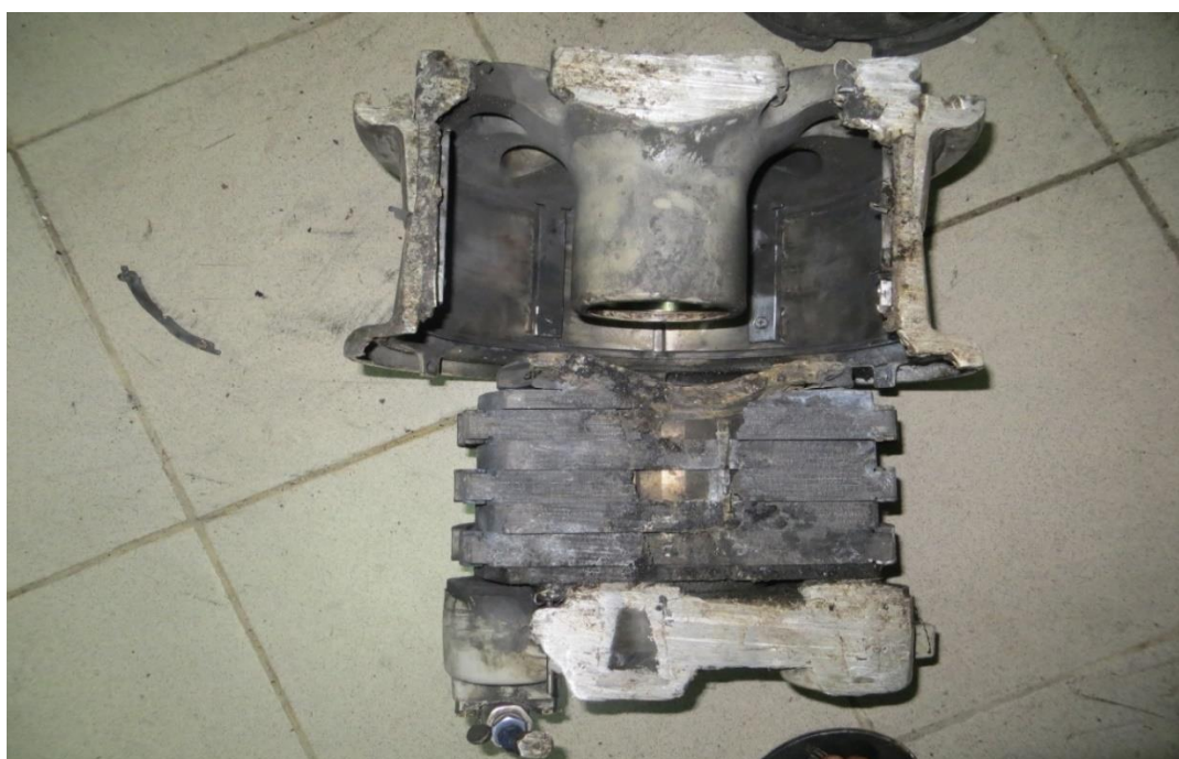
Figure 5: Damaged main landing gear brake assembly
