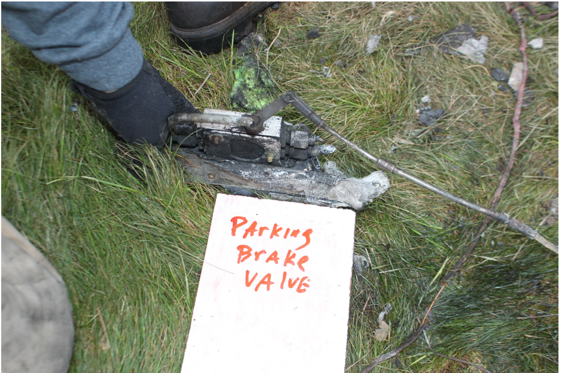
Photo 8 - NTSB Digital Photograph. View of the Parking Brake Valve and Attached Cable after Recovery From the Wreckage.
