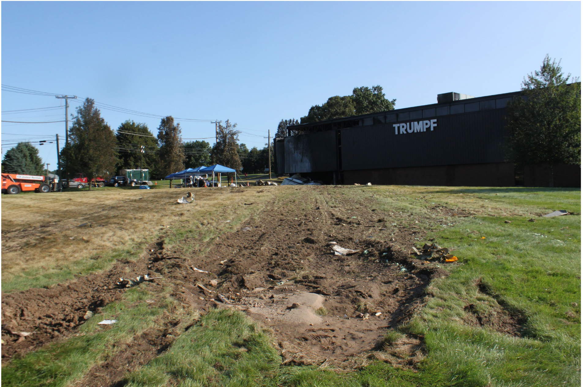
Photo 2 - NTSB Digital Photograph. View Looking at the Ground Impact Location Consistent with the Top Portion of the Fuselage with the Main Wreckage in the Background.
