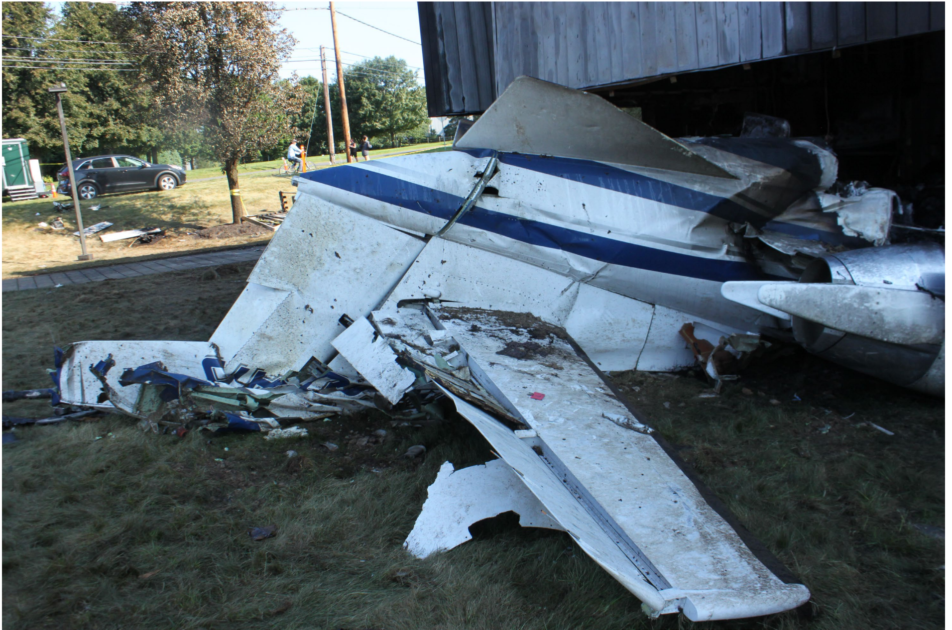
Photo 4 - NTSB Digital Photograph. Left Side View of the Inverted Aft Empennage at the Accident Site.
