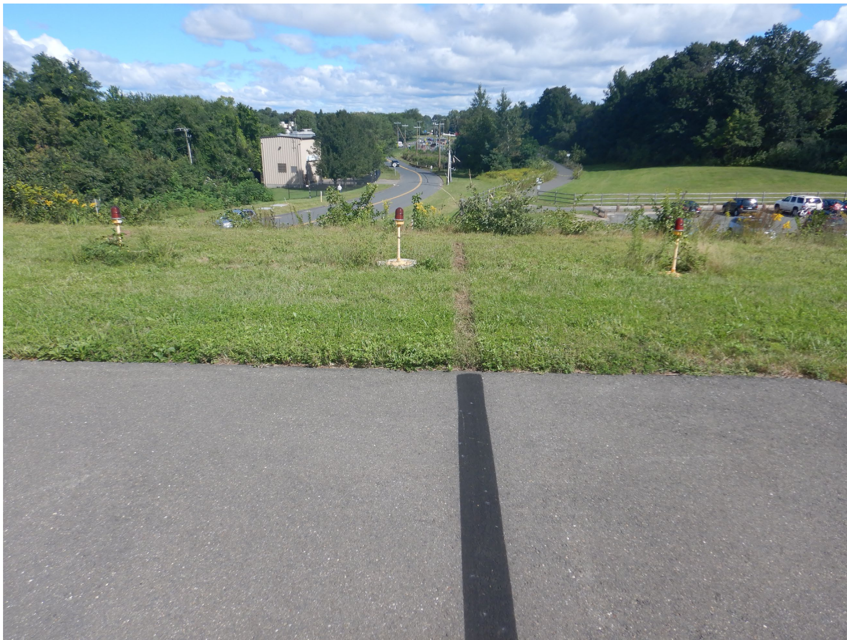
Photo 17 - Textron Aviation Digital Photograph. View Taken Near the Departure End of the Runway Showing the Right Main Landing Gear Tire Mark. Note the Lack of Drainage Grooves in The Tread.
