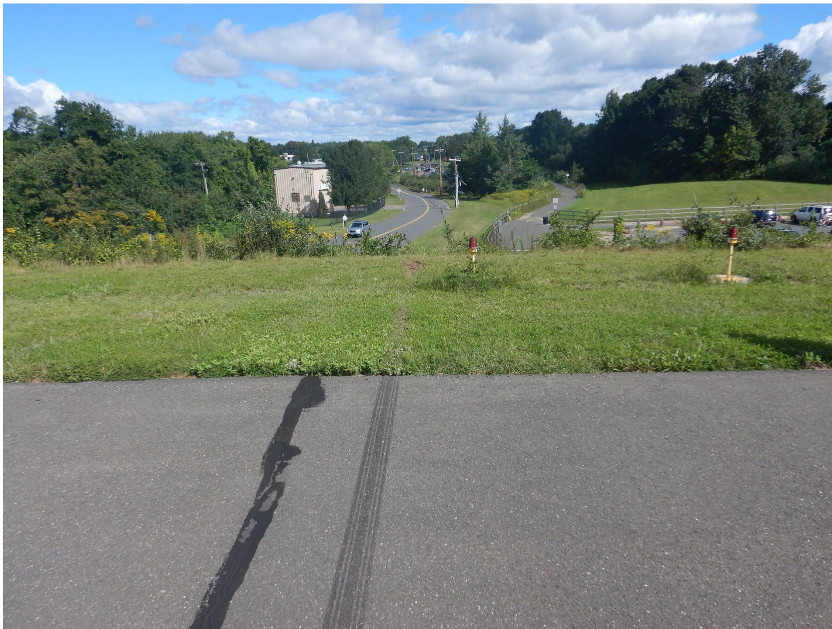
Photo 16 - Textron Aviation Digital Photograph. View Taken Near the Departure End of the Runway Showing the Left Main Landing Gear Tire Mark. Note the Drainage Grooves in The Tread.
