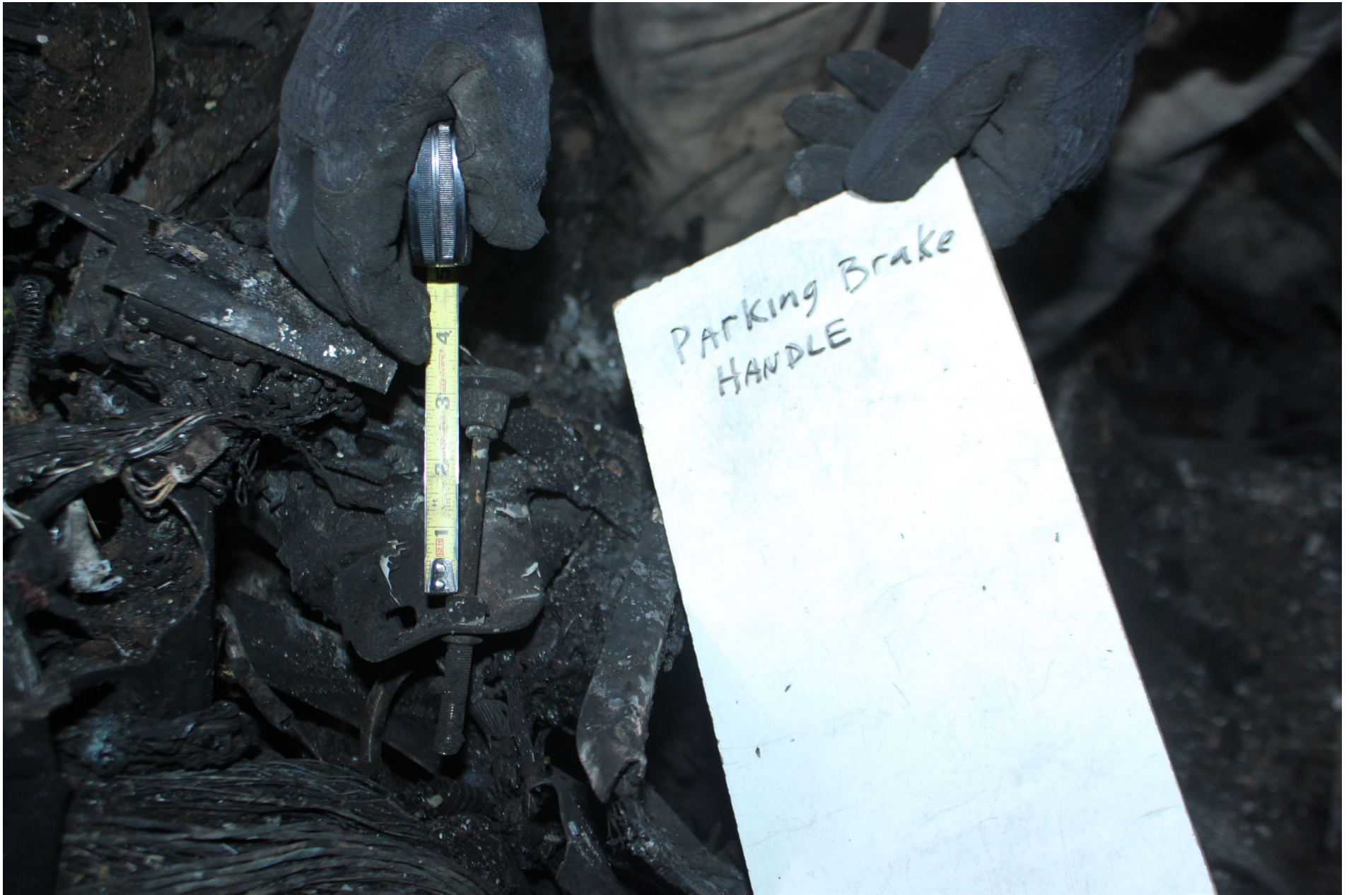
Photo 9 - NTSB Digital Photograph. View of the Parking Brake Knob as First Found in the Wreckage. Note the Approximate Extension of 2.5 Inches.
