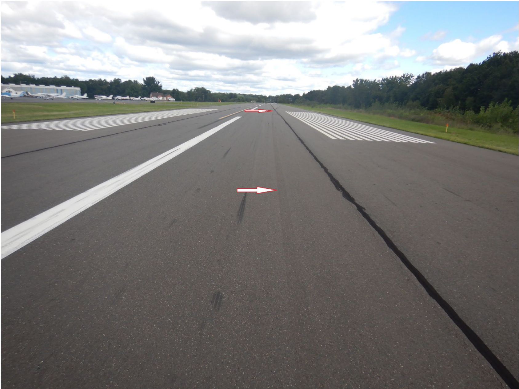
Photo 11 – Textron Aviation Digital Photograph. Arrows Point to Right Main Landing Gear Tire Mark. Note the Deviation to the Right.
