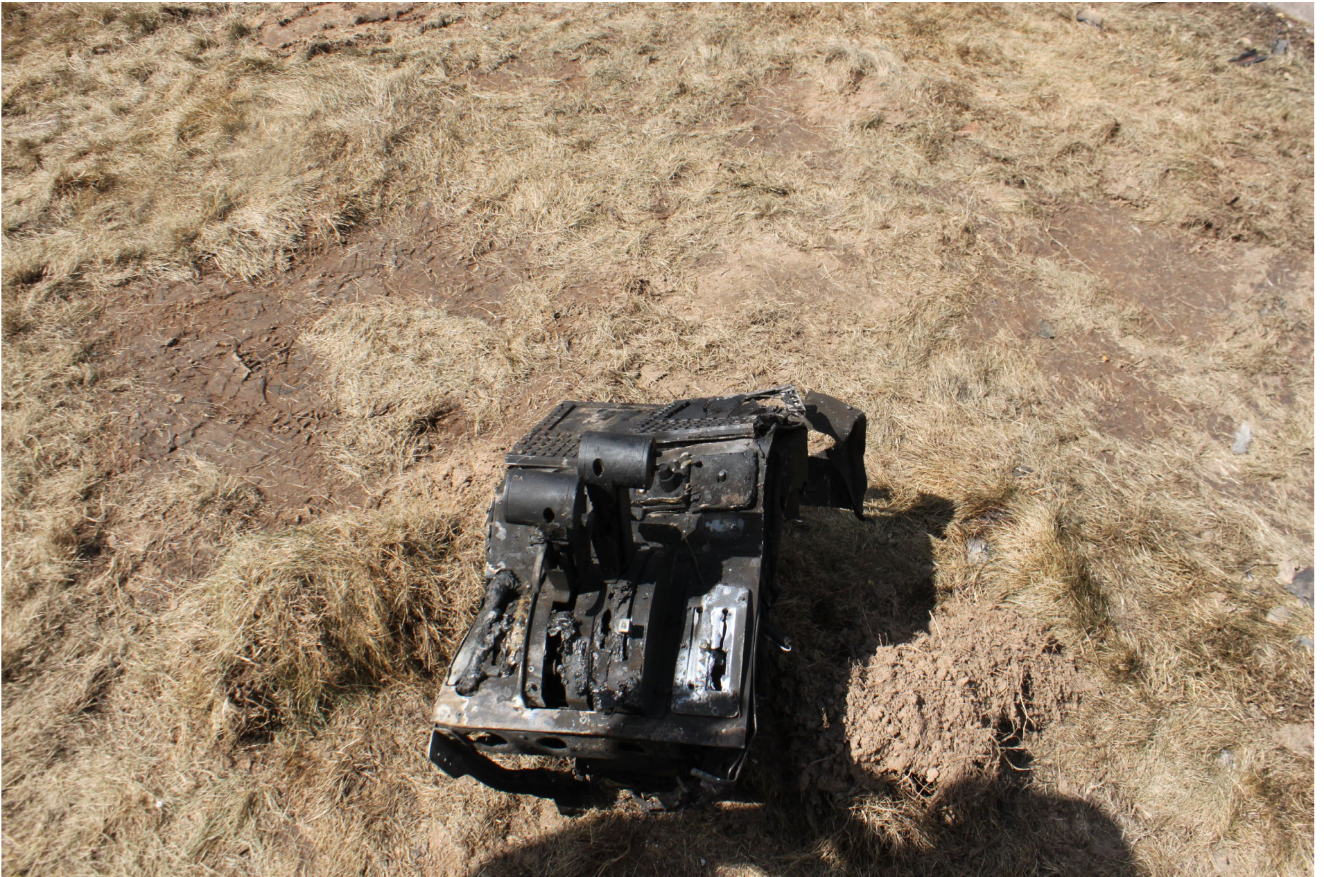
Photo 6 - NTSB Digital Photograph. View of the Separated Throttle Quadrant.
