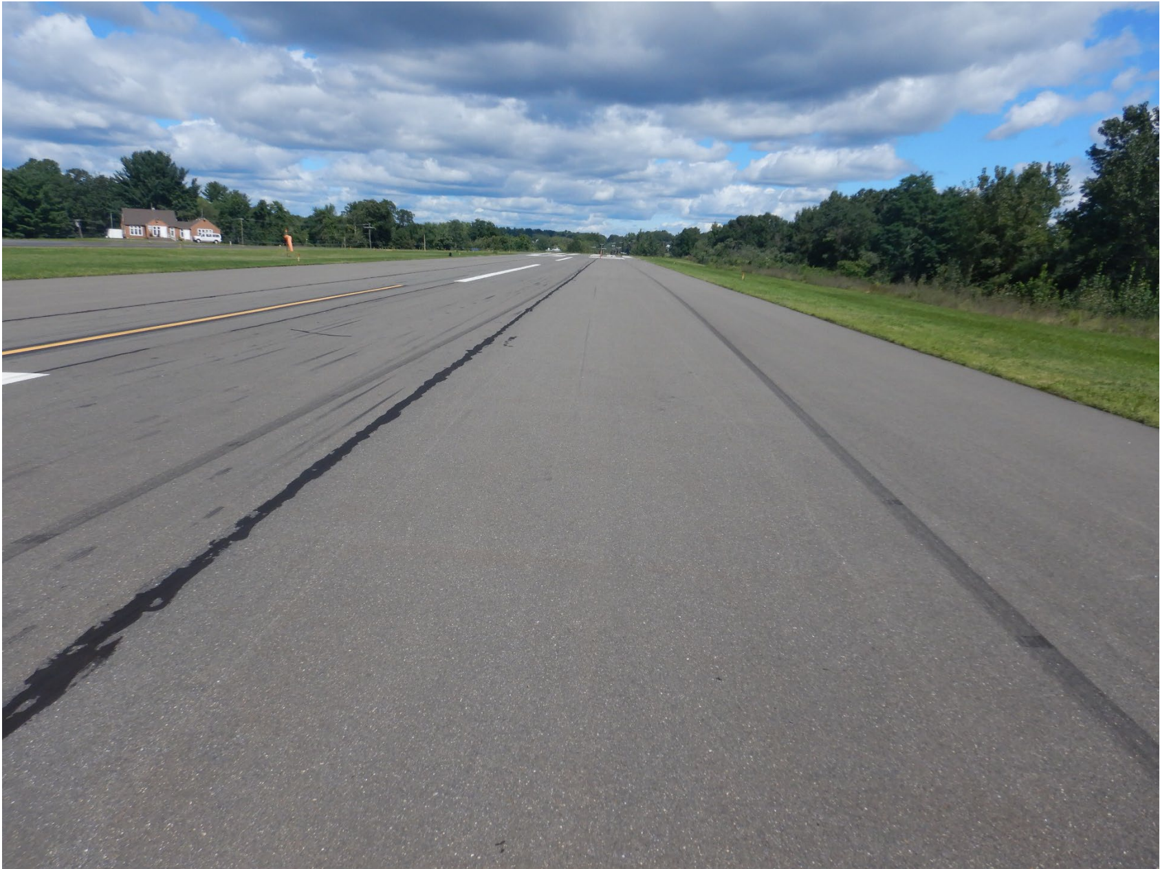
Photo 15 - Textron Aviation Digital Photograph. View Showing the Left and Right Main Landing Gear Tire Skid Marks. Note the Alternating Light and Dark Spaced 6 Ft 6 Inches Apart for Both.
