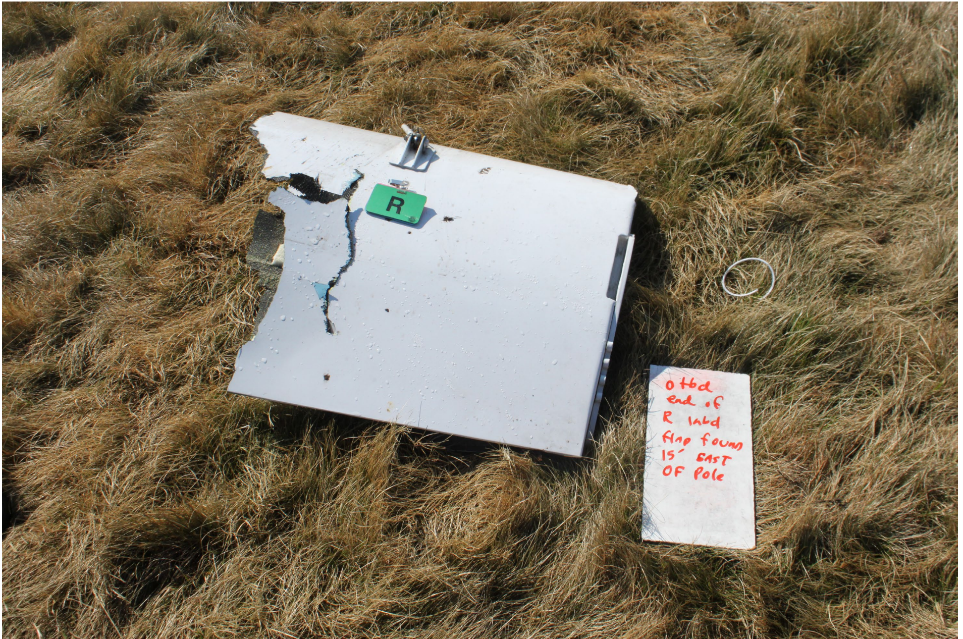
Photo 3 - NTSB Digital Photograph. Outboard End of Right Inboard Flap Found 15 Ft East of Impacted Pole.
