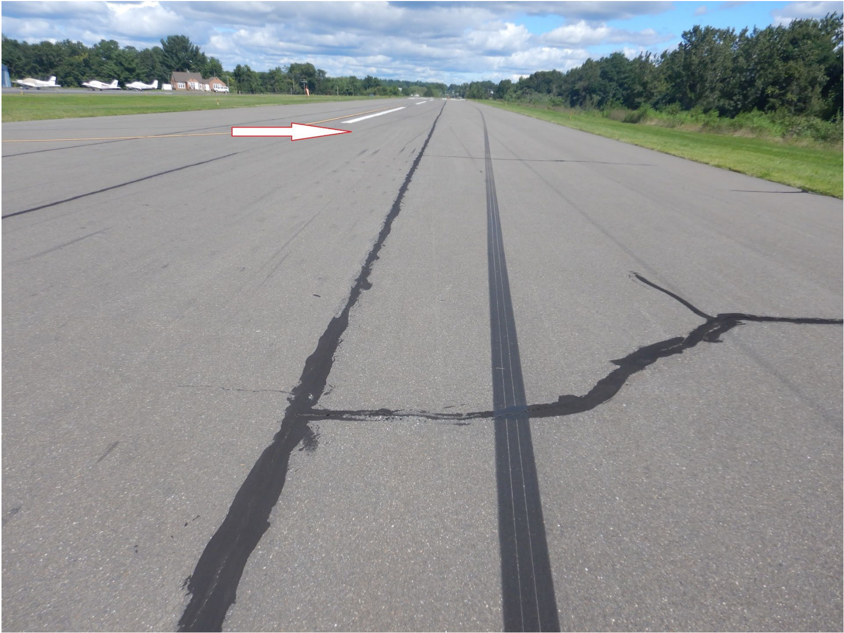
Photo 12 - Textron Aviation Digital Photograph. Arrow Points to Left Main Landing Gear Tire Mark. Note the Very Dark Mark From Right Main Landing Gear Tire and The Drainage Grooves in The Tread.
