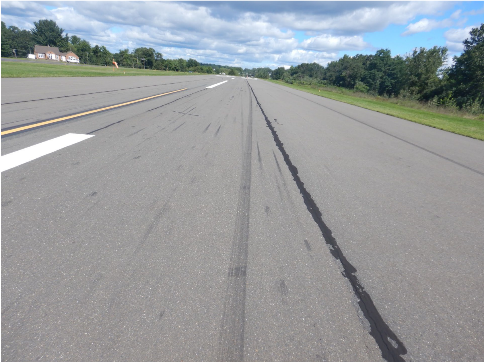
Photo 14 - Textron Aviation Digital Photograph. View of Left Main Landing Gear Tire Track. Note the Alternating Light and Dark Locations Spaced 6 Ft 6 Inches Apart.
