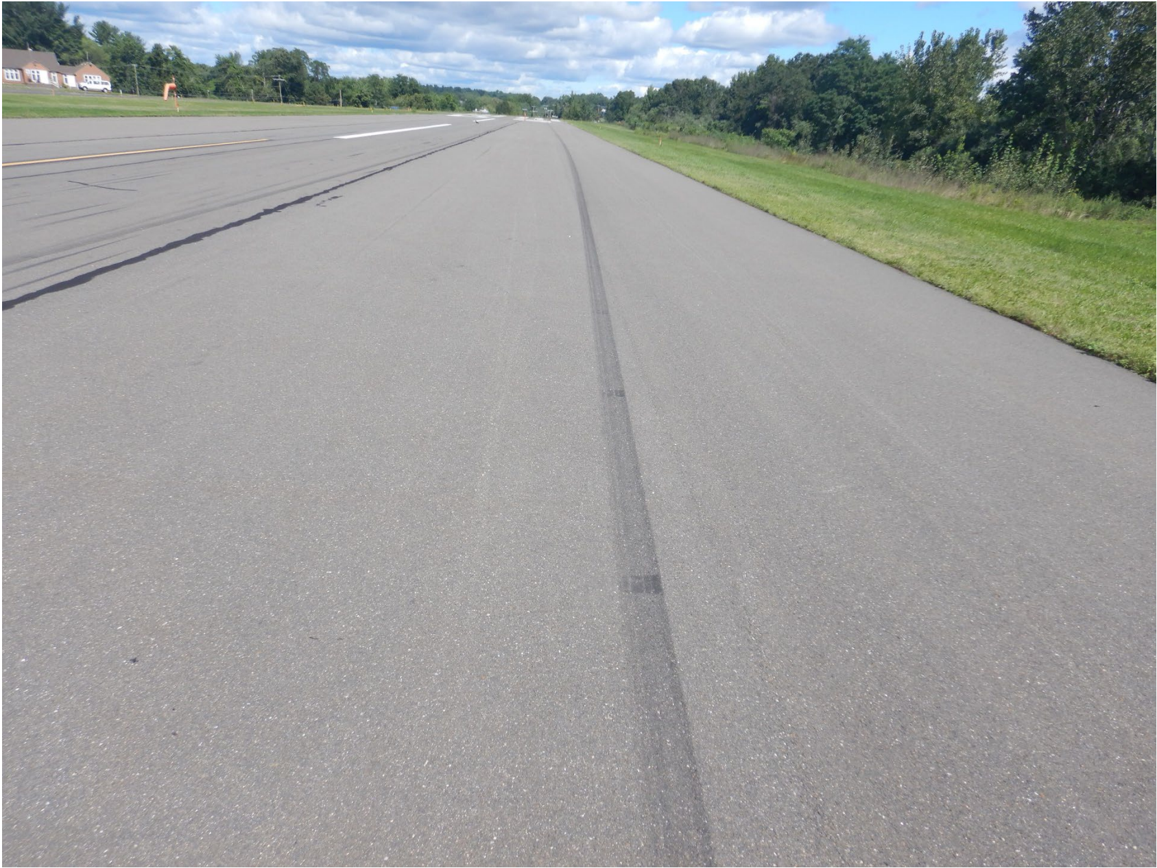
Photo 13 - Textron Aviation Digital Photograph. View of Right Main Landing Gear Tire Track. Note the Alternating Light and Dark Locations Spaced 6 Ft 6 Inches Apart.
