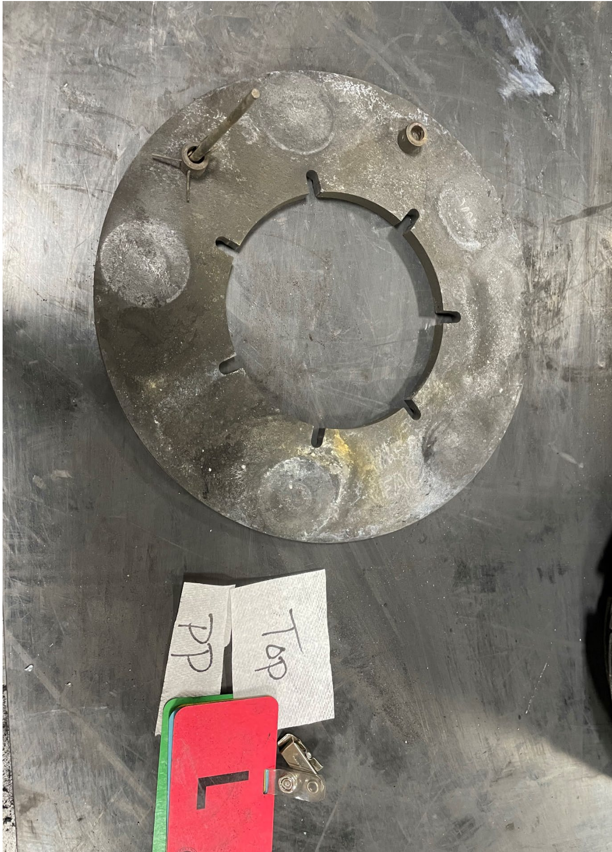
Figure 17. The left brake assembly pressure plate, top side.
