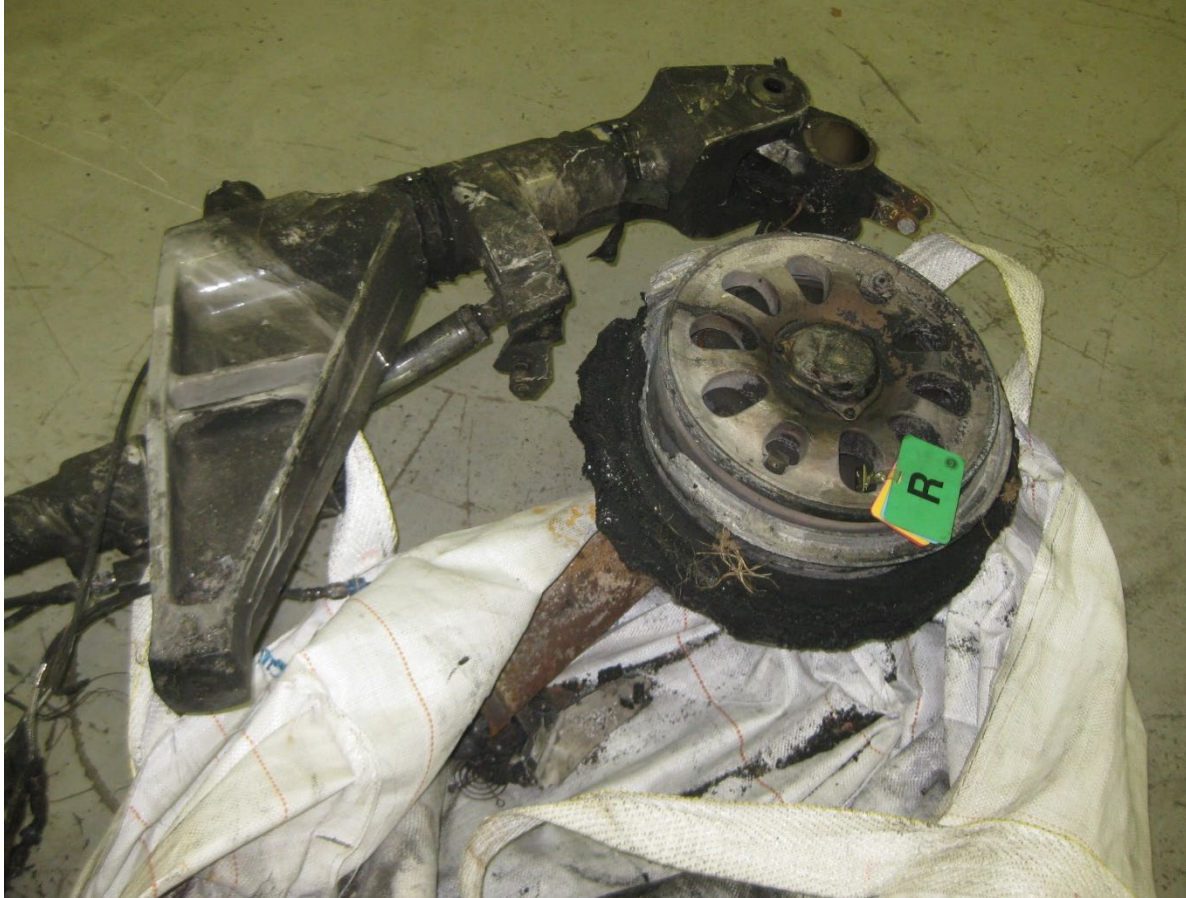
Figure 11. The right landing gear, tire remnants, and wheel assembly.
