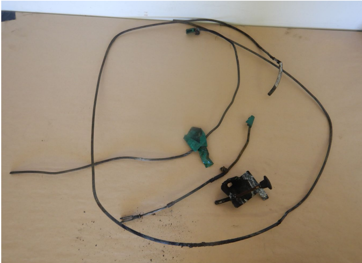
Figure 7. Portions of the parking brake cable (and parking brake knob), as found.
