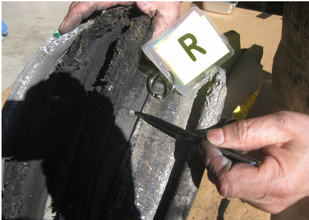
Figure 12. An opened fuse plug hole on the right wheel.
