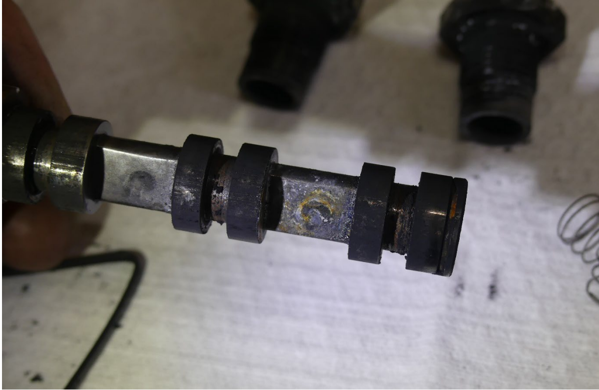
Figure 19. The parking brake valve cam, with witness marks on the flat spots.
