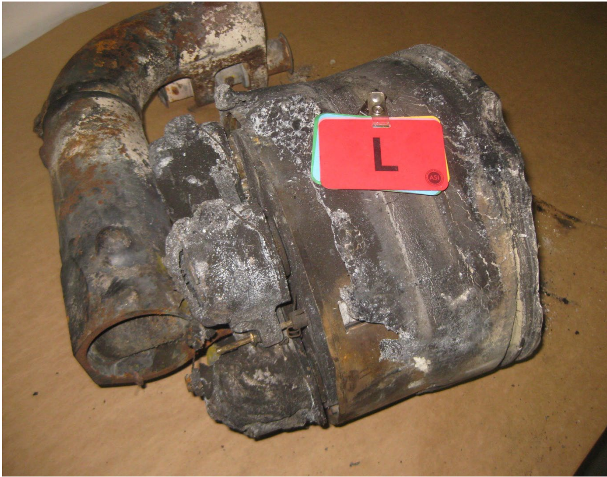
Figure 9. The left wheel and brake assembly.
