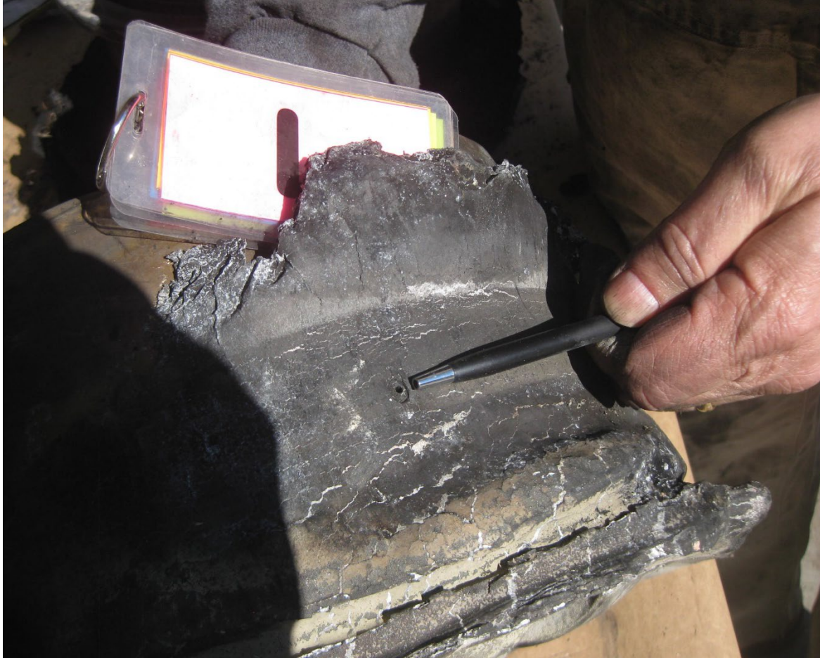
Figure 10. An opened fuse plug hole on the left wheel.
