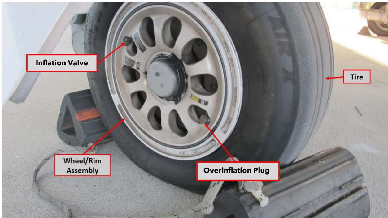
Figure 5. Main landing gear tire and wheel assembly, from an exemplar airplane.
