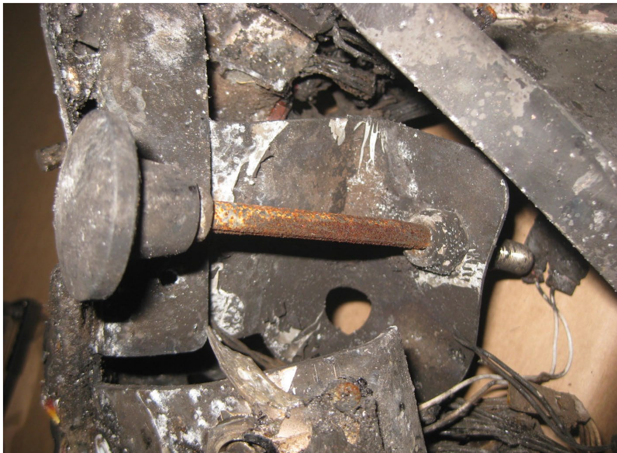
Figure 6. The flight deck parking brake knob, as identified in the airplane wreckage.
