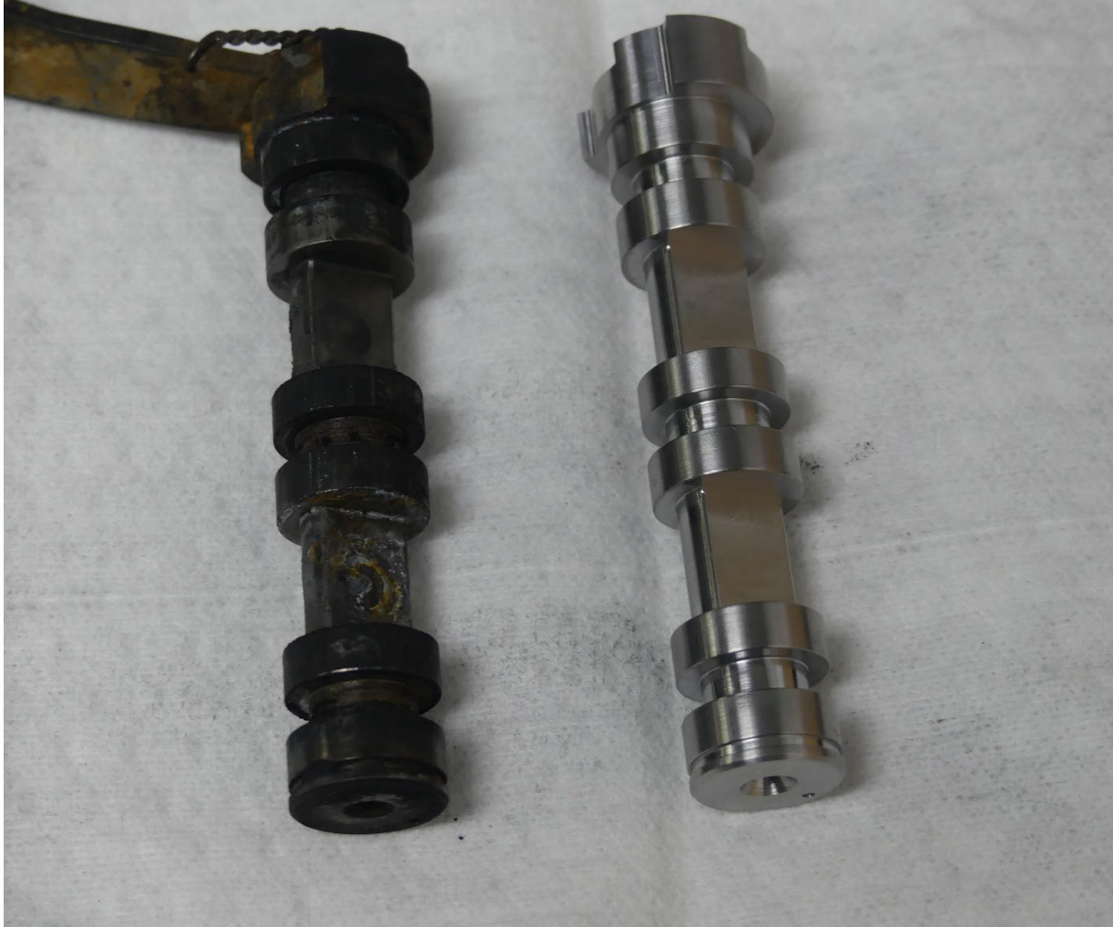
Figure 20. Side by side comparison of the accident parking brake valve's cam and lever (left) against a new cam (right).
