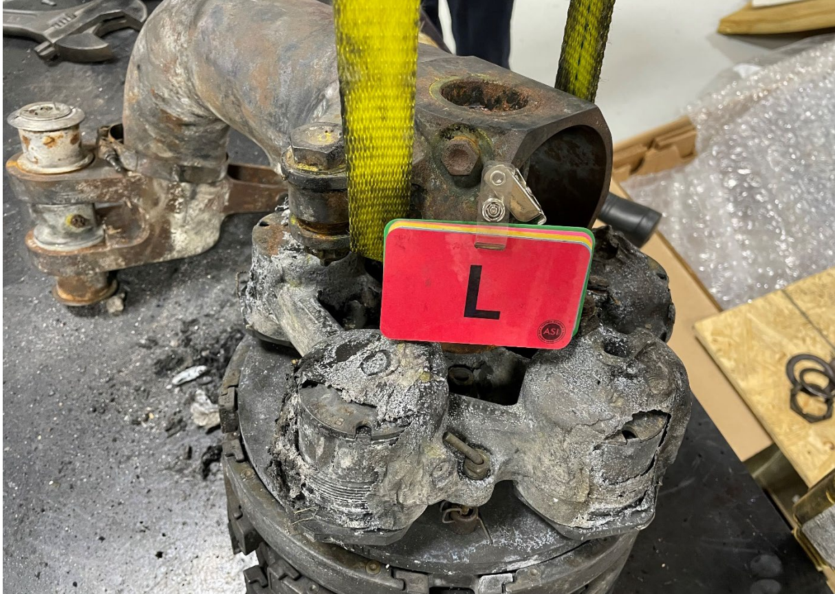
Figure 15. Left brake assembly and damage to the brake piston housings.
