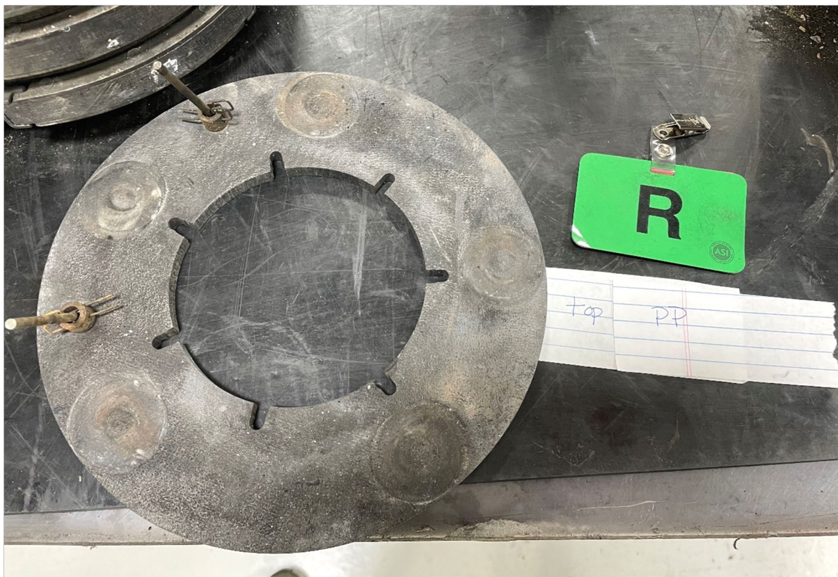
Figure 14. The right brake assembly pressure plate, top side, after disassembly.
