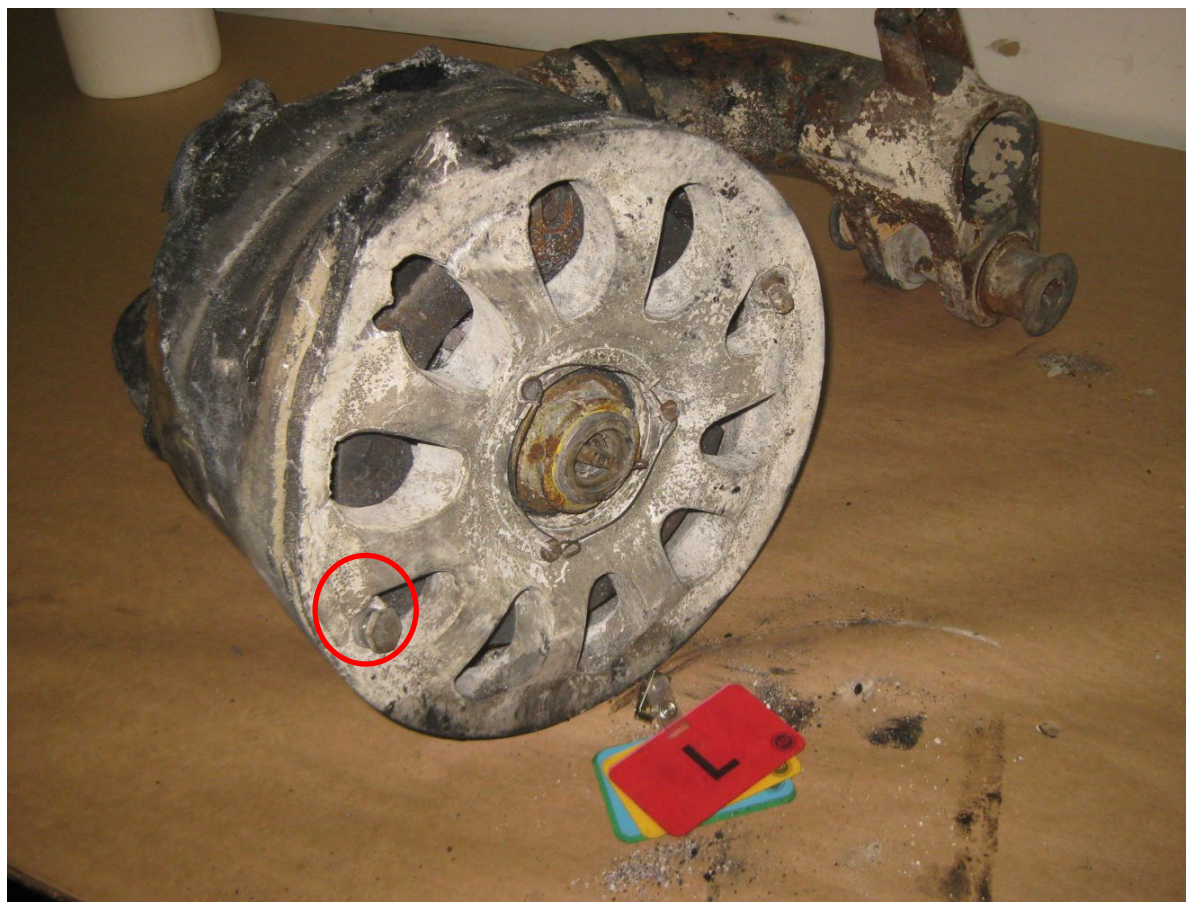
Figure 8. The left main landing gear wheel assembly and trailing link. The overinflation plug is circled in red.
