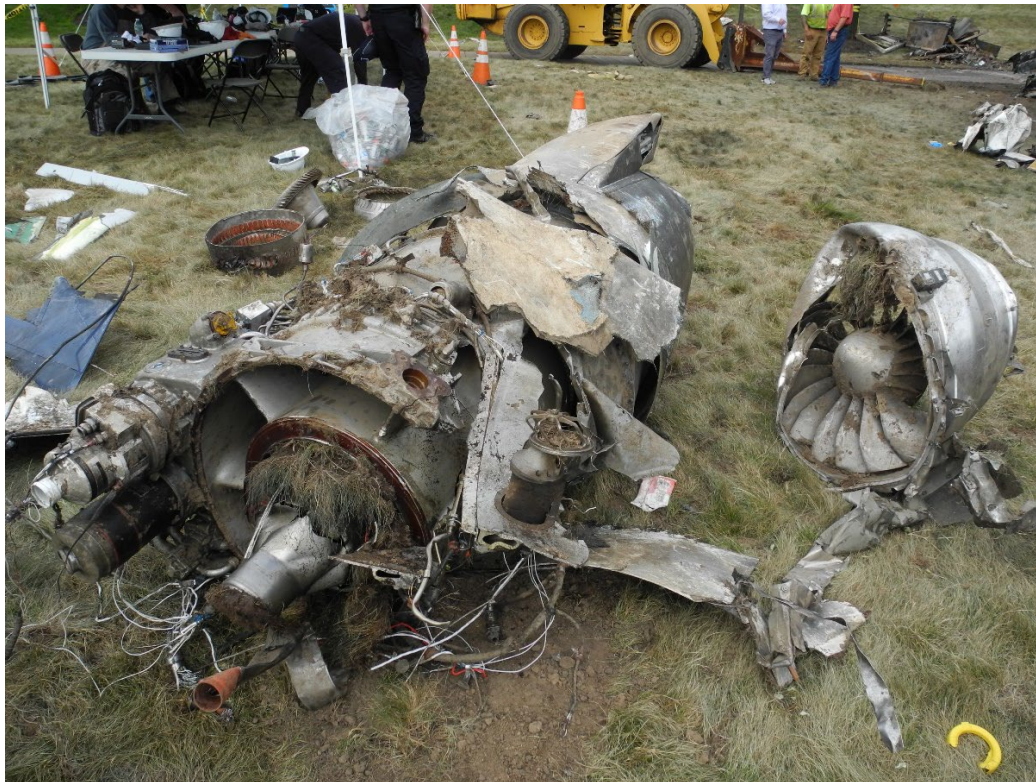
Photo 10 – RH cowling parts retrieved from field and placed with engine
