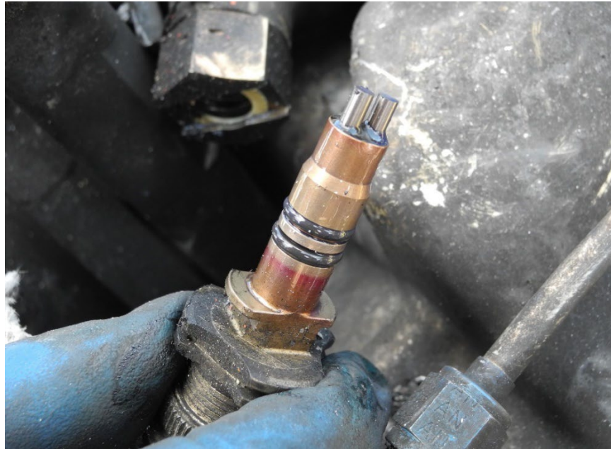
Photo 6 - LH Engine chip detector - Clean
