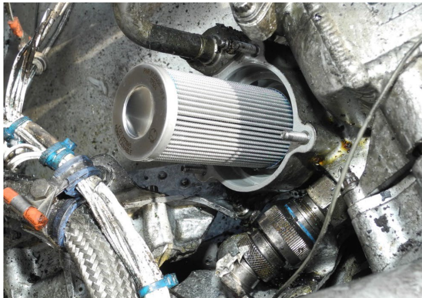
Photo 7 - LH Engine fuel filter - Clean
