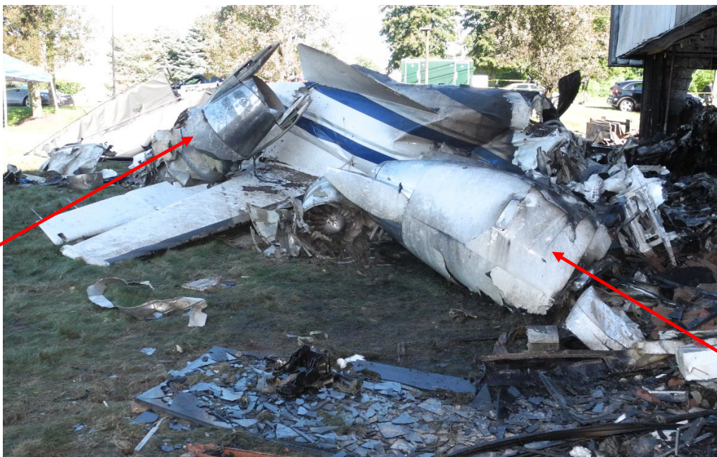
Photo 1 - RH & LH Engine - On-scene and In-Situ - View from side - Note inverted fuselage
