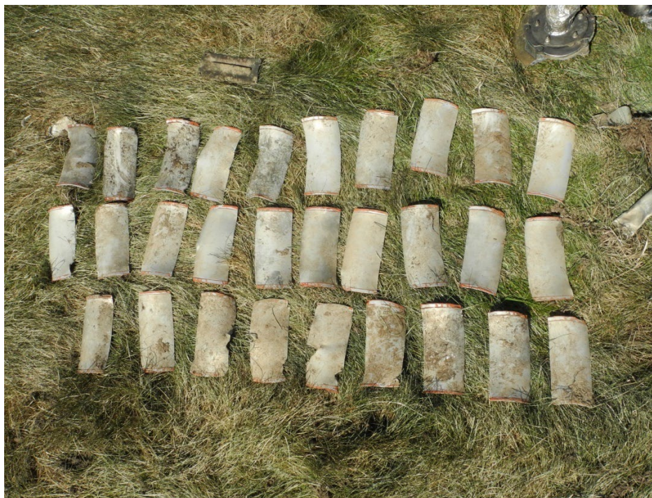
Photo 14 - RH engine fan exit guide vanes - Collected from debris field
