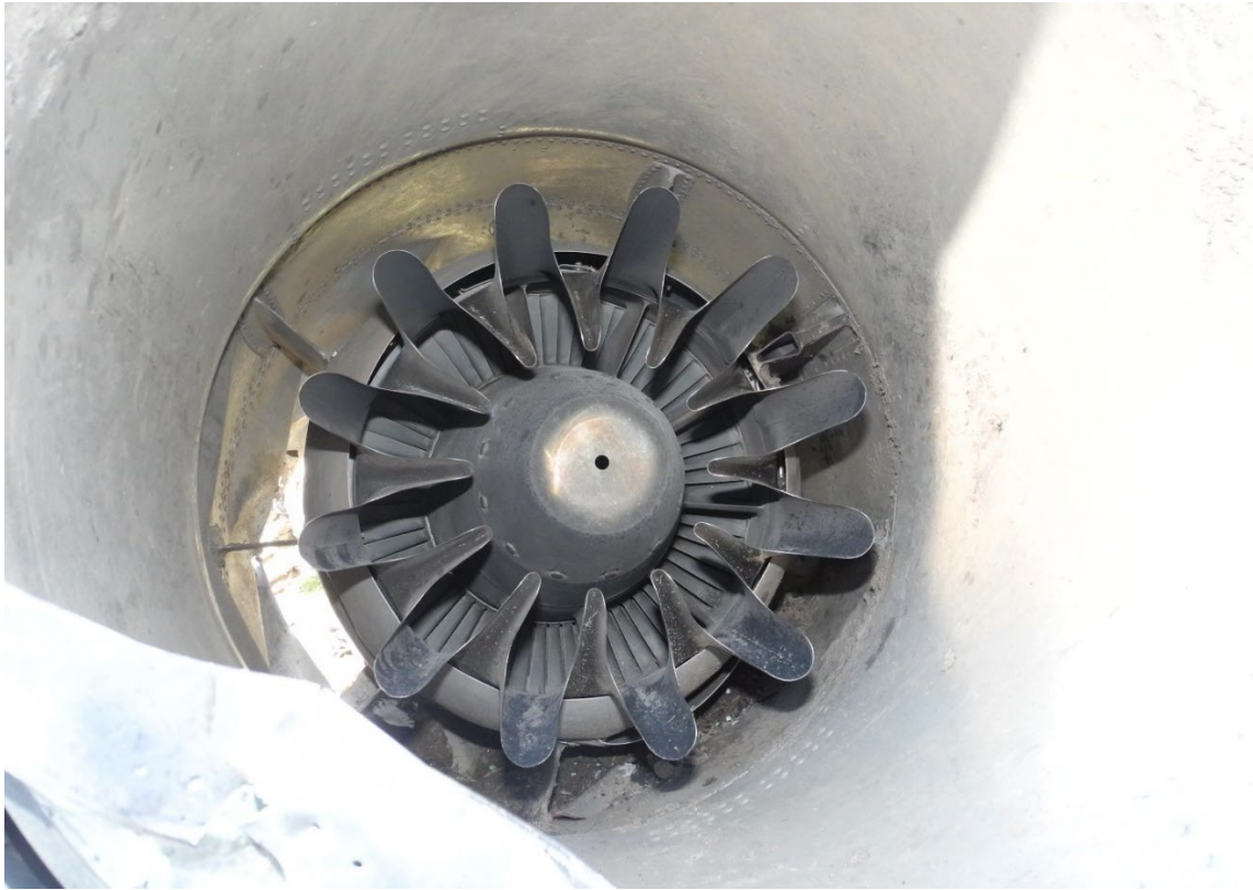
Photo 15 - RH engine last stage LPT blades and mixer
