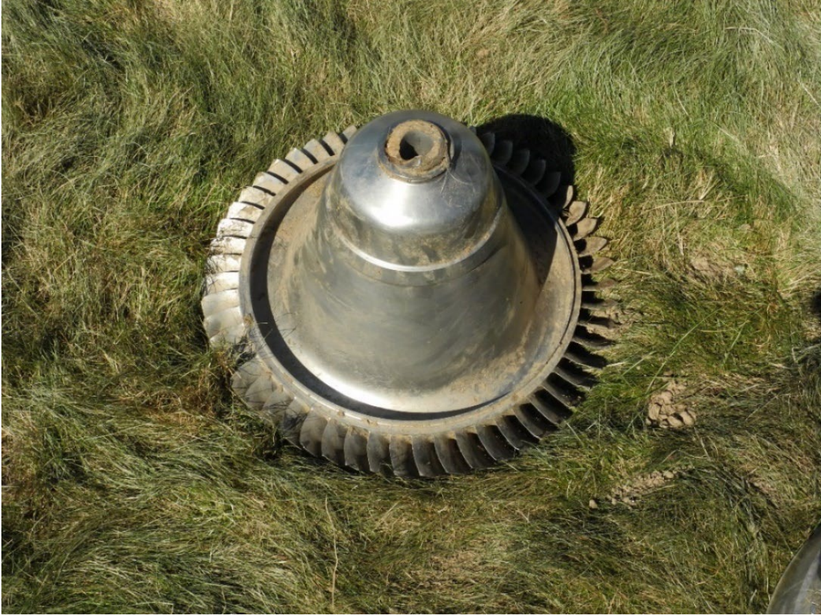
Photo 12 - RH Engine LPC rotor and hub
