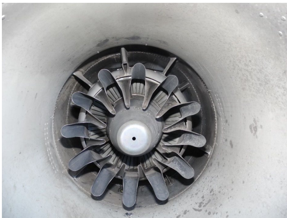
Photo 5 - LH Engine - Low pressure turbine - No damage
