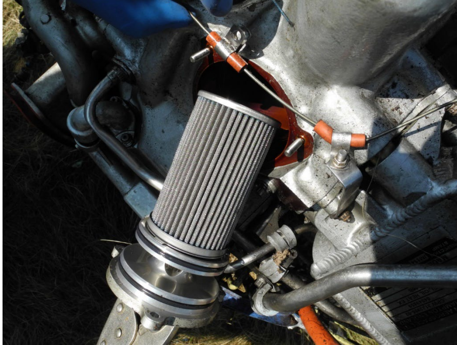
Photo 18 - RH Engine oil filter - Clean
