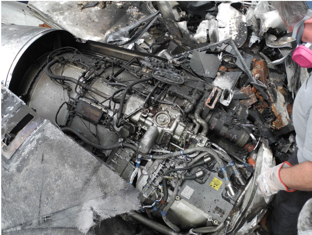
Photo 3 - LH Engine - Sooty deposits on external components
