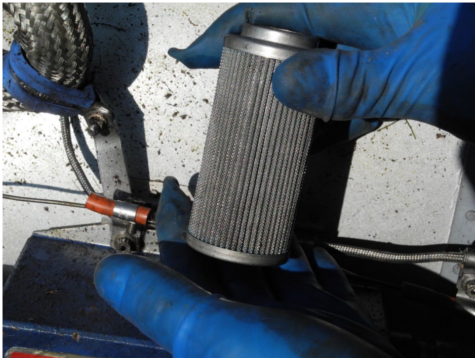
Photo 17 - RH engine fuel filter - Clean
