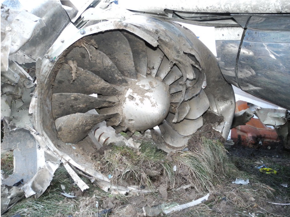
Photo 11 - RH engine fan disk and fan case - Separated from engine
