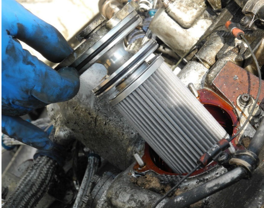
Photo 8 - LH Engine oil filter - Clean
