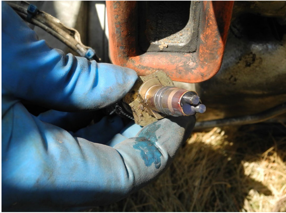
Photo 16 - RH engine chip detector - Clean
