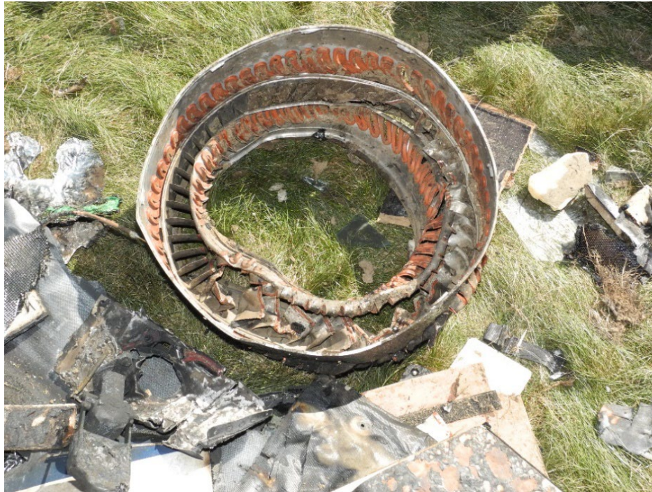
Photo 13 - RH engine inner stator core
