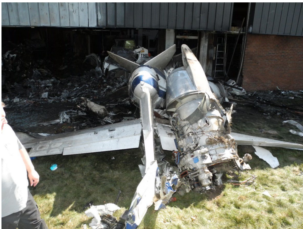
Photo 2 - RH Engine In-Situ - View from aft. LH engine in background. Note inverted empennage
