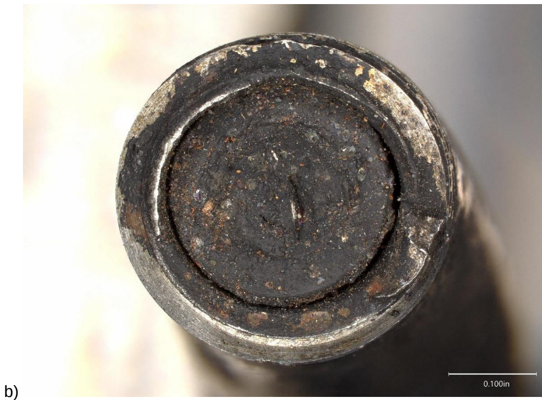
Figure 3: Images of the fracture through the sleeve and the inner cable assembly, as received; a) side connected to the pull rod and knob and b) side connected to the cable.
