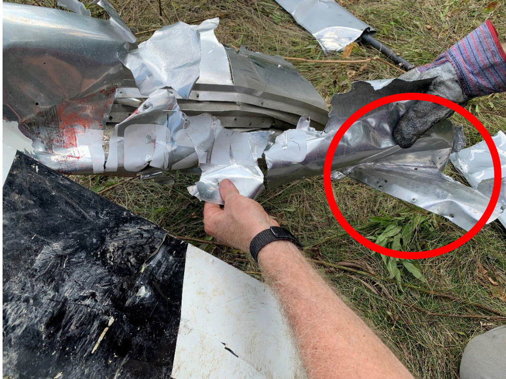
Figure 8 Impact Marks at Forward End of Tail Boom Section
