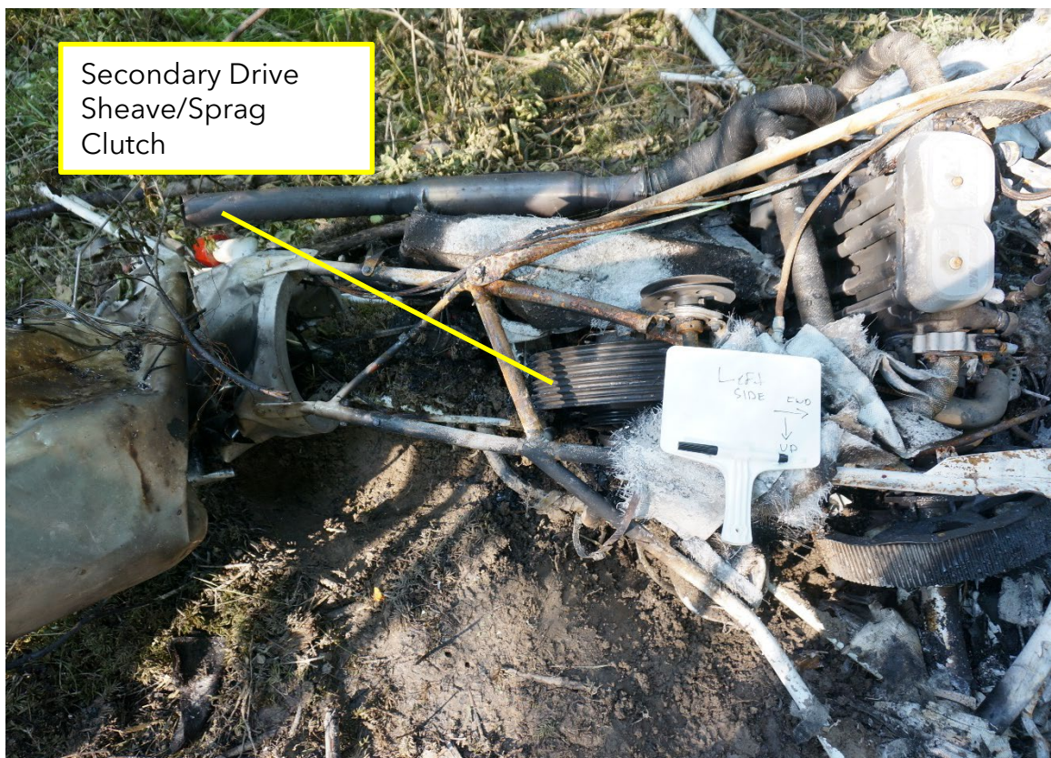
Figure 35 - Secondary Drive Sheave
