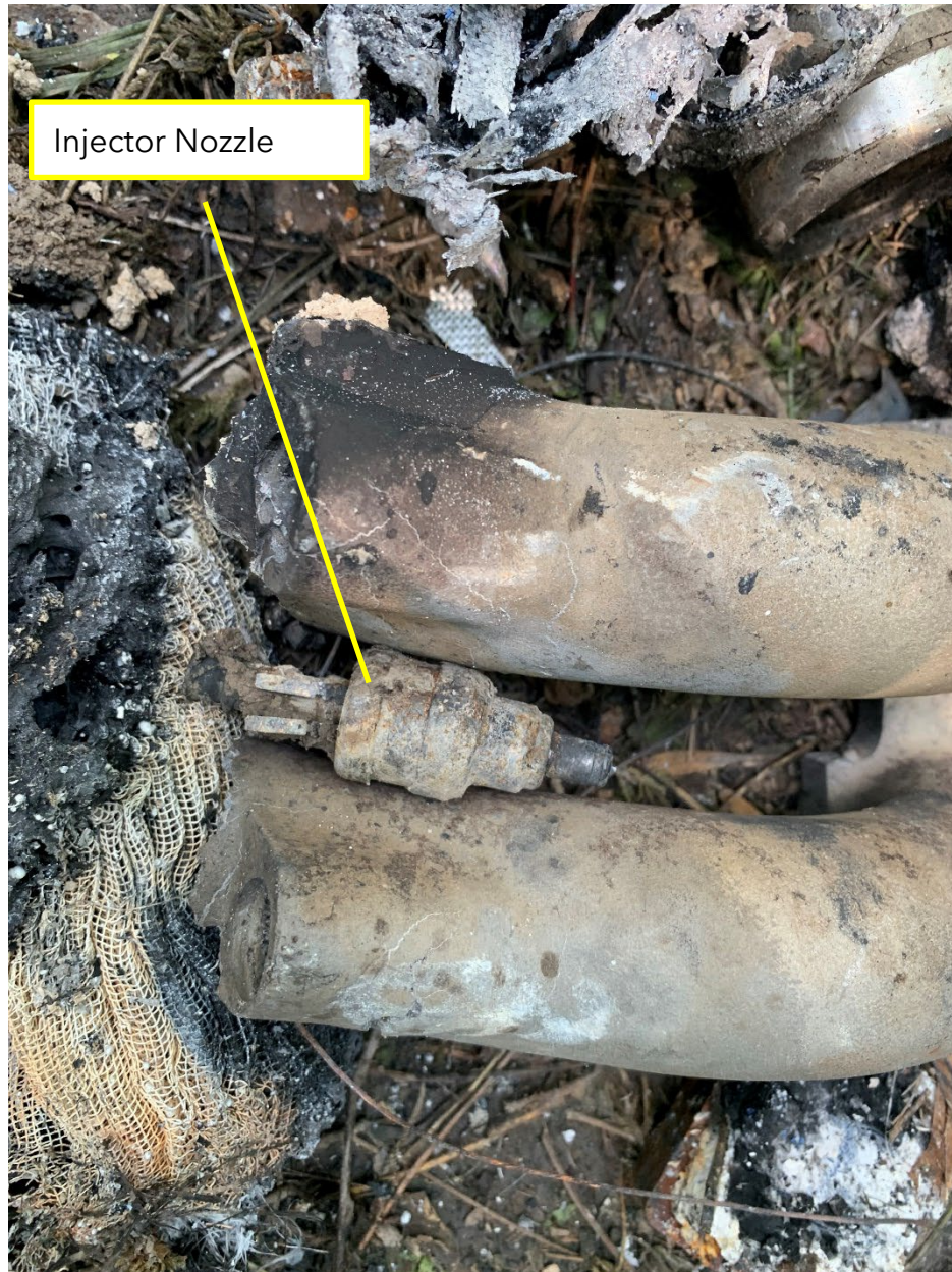
Figure 32 - Intake Manifold, Unknown Side
