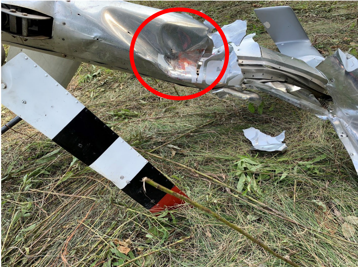
Figure 7 - Impact Marks and Paint Transfer - Tail Rotor Blade
