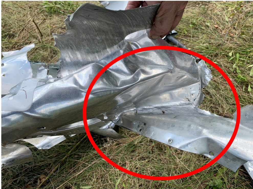
Figure 9 - Impact Marks at Forward End of Tail Boom Section (enlarged)
