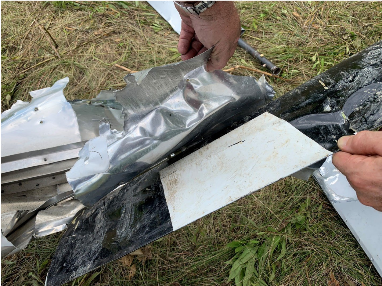
Figure 10 - Main Rotor Blade Shown at Impact Marks
