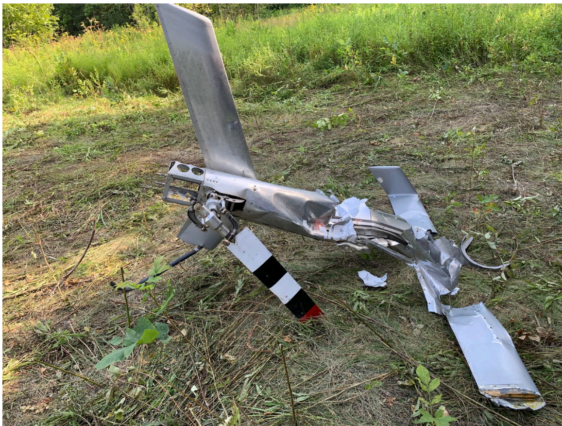
Photograph 4 - View of the Separated Tail Boom
