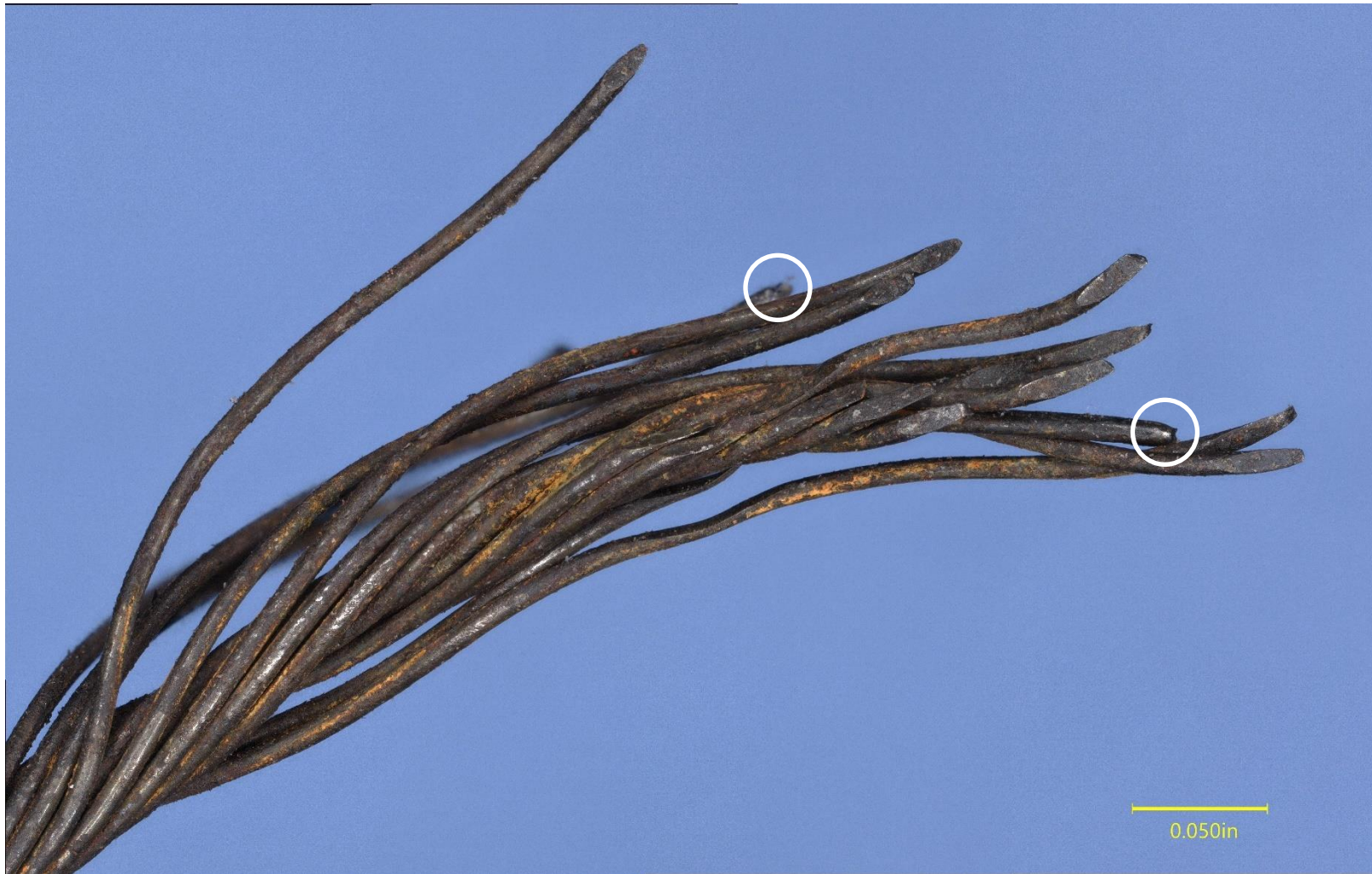
Figure 3: Strand 1 separated end. Two wires exhibited features consistent with overstress (white circles). The remainder were beveled, consistent with wear.
