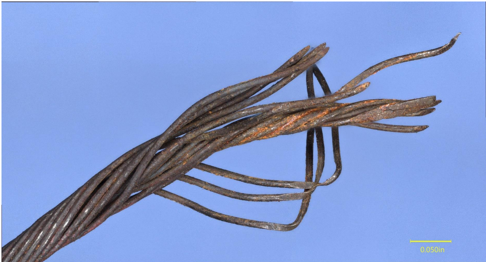
Figure 4: Strand 2 separated end. All wires were beveled, consistent with wear.
