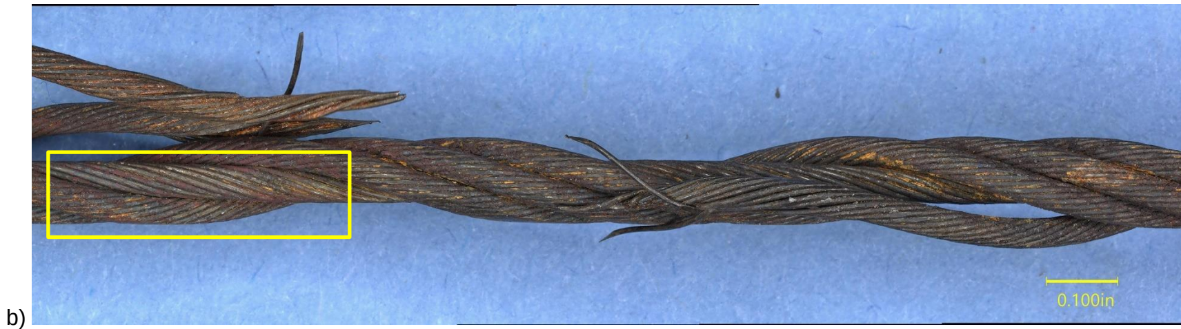
Figure 2: a) and b) higher magnification images of the cable at the point of strand separation. A yellow box in part b) highlights a region exhibiting wear of outward-facing wires on an intact strand.
