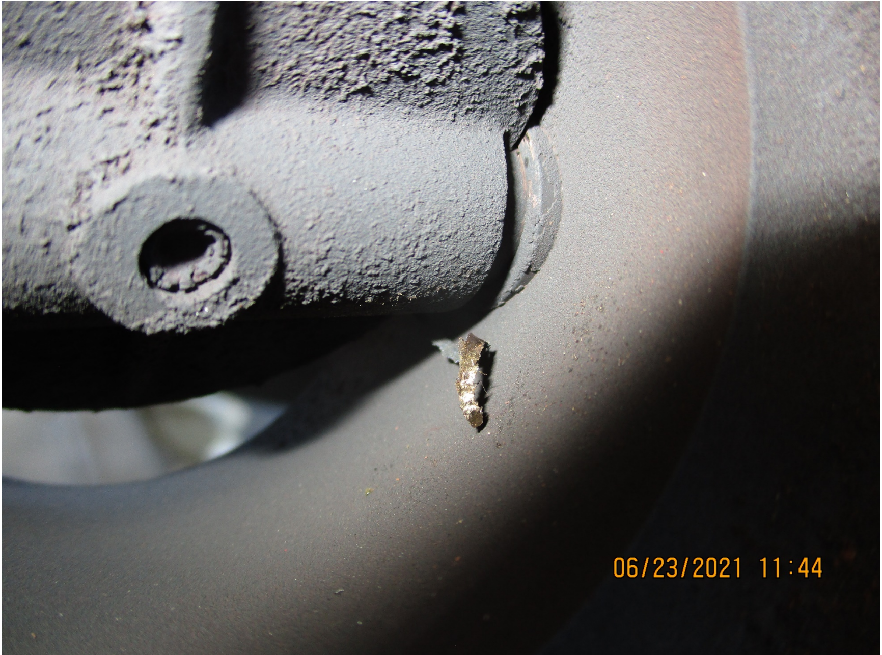
Photo 5 – close up of wire stuck in waste gate
