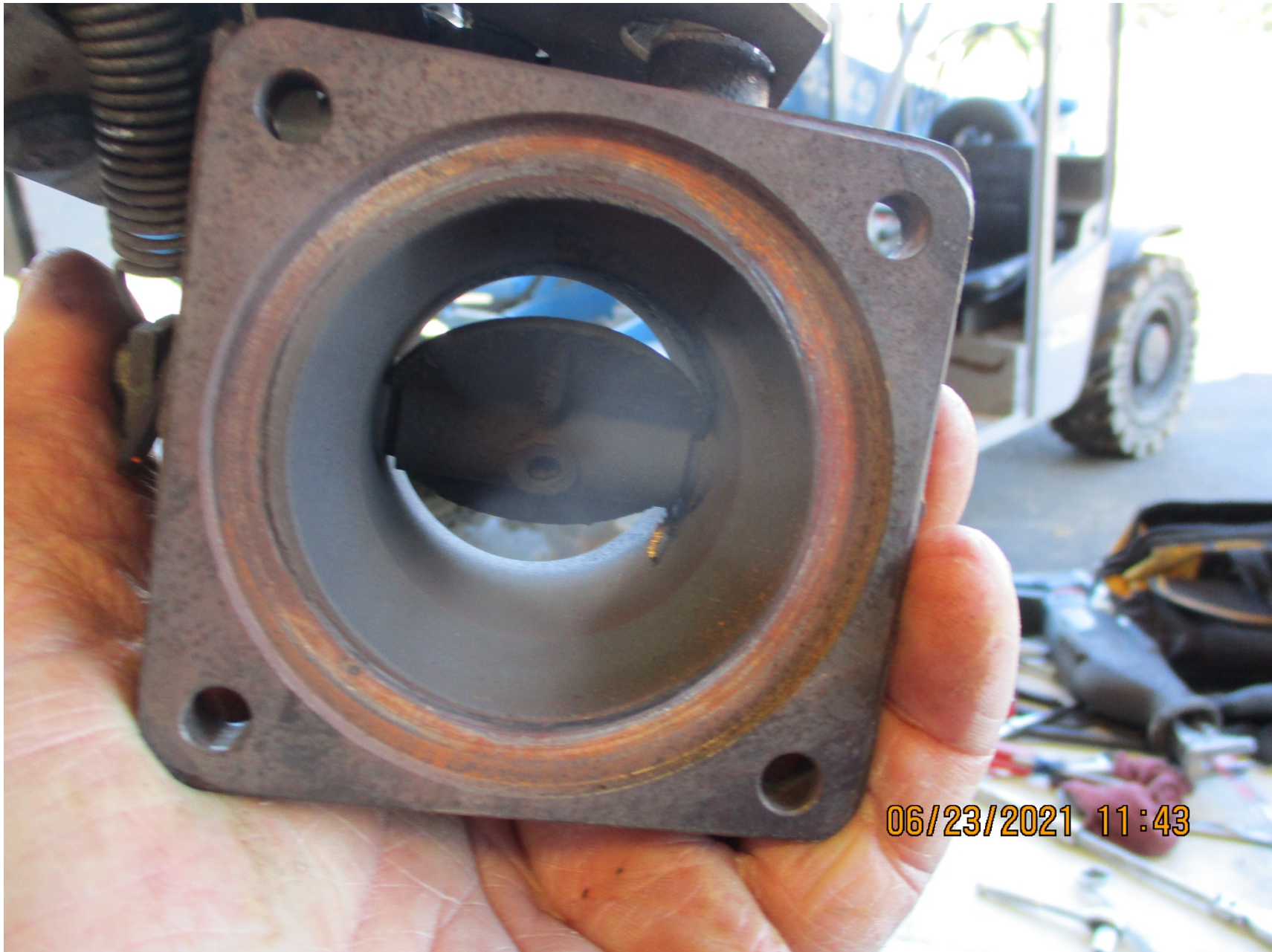
Photo 4 – wire stuck in waste gate
