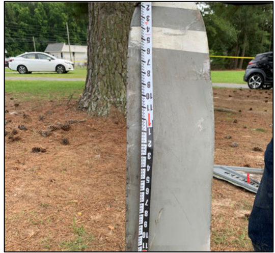
Figure 16: View of a propeller blade displaying impact marks and measurements of a chain fence impacted by airplane
