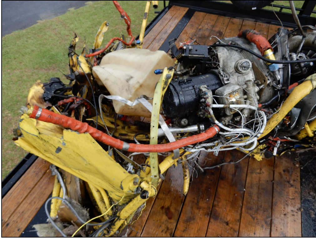
Figure 10: View of the engine once removed from terrain
