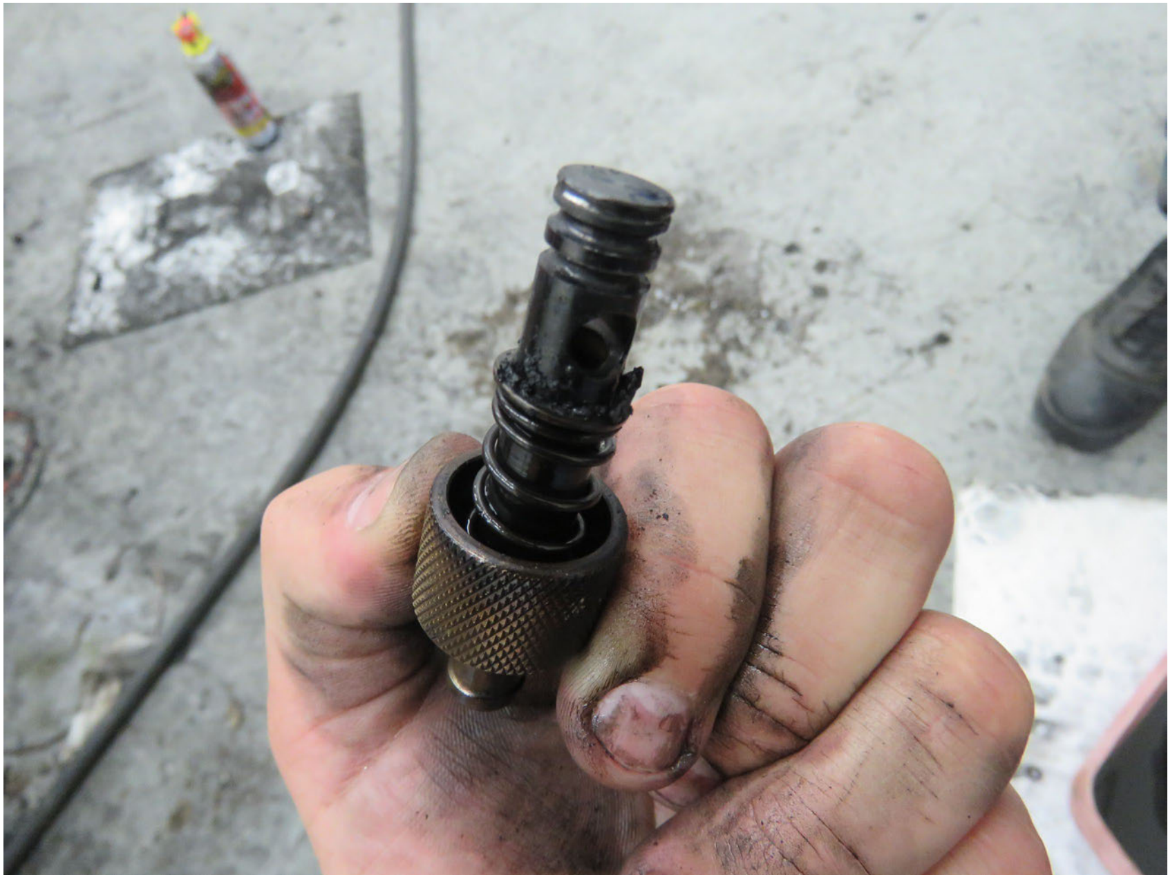
Photo 16 – Oil Quick Drain Displaying Gold Coloration and Thermal Damage – Courtesy of Lycoming Engines
