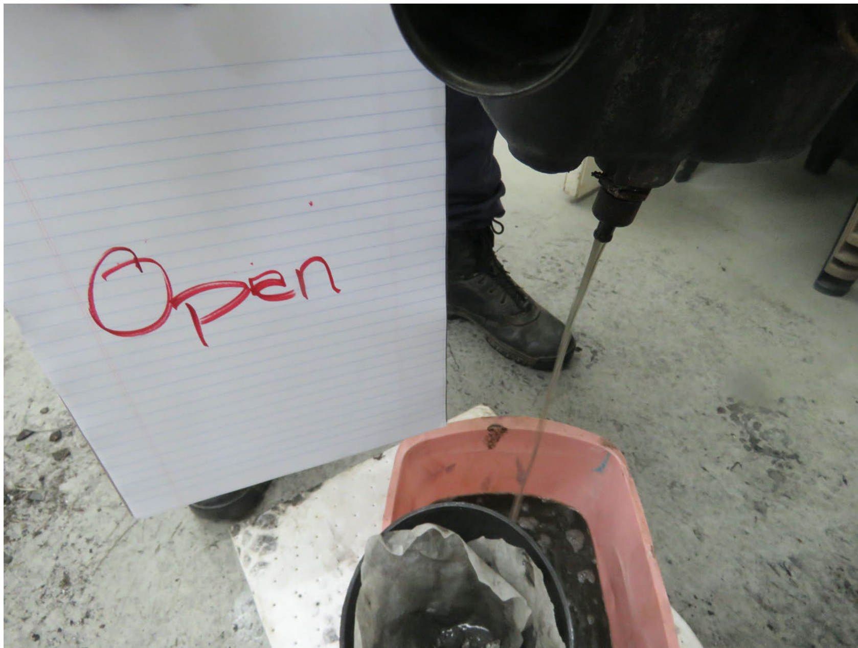
Photo 15 – Oil Quick Drain in Open Position – Courtesy of Lycoming Engines
