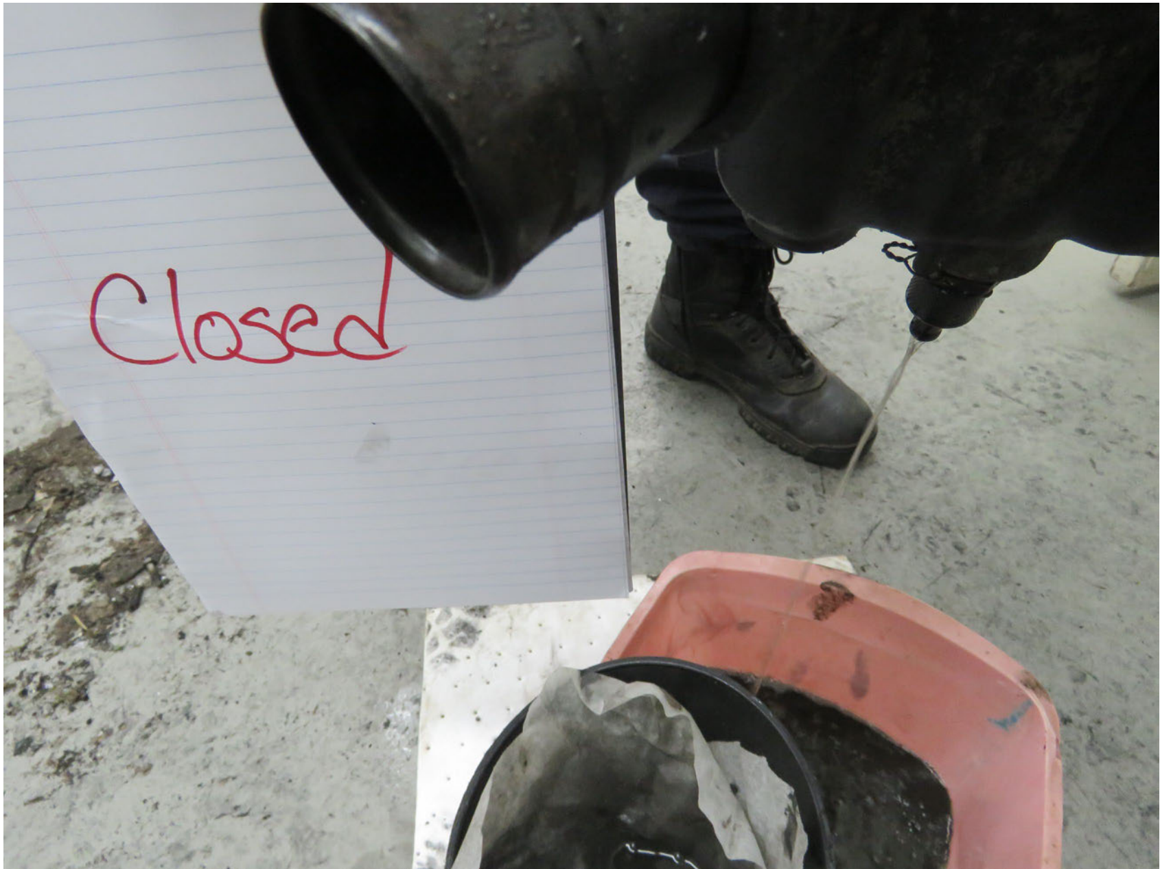
Photo 14 – Oil Quick Drain Leaking in Closed Position – Courtesy of Lycoming Engines
